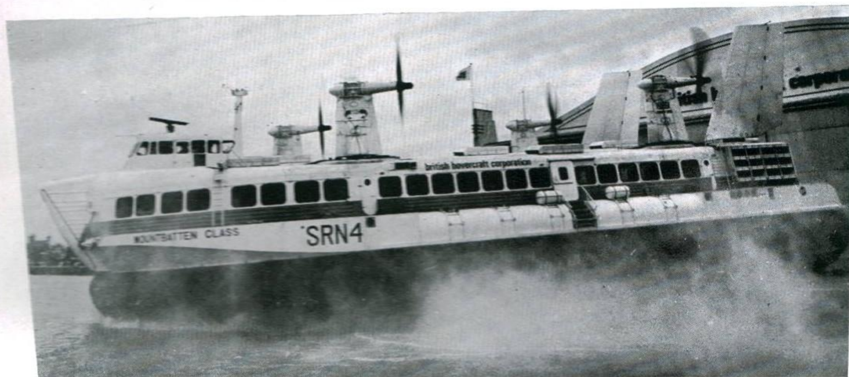
The first 165-ton "Mountbatten" (SR.N4) Class hovercraft, launched from BHC's East Cowes slipway, Isle of Wight in February
