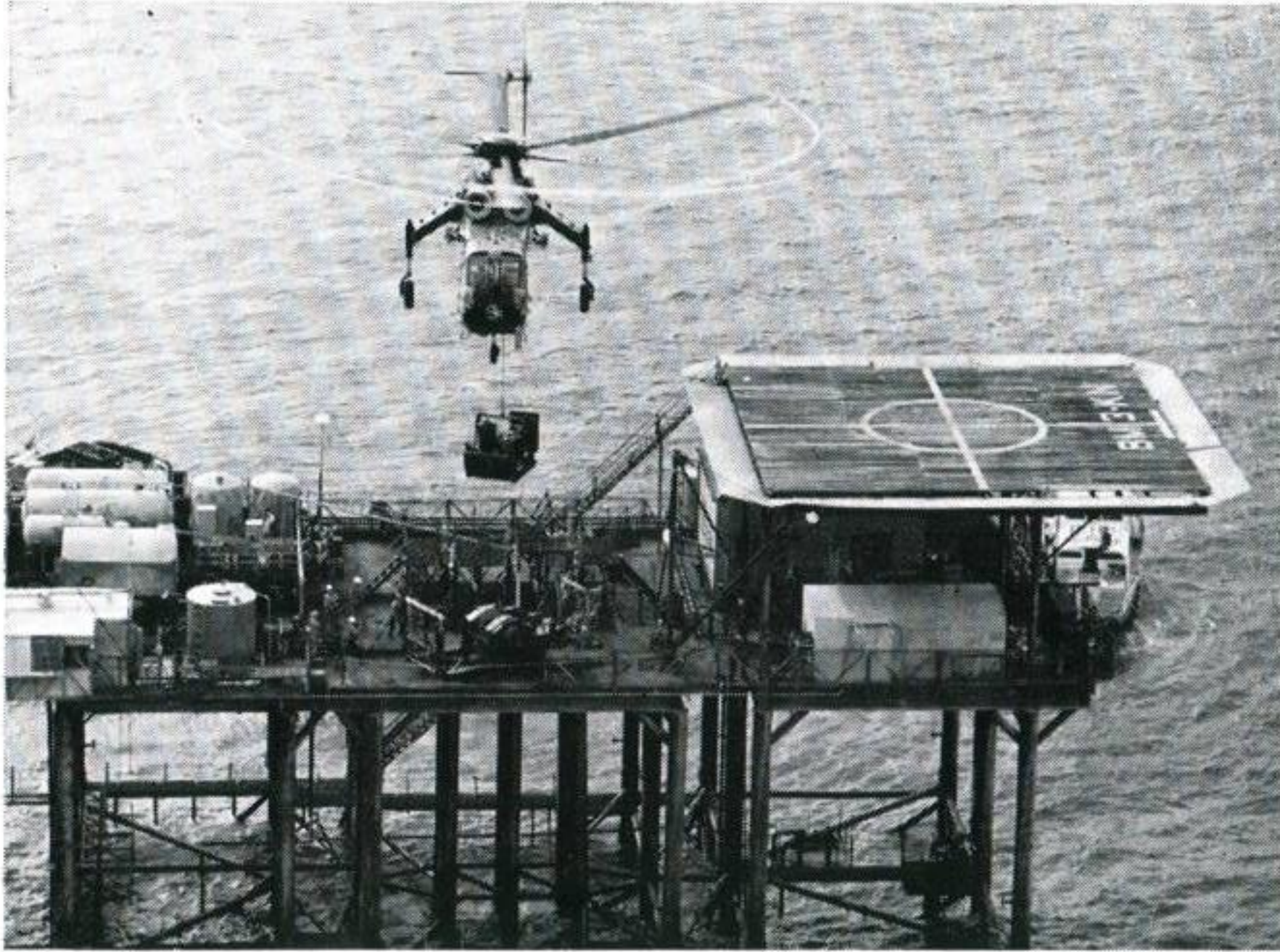
Cover Photo: Sikorsky S-64E Skycrane lowers drawworks engine assembly to offshore platform. An average of only 1.7 minutes required for the Skycrane to precision-place each piece of equipment. Loads were flown to the rig at a speed of 100 knots. The average round trip from marshalling yard to rig was 13.6 minutes.
