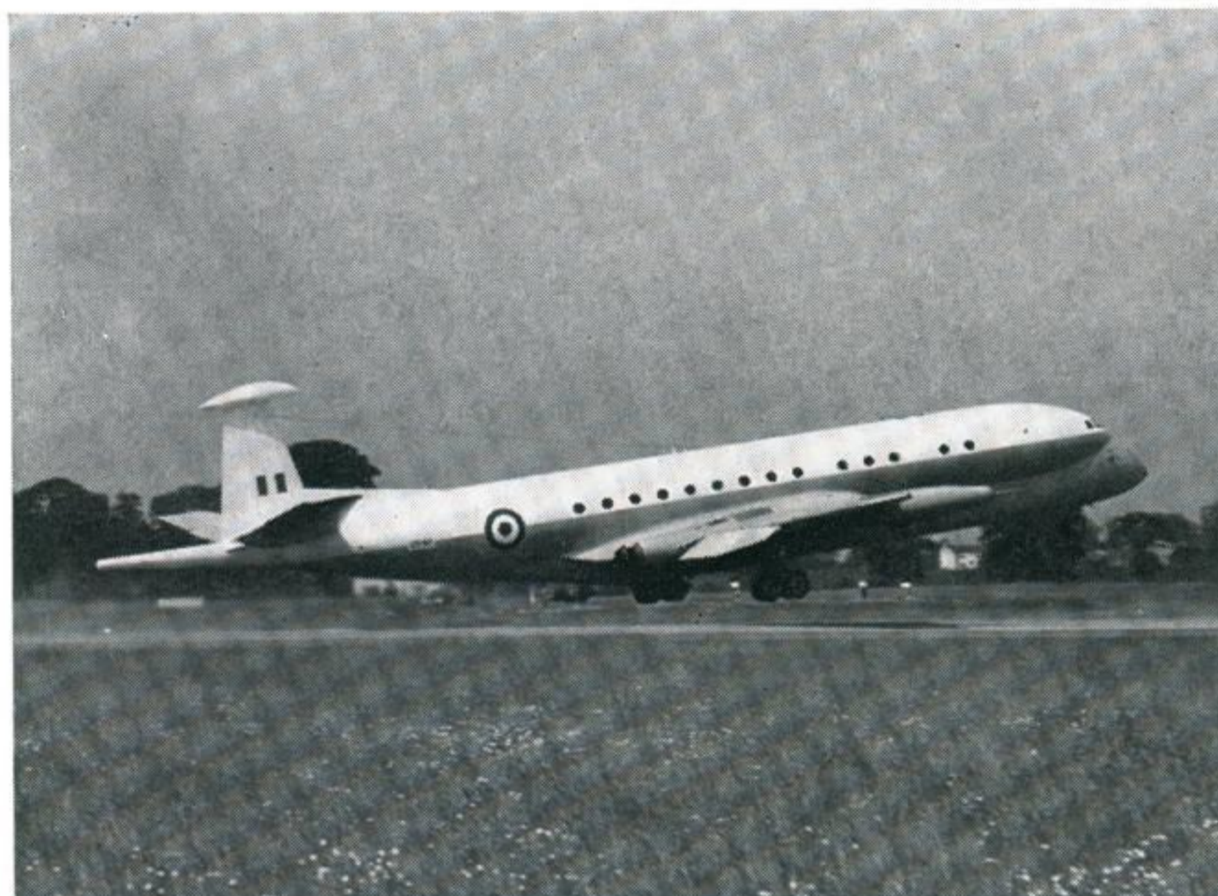
Cover Photo: A Hawker Siddeley Nimrod on a test flight from the Company's Woodford airfield. Designed to go into service with the RAF Coastal Command in the late 1960's as a maritime reconnaissance aircraft, the Nimrod will fly at high subsonic speed and high-altitude to the search area, low speed low-level patrol and a fast return to base. The aircraft is powered by four Rolls-Royce Spey turbofan engines.
