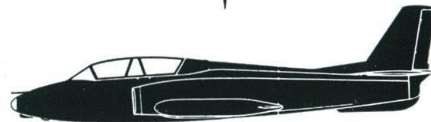
Span 34-38 feet according to the fitting of tip-tanks
