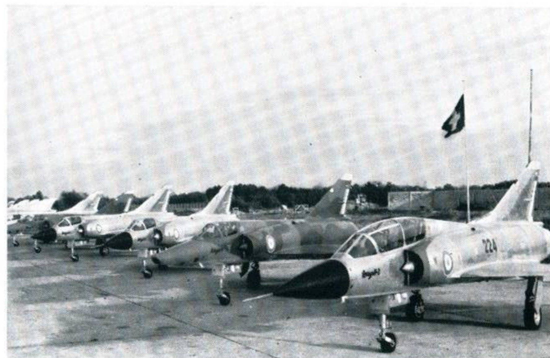
Finish according to function is epitomised by this line-up of French Air Force Mirage IIIs where the reconnaissance versions are camouflaged. The sub-types are, from front to rear: IIIB (two-seater), IIIR, IIIC, IIIC, IIIR, IIIC.
