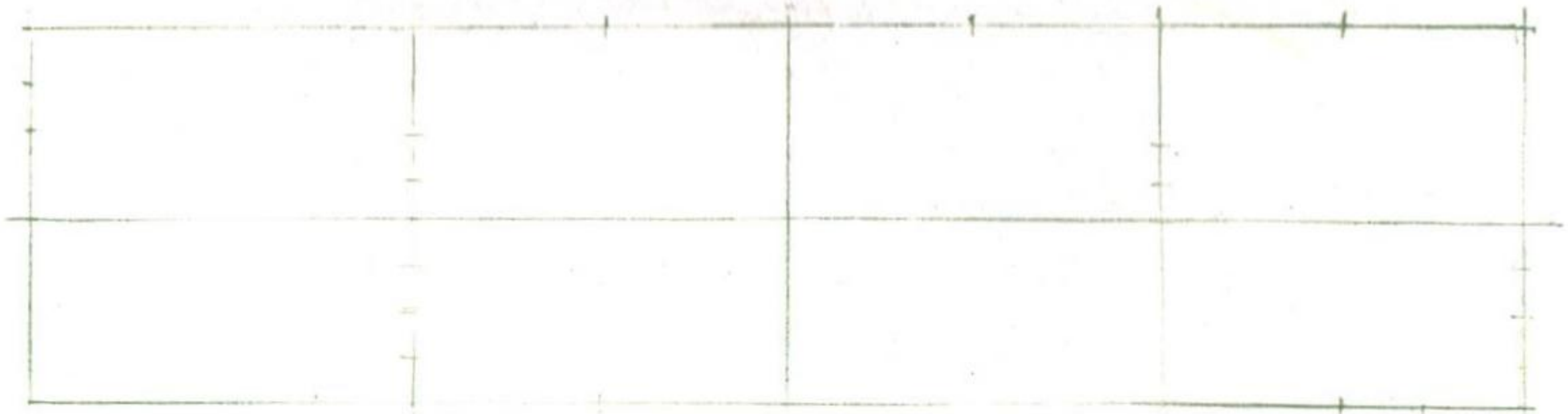
Stage 1 An oblong four times longer than high, bisected horizontally and sub-marked as indicated.
