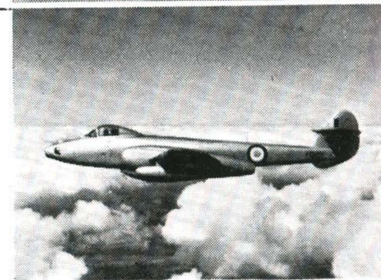
METEOR PR Mk. 10 (G.B.) Photo-Recce Ventral fuselage and/or under-wing tanks may be carried. Span: 43 ft.
