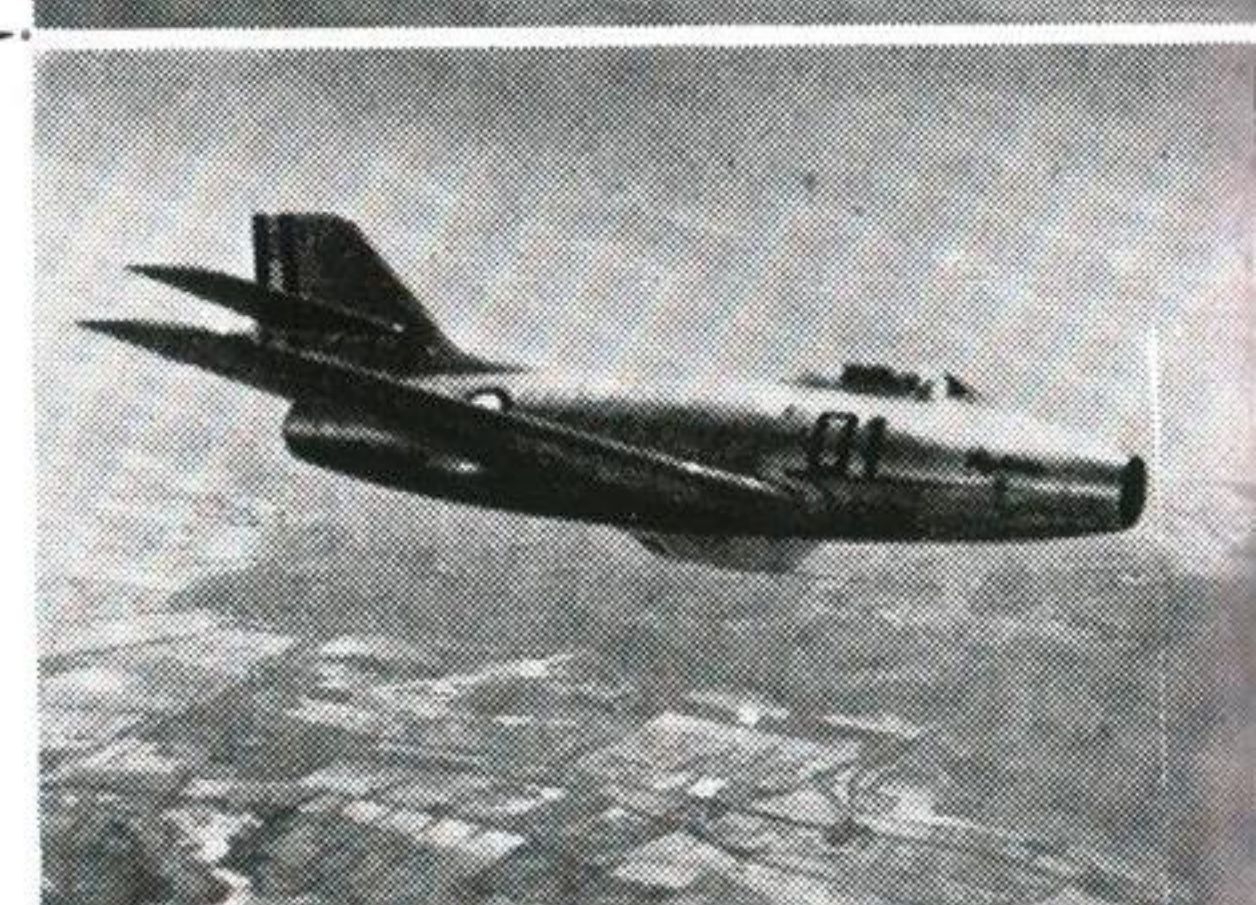
MYSTÈRE IIC (FRANCE) Fighter Wing-tip tanks may be carried. Span: 38 ft.
