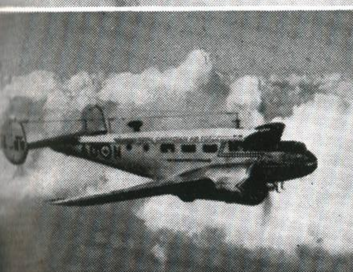
EXPEDITOR (U.S.A.) Light Transport U.S.A.F.: C-45. U.S. Navy: JRB and SNB. South America: T-11, Kansan, similar but having blunt, transparent nose and dorsal cupola. Span: 48 ft.
