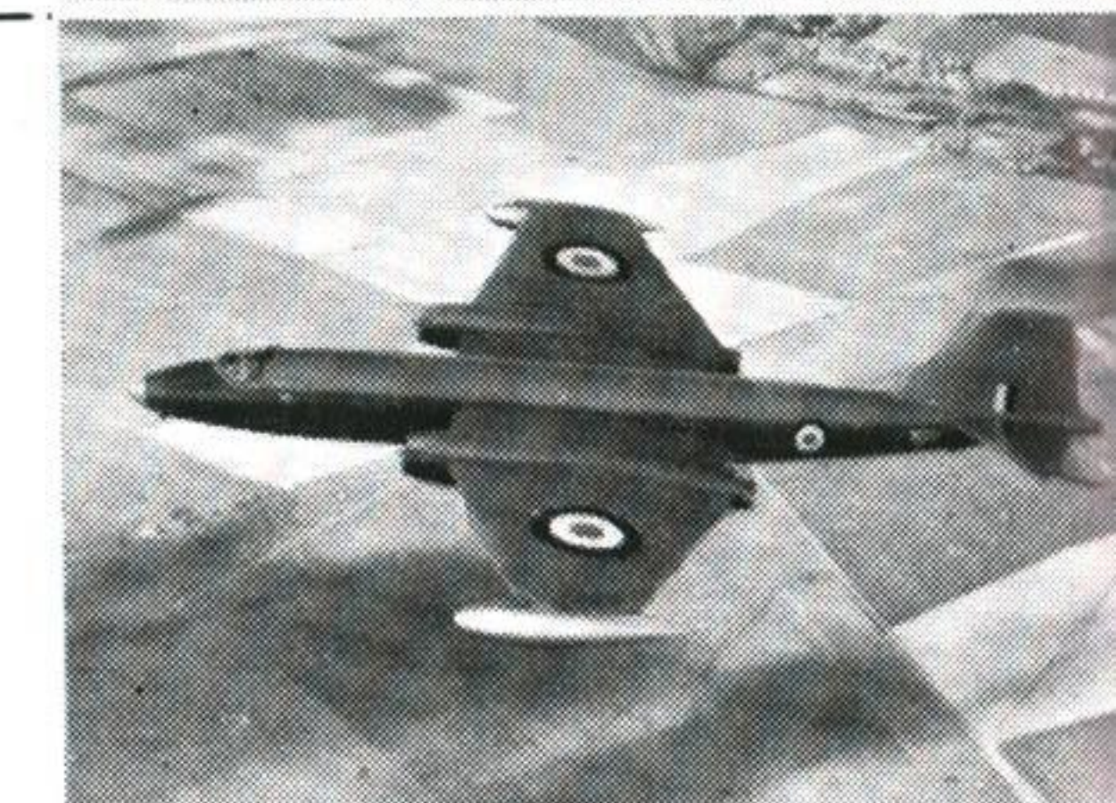
CANBERRA B Mk. 2 (G.B.) Light Bomber T.4, similar but with unglazed nose. B.6, PR. 3 and 7, similar but have longer fuselages. Wing-tip tanks may be carried. Span: 64 ft.
