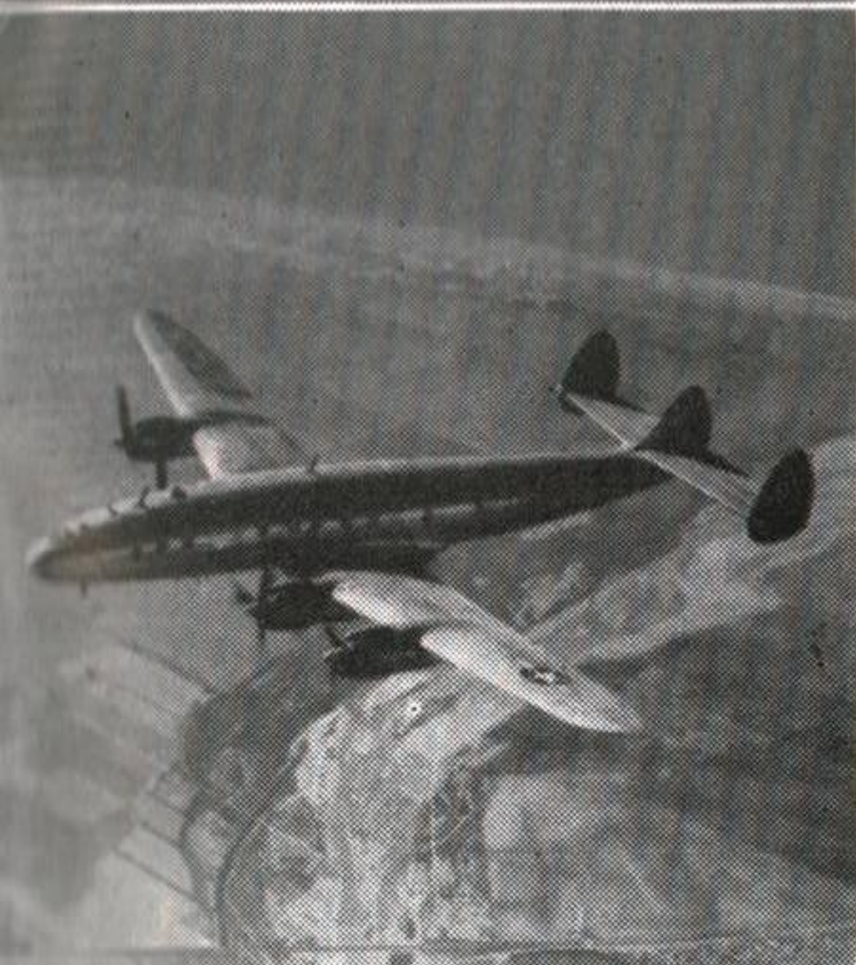
CONSTELLATION (U.S.A.) Commercial and Military Transport U.S.A.F.: C-121 (see photo). U.S. Navy: WV-1 with radomes in nose, above and below fuselage. Civilian version may carry ventral fuselage 'pack'. Span: 123 ft.
