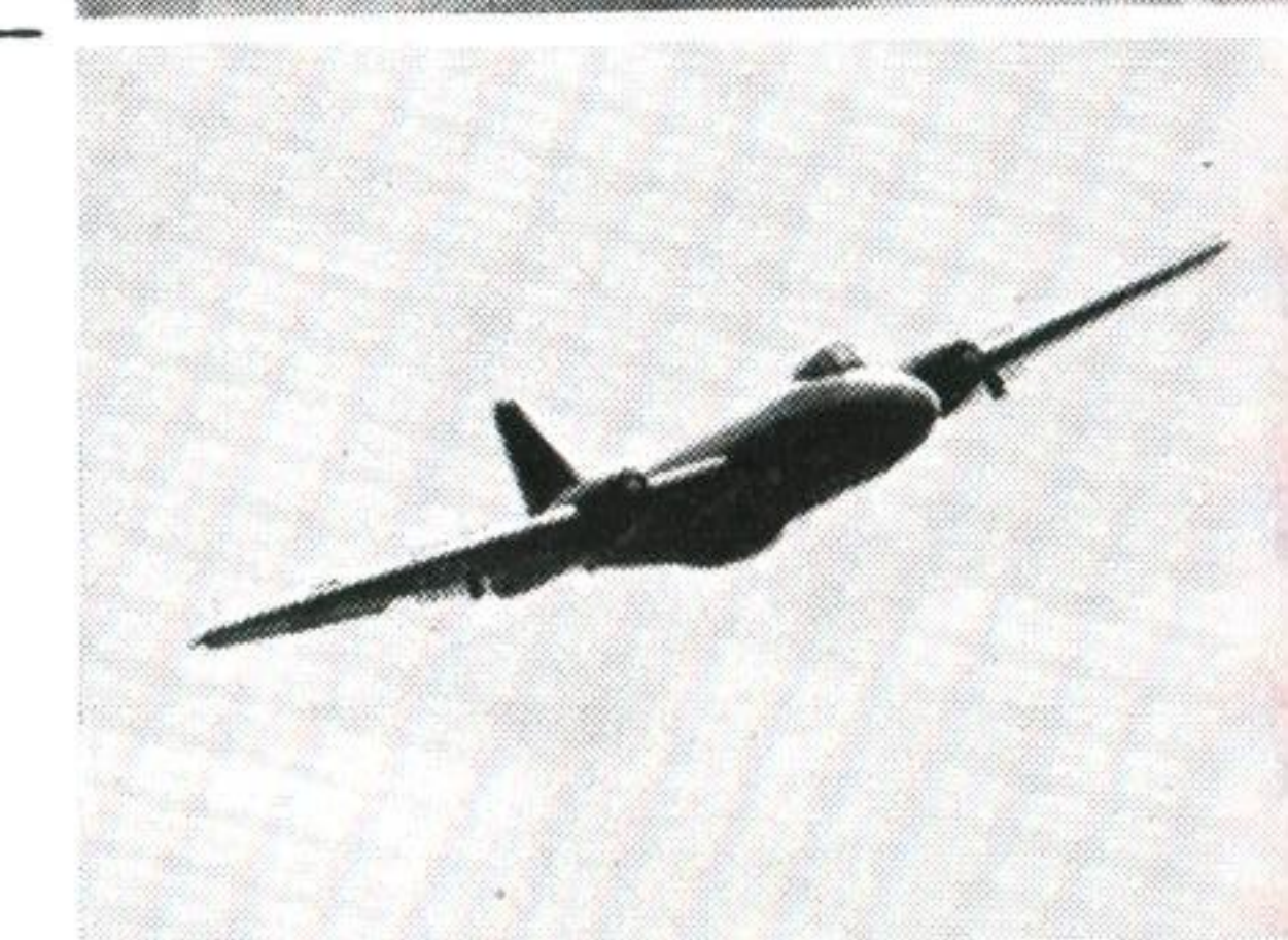
CANBERRA B Mk. 8 (G.B.) Light Bomber Ventral fuselage gun pack may or may not be carried. Wing-tip tanks and/or under-wing stores may be carried. Span: 64 ft.
