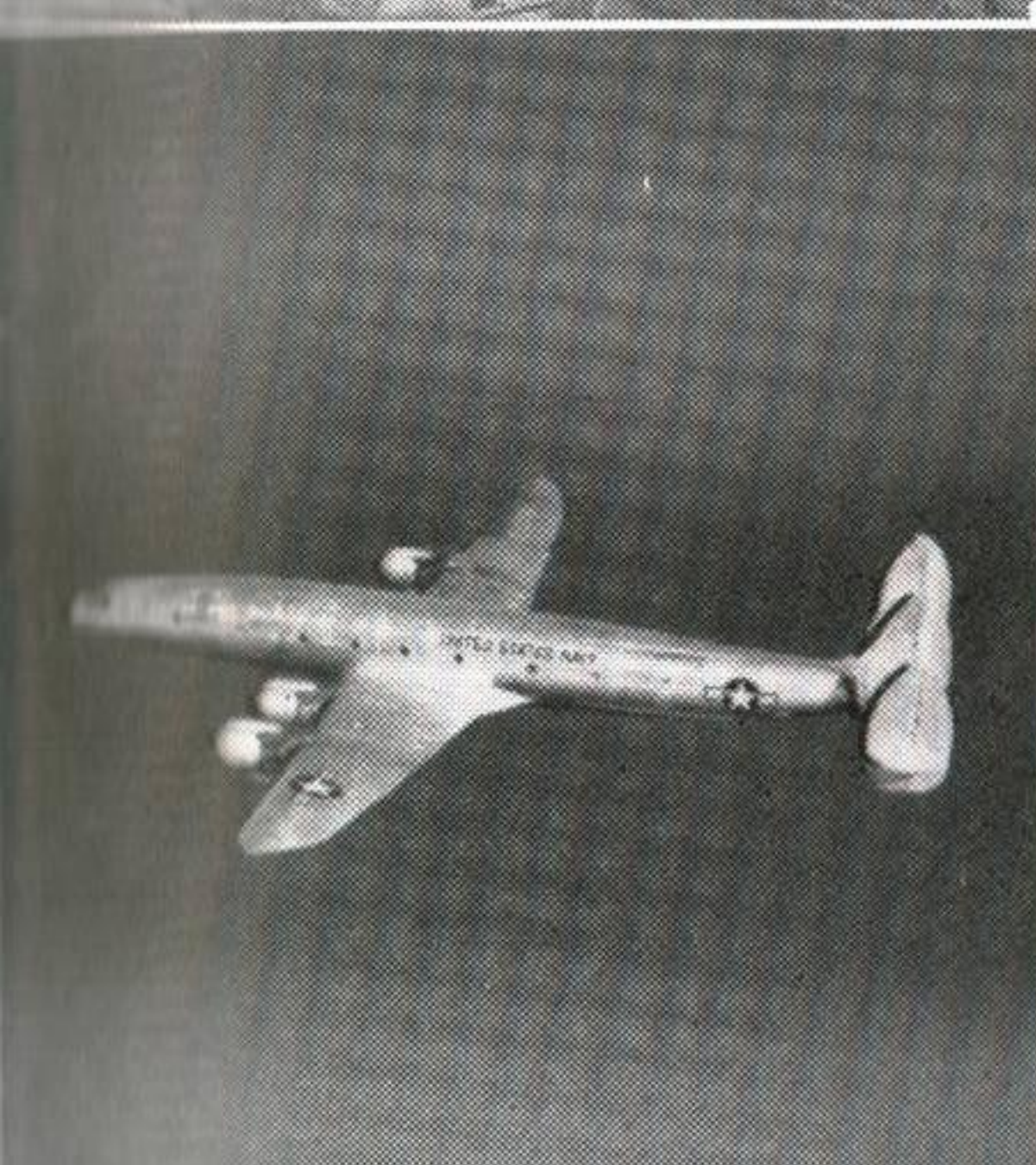
SUPER CONSTELLATION (U.S.A.) Commercial and Military Transport U.S.A.F.: C-121C. U.S. Navy: R7V-1 (see photo). RC-121C (U.S.A.F.) and WV-2 (U.S.N.) carry very large dorsal and ventral radomes, may carry wing-tip tanks, C-134(U.S.A.F.) and R7V-2(U.S.N.) are experimental turbo-prop versions. Span: 123 ft.
