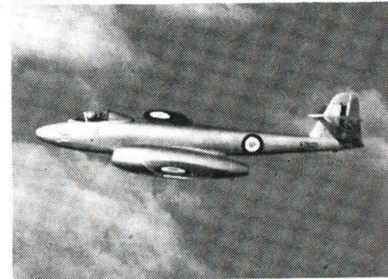
METEOR F Mk. 8 (G.B.) Fighter FR Mk. 9 (inset), similar except for camera windows in nose. Both marks may carry ventral fuselage and/or under-wing tanks. F Mk. 4, similar but with Mk. 7 tail unit. Span: 37 ft.
