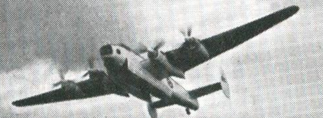
Avro SHACKLETON MR Mk.1 (Four R.R. Griffon radial) Span : 120 ft. Length : 77 ft.
