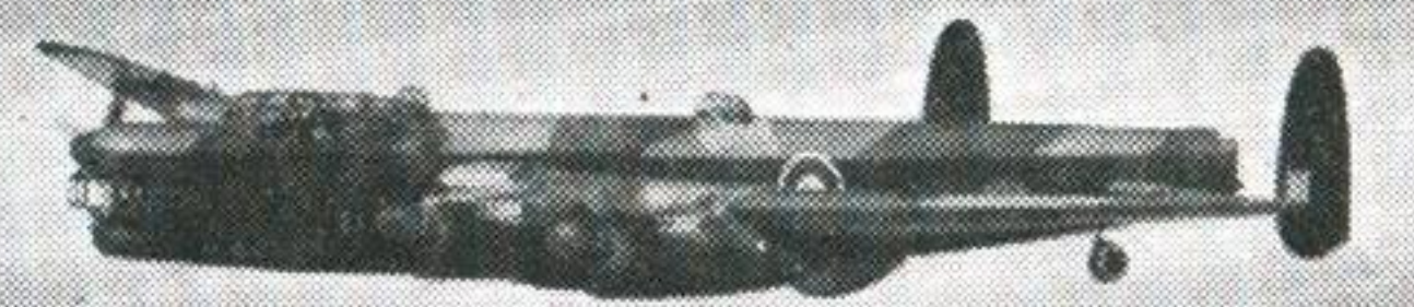
Avro LINCOLN B Mk. 2 (Four R.R. Merlin radial) Span : 120 ft. Length : 78 ft. 3 in.
