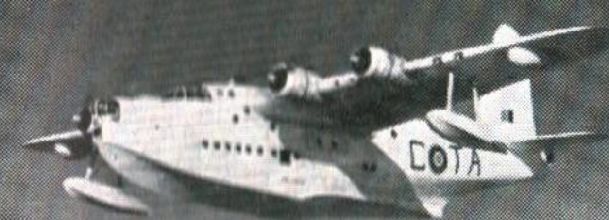
Short SUNDERLAND GR Mk.5 (Four P & W Twin Wasp radial) Span : 112 ft. 9 in. Length : 85 ft. 4 in.
