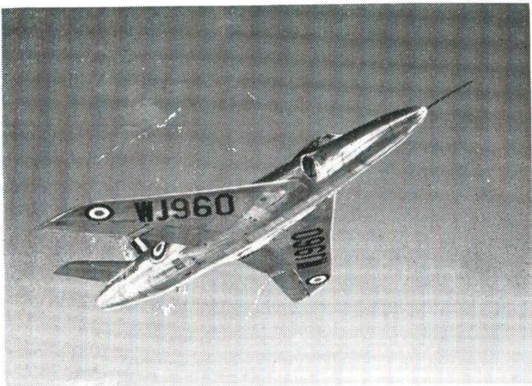
Cover Photo : Vickers Supermarine Swift all-swept jet fighter, in super-priority production for the Royal Air Force. The Swift is powered by a Rolls-Royce Avon turbojet.
