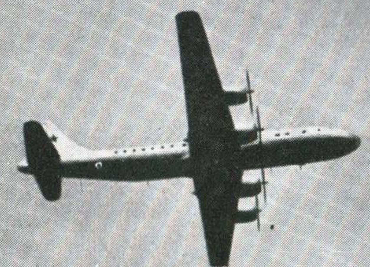
Tupolev TU-70 (Four ASL-90 radial) Span : 141 ft. 3 in. Length : 119 ft.
