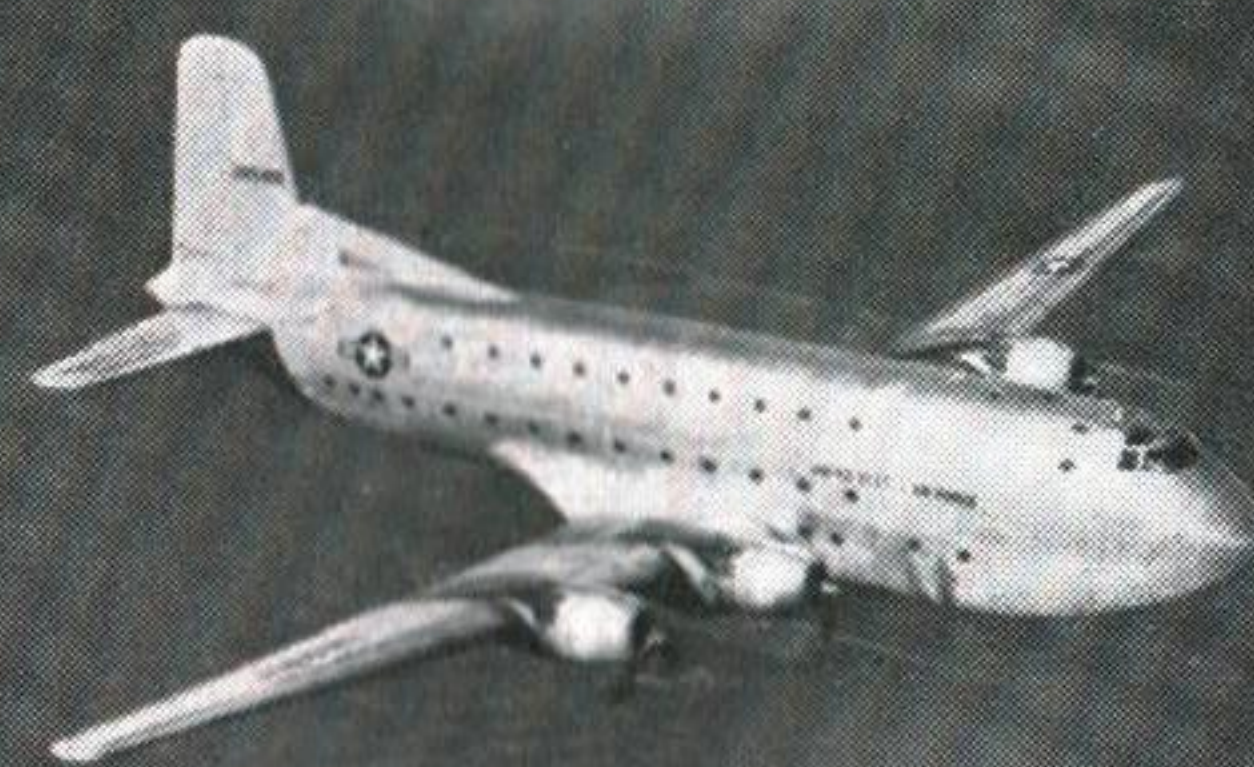
Douglas GLOBEMASTER 2 USAF : C-124A (Four P & W Wasp Major radial) Span : 173 ft. 3 in. Length : 127 ft. 2 in.
