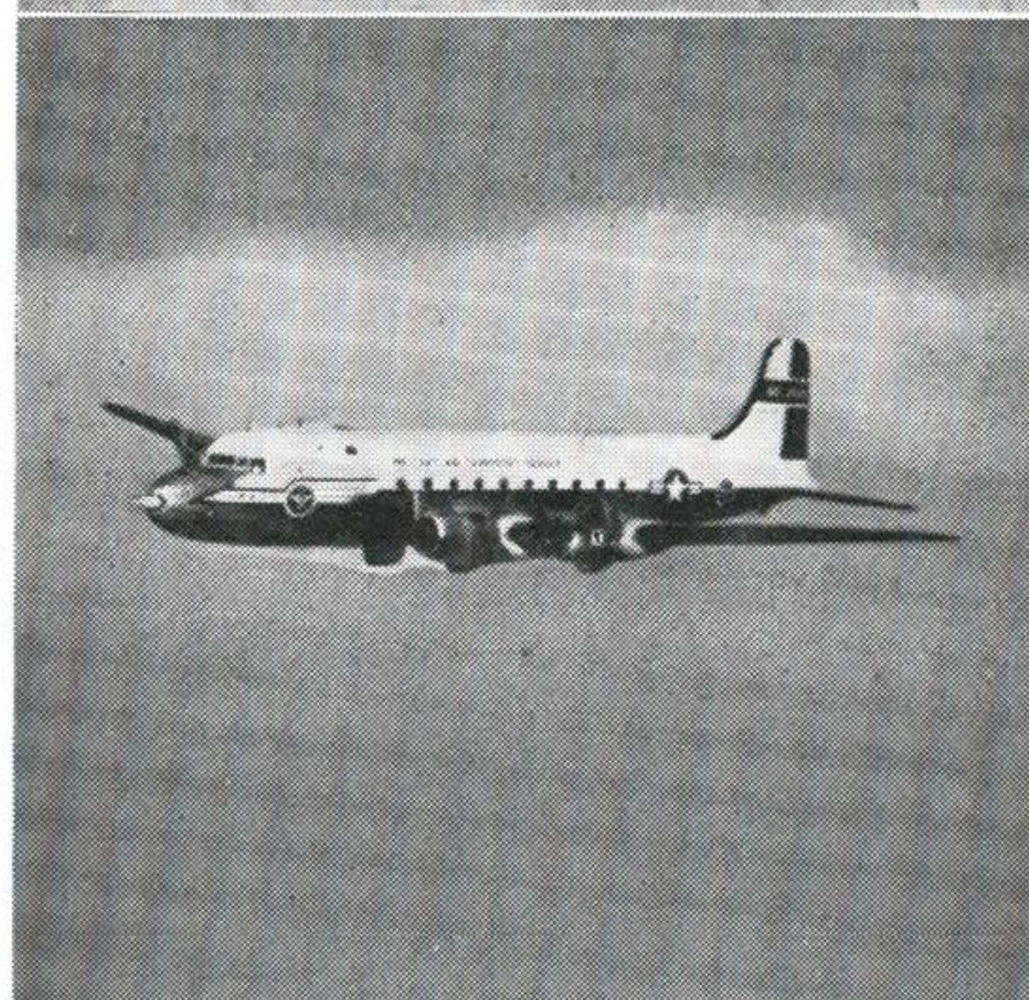
Douglas SKYMASTER (DC-4) USAF : C-54 (Four P & W Twin Wasp radial) Span : 117 ft. 6 in. Length : 93 ft. 11 in.
