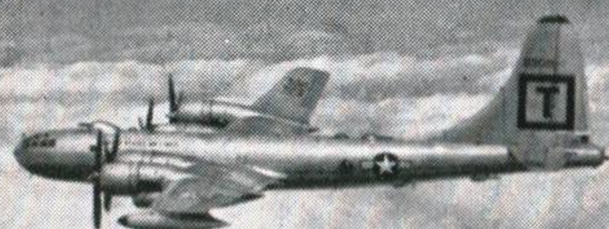
Boeing SUPERFORTRESS USAF : B-50A (Four P & W Wasp Major radial) Span : 141 ft. 3 in. Length : 99 ft.
