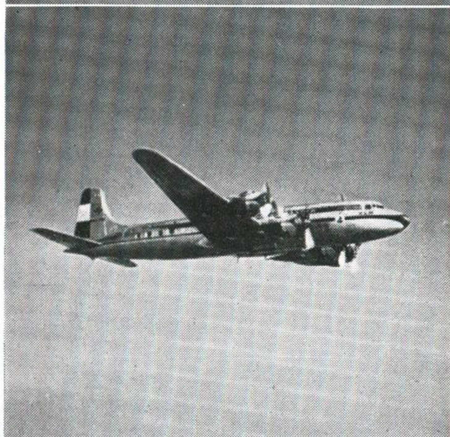
Douglas CLOUDMASTER (DC-6) USAF : C-118 (Four P & W Double Wasp radial) Span : 117 ft. 6 in. Length : 100 ft. 7 in.
