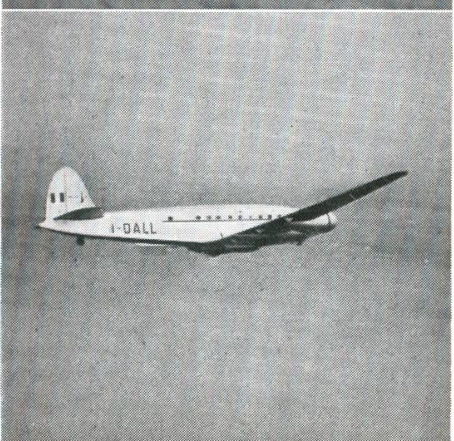
Siai-Marchetti SM.95 (Four P & W Twin Wasp radial) Span : 112 ft. 5 in. Length : 81 ft. 3 in.
