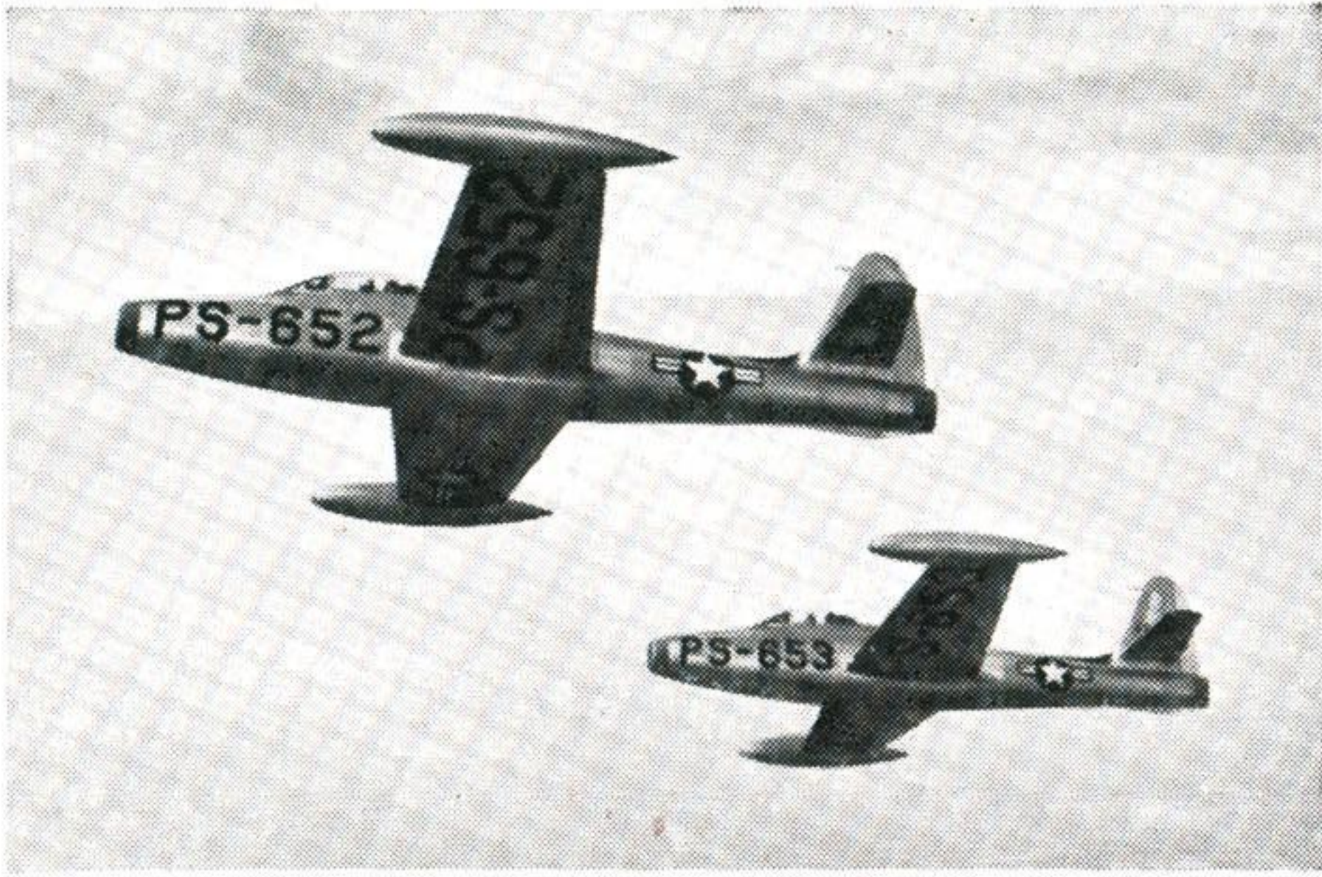
COVER: Republic Thunderjets characterized by near rectangular wings and tailplane, pear-shaped fin and rudder and a fuselage which suggests to us the nickname "Thunderbottle."
