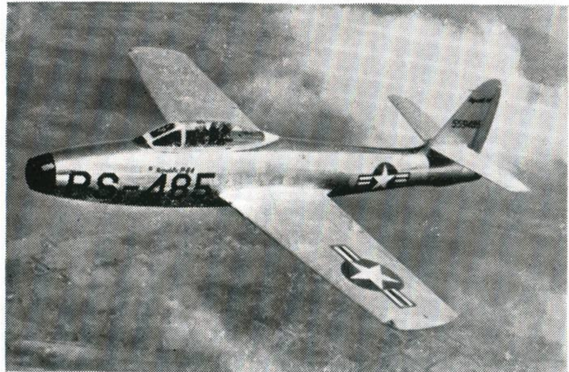
COVER: Republic Thunderjets characterized by near rectangular wings and tailplane, pear-shaped fin and rudder and a fuselage which suggests to us the nickname "Thunderbottle."
