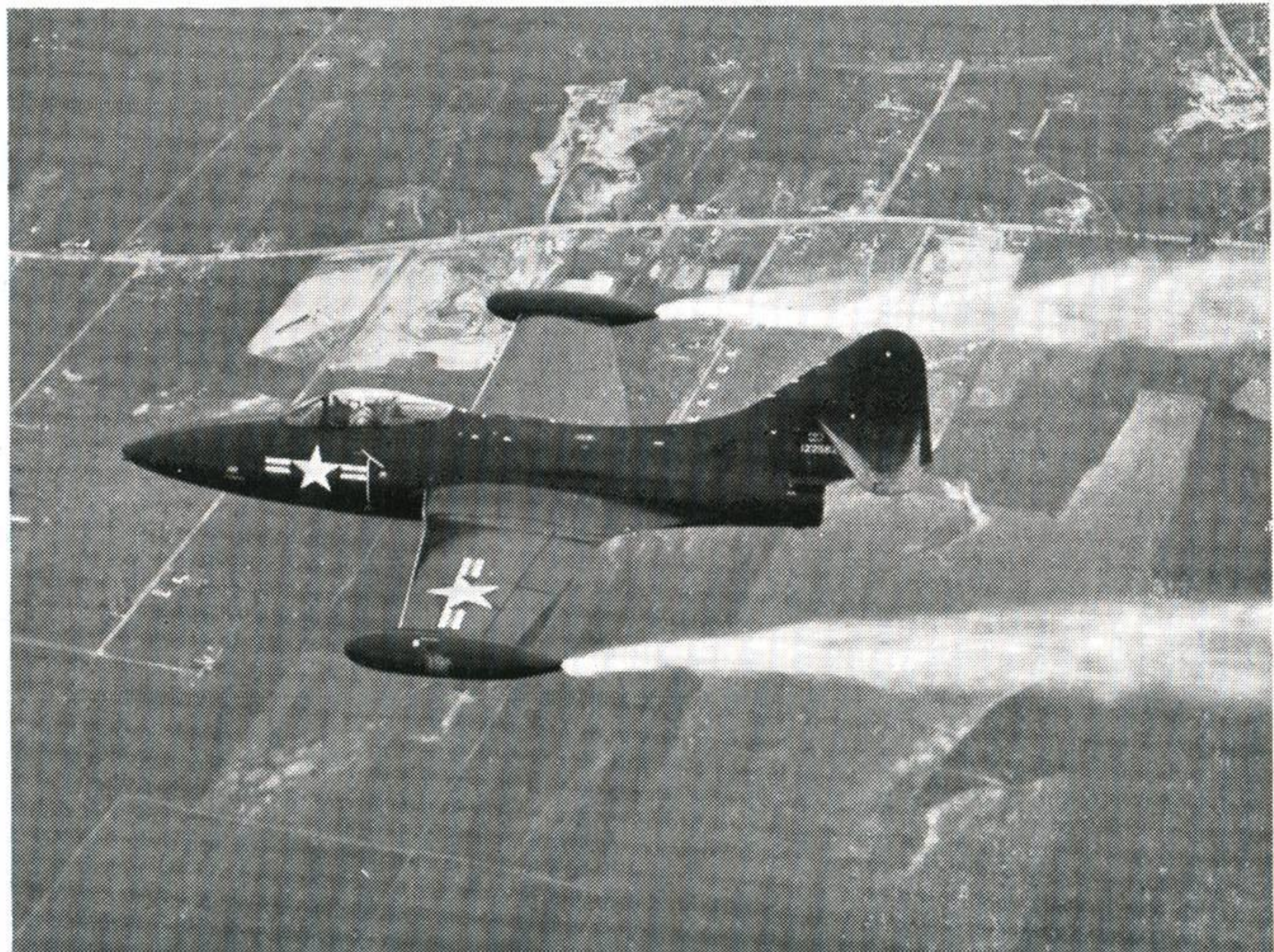
Tip Tank Tactics by a Grumman F9F-3 Panther. Fuel is being exhausted by air pressure.
