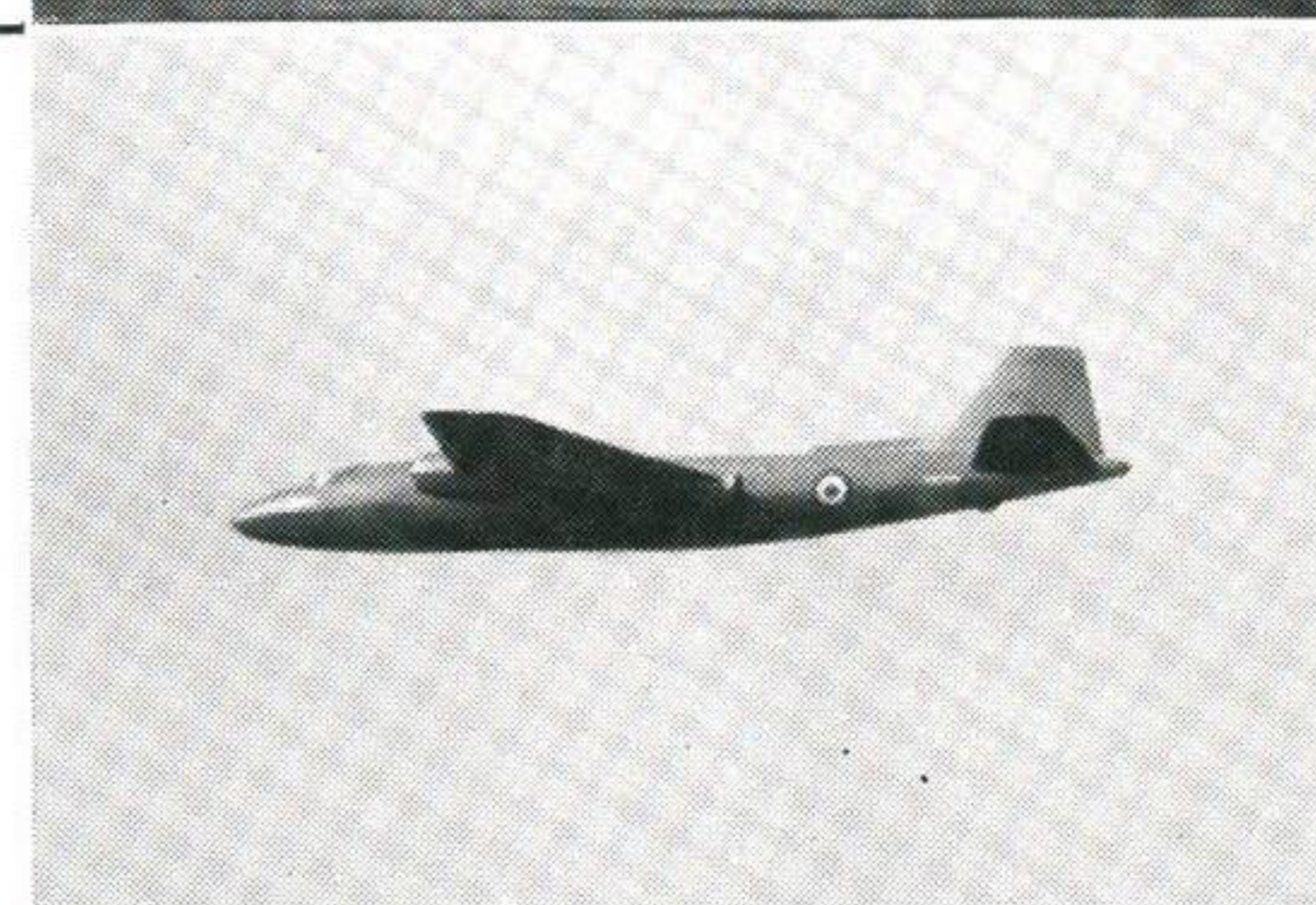
English Electric CANBERRA B Mk. 1 (Two Avon engines) Span 63' 11" Length 66' 3"
