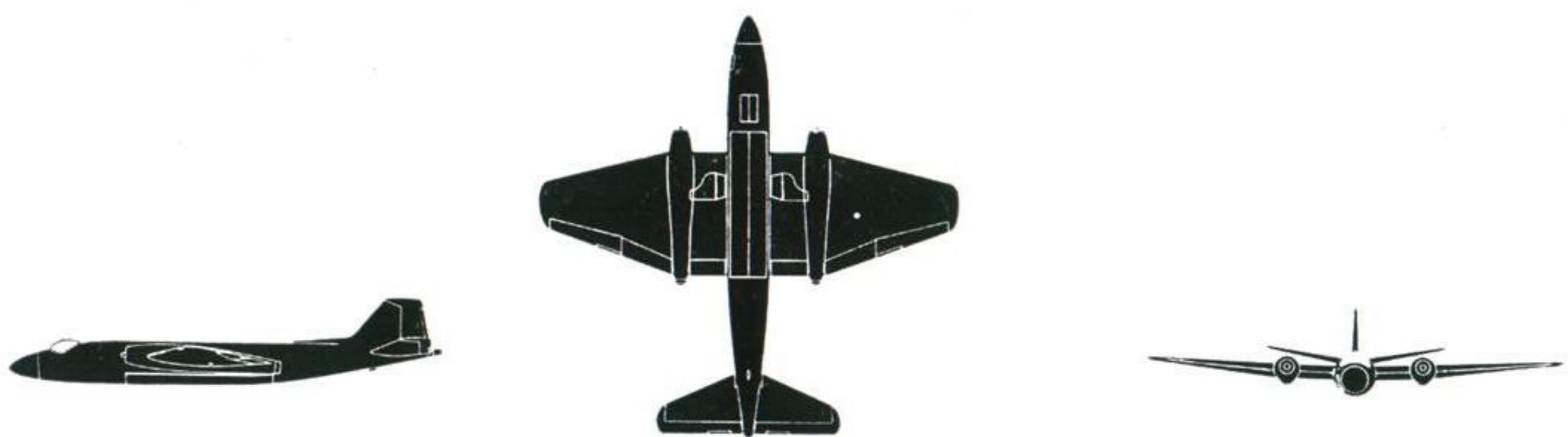
English Electric CANBERRA B Mk. 1 (Two Avon engines) Span 63' 11" Length 66' 3"
