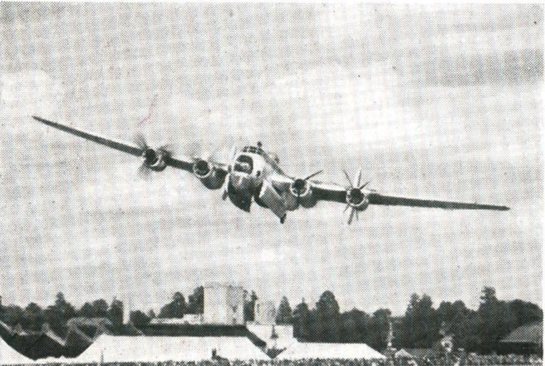
Cover Photo: Billowing clouds (and crowds) form a dramatic backcloth for this Avro Shackleton GR Mk. I seen taking-off at Farnborough last year. Views below show the Shackleton with open bomb-doors; its "stings" (tail and mid-upper); the deep fuselage; the outsize fins and rudders; and the distinguishing "wart" under its nose.
