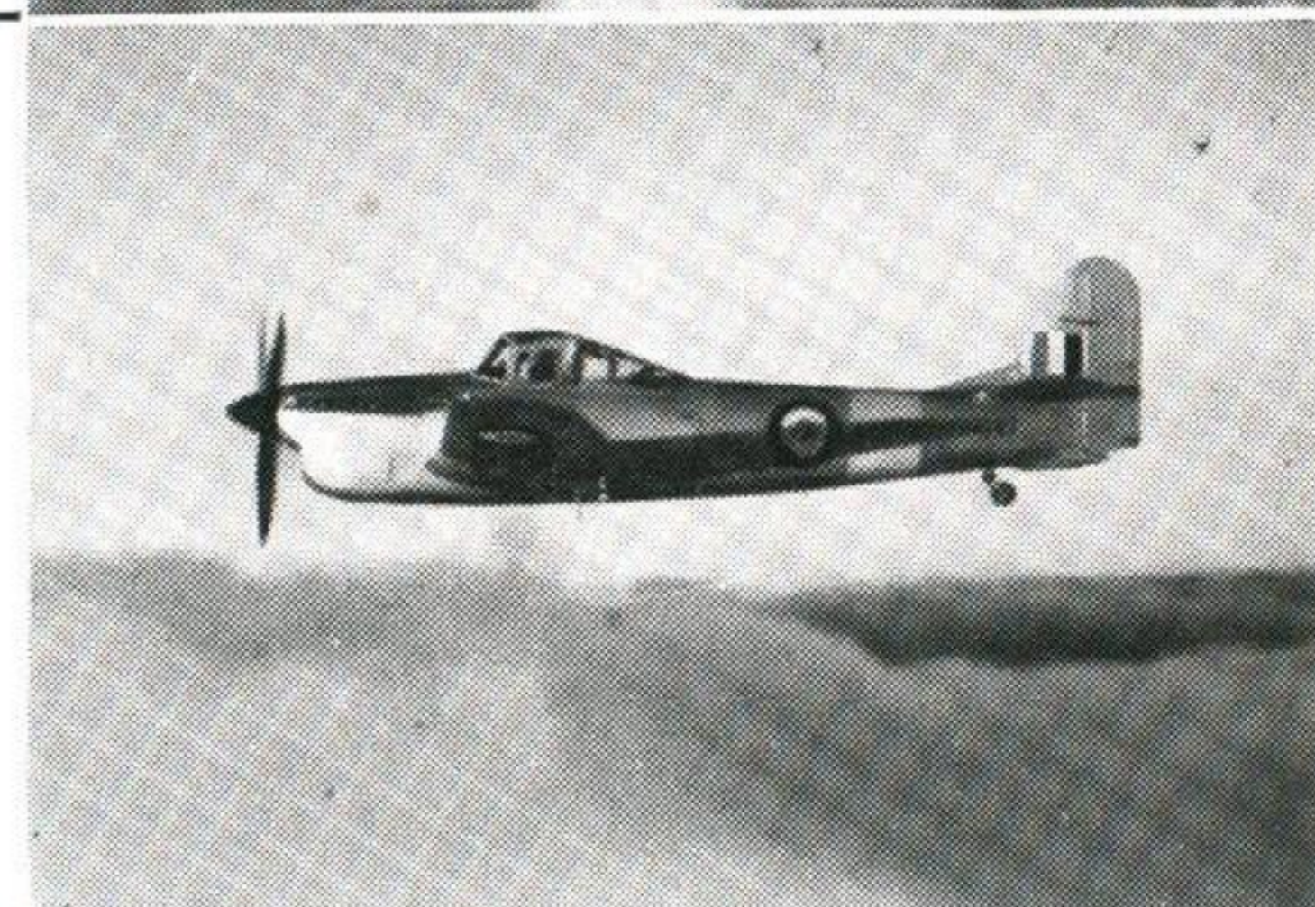
Avro ATHENA T Mk. 2 (One Merlin 35 engine) Span 40' 0" Length 37' 6"
