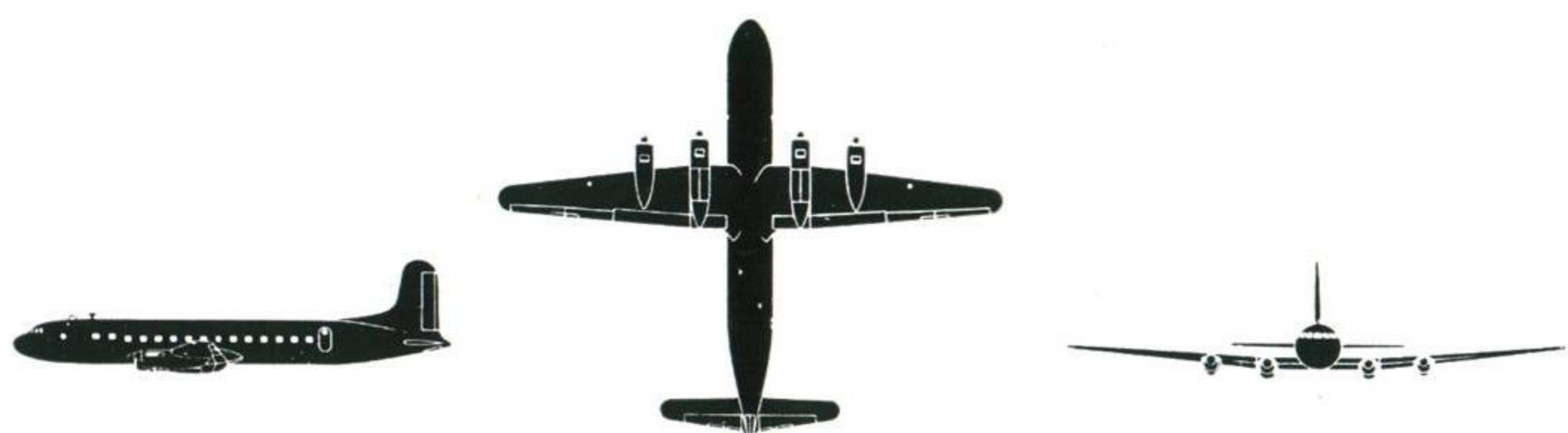
Avro TUDOR 2 (Four Merlin 621 engines) Span 120' 0" Length 106' 7" (Tudor 5 is the same except for circular windows)
