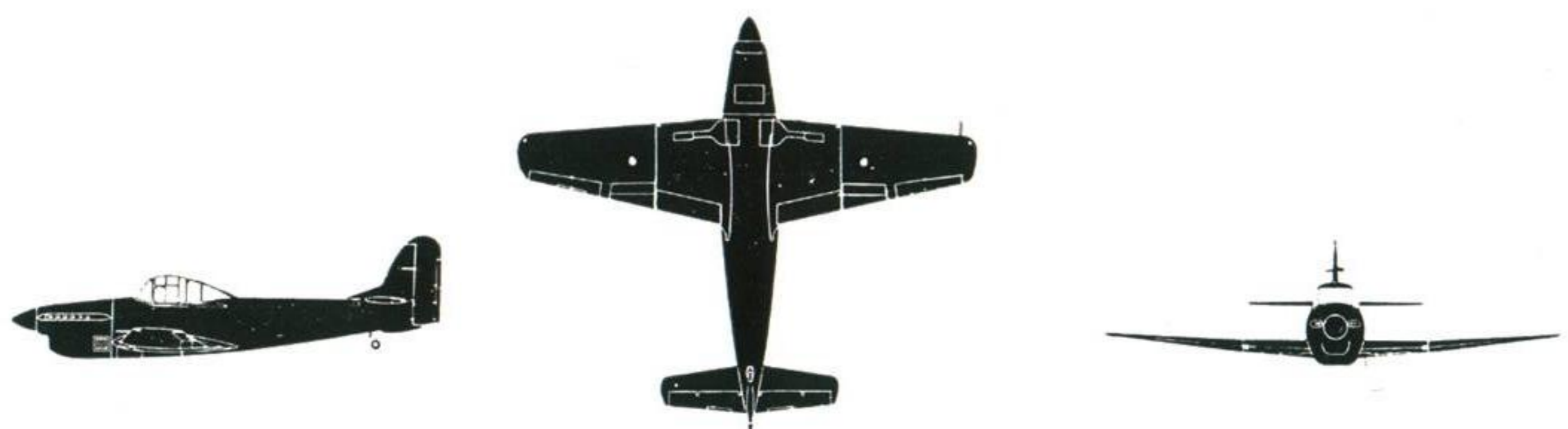
Avro ATHENA T Mk. 2 (One Merlin 35 engine) Span 40' 0" Length 37' 6"
