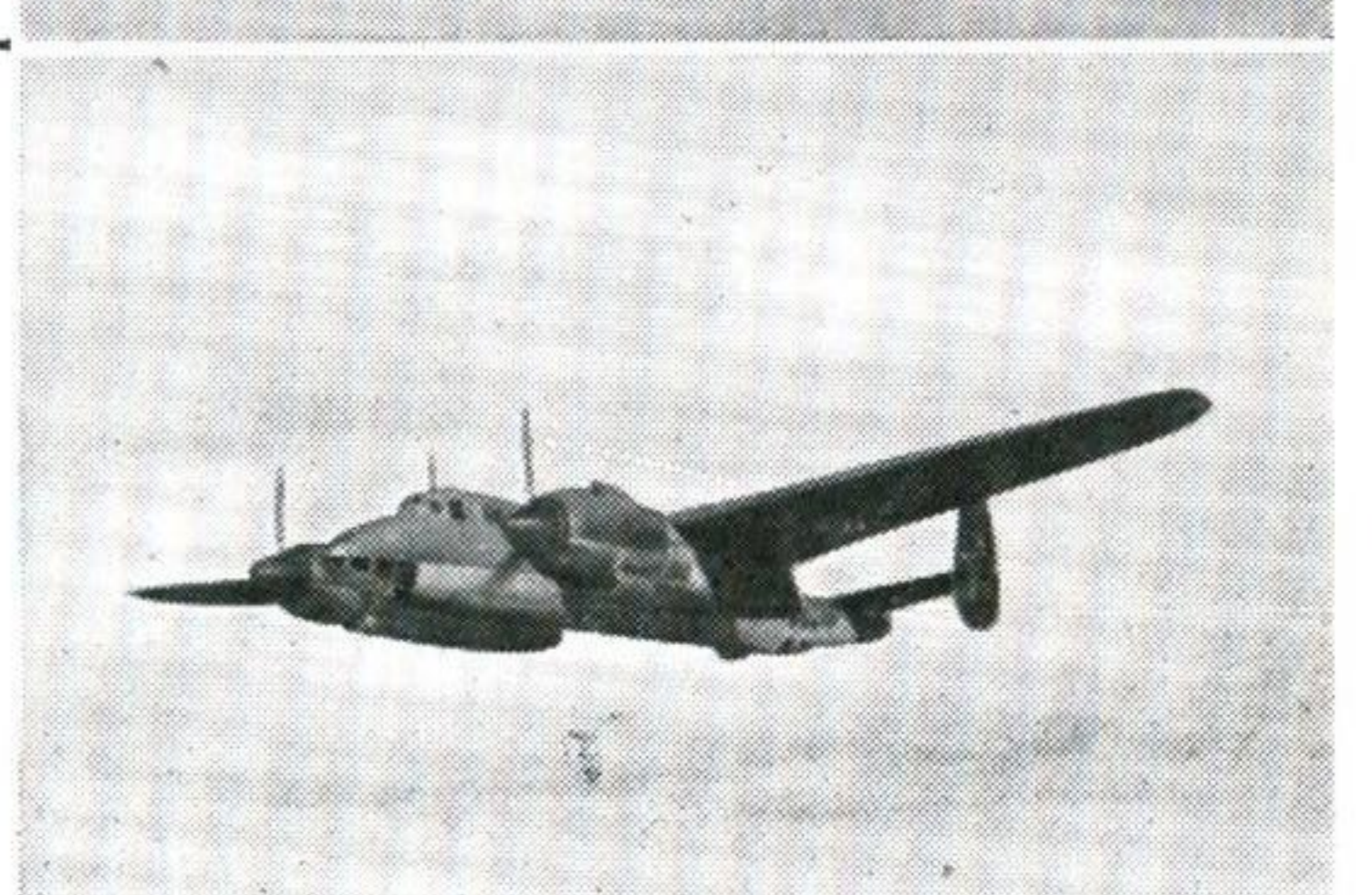
TU-2 (Bomber) (Two ASH.82 FNV engines) Span 60' 11" Length 45' 3"
