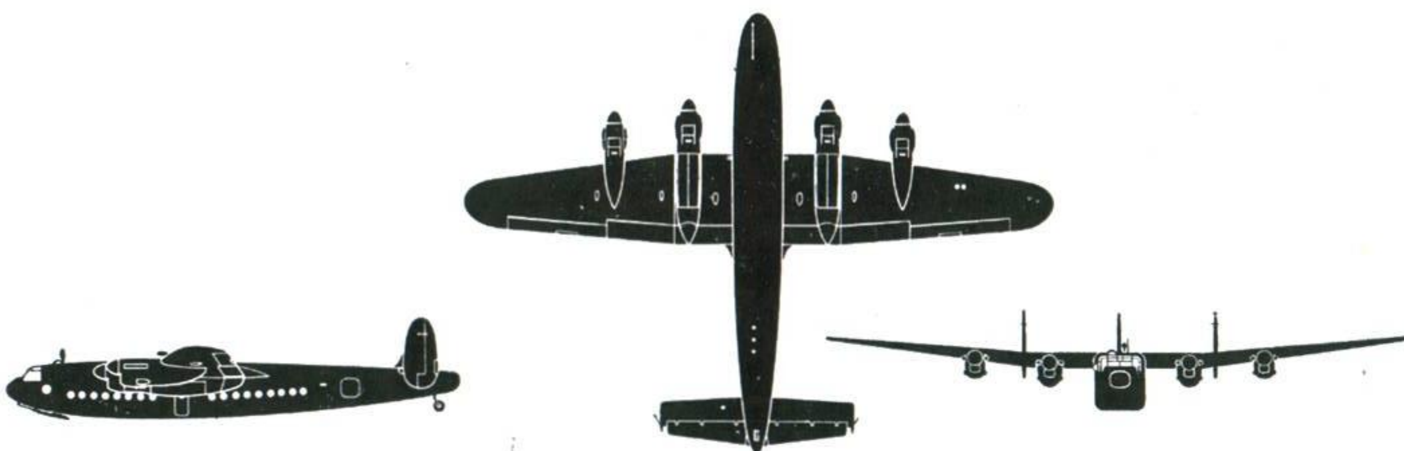
Avro YORK (Four R-R. Merlin 24 engines) Span 102' 0" Length 78' 0"
