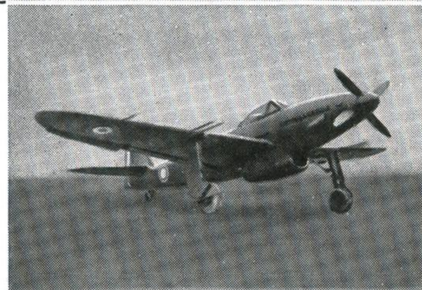
Arsenal VB.10 (Fighter) (Two Hispano Suiza 122 engines) Span 50' 9" Length 42' 6"
