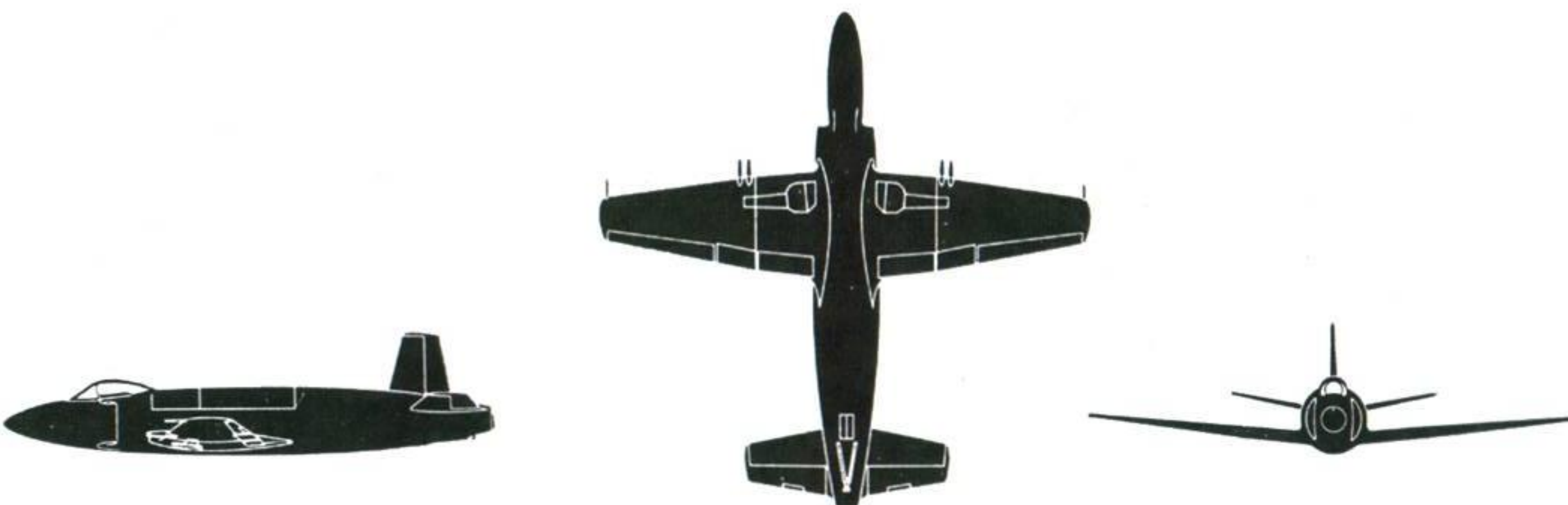
Supermarine ATTACKER F Mk. 1 (One R-R. Nene 1 engine) Span 36' 11" Length 37' 6"
