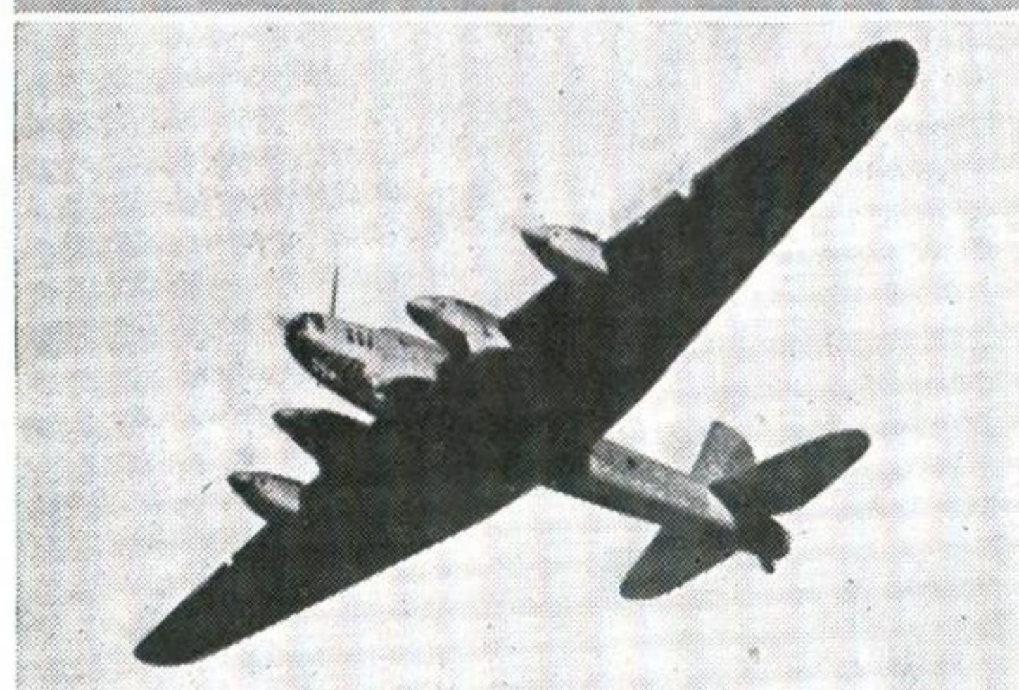
PE-8 (Bomber) (Four AM.35A engines) Span 131' 3" Length 80' 6"
