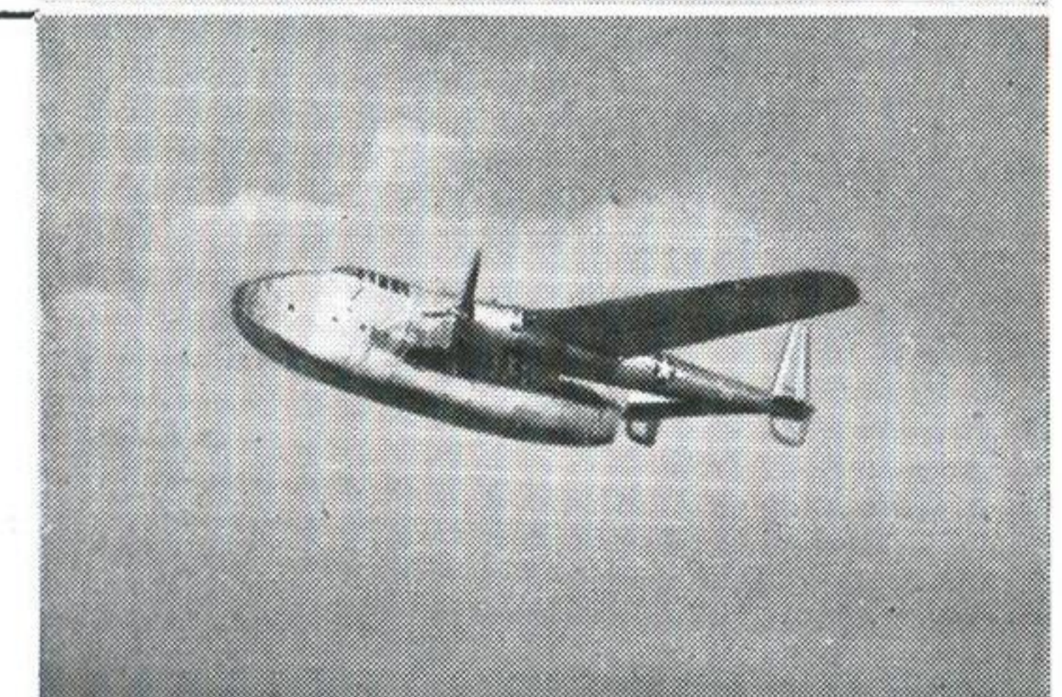
Fairchild C-82 PACKET (Two Double Wasp engines) Span 106' 5" Length 77' 2"
