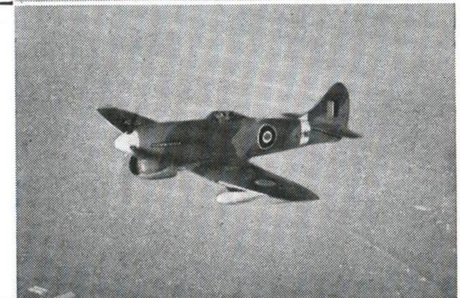
Hawker TEMPEST F Mk. 6 (One Napier Sabre 5 engine) Span 41' 0" Length 33' 8"
