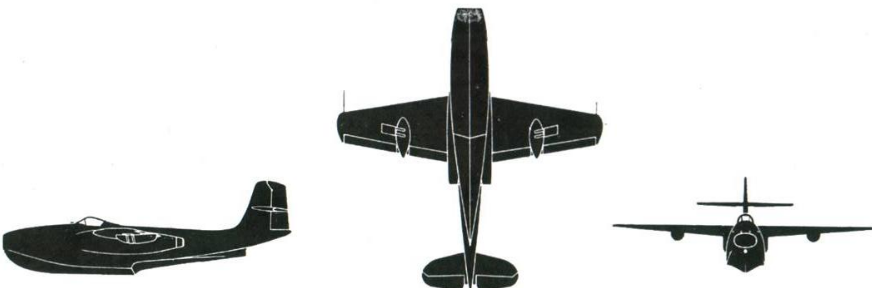
Saunders Roe S.R./A.1 (Two M.V. Beryl 1 or 2 (F.2/4) engines) Span 46' 0" Length 50' 0"
