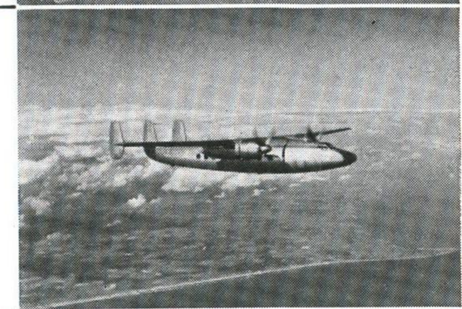
Airspeed AMBASSADOR (Two Bristol Centaurus 661 engines) Span 115' 0" Length 80' 3"
