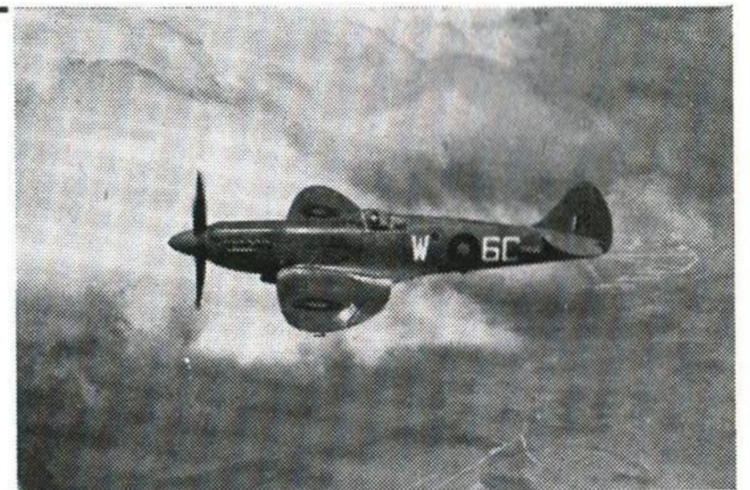
Supermarine SPITFIRE F Mk. 14 (One R-R. Griffon 65 or 85 engine) Span 36' 10" Length 32' 8"
