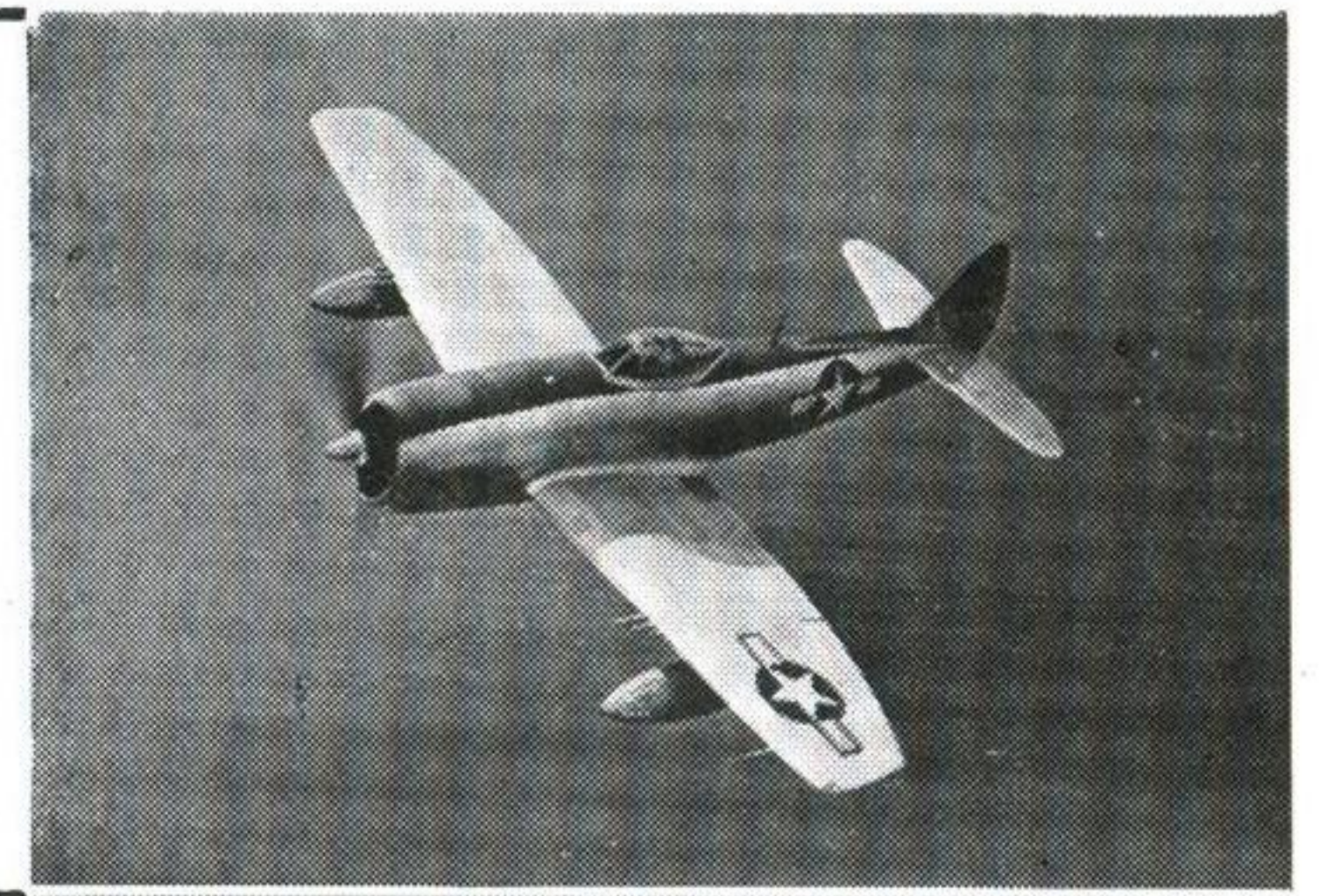
Republic F-47N THUNDERBOLT (One Double Wasp engine) Span 42' 7" Length 36' 2"
