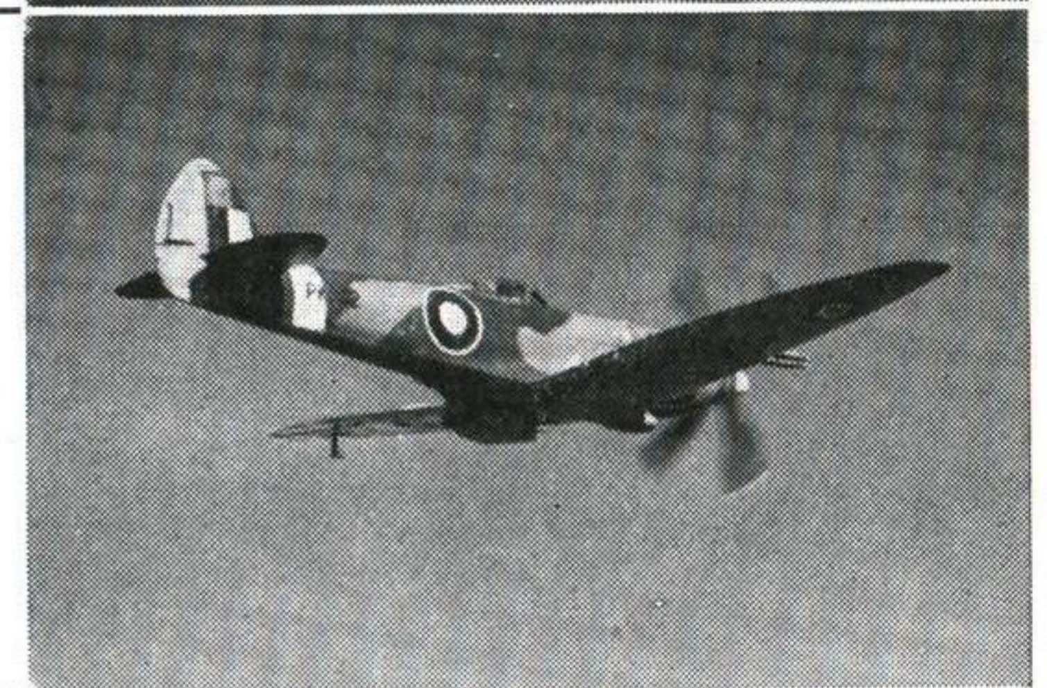
Supermarine SPITFIRE F Mk. 22 (One R-R. Griffon 61, 64 or 85 engine) Span 36' 11" Length 32' 11"
