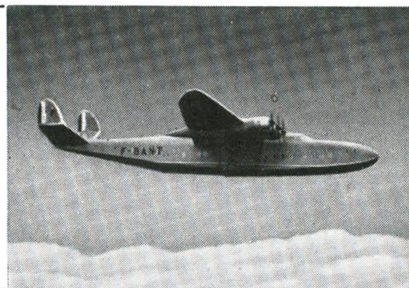
Latécoère 631 (Trans-ocean Transport) (Six Wright Cyclone 14 engines) Span 188' 4" Length 142' 6"
