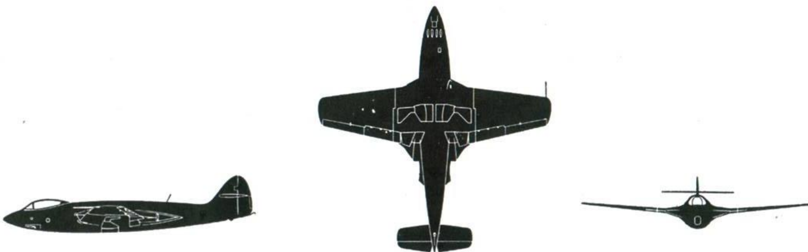
Hawker P.1040 (One R-R. Nene 2 engine) Span 36' 6" Length 38' 4"
