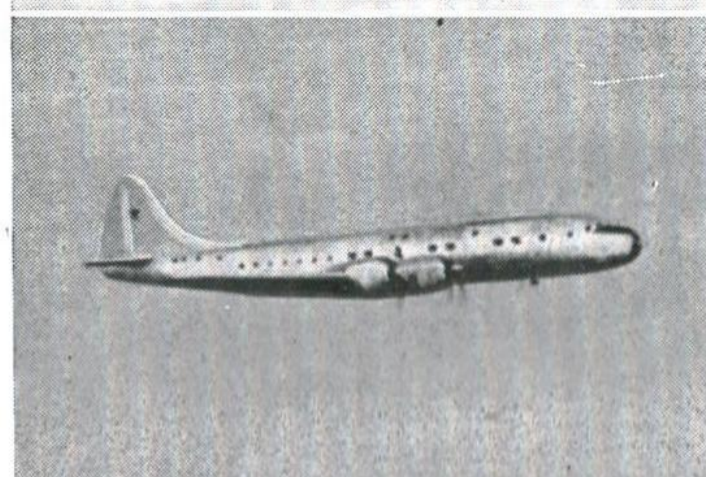
TU-70 (Transport) (Four Russian built Wright W. Cyclone engines) Span 141' 3" Length 119' 0"
