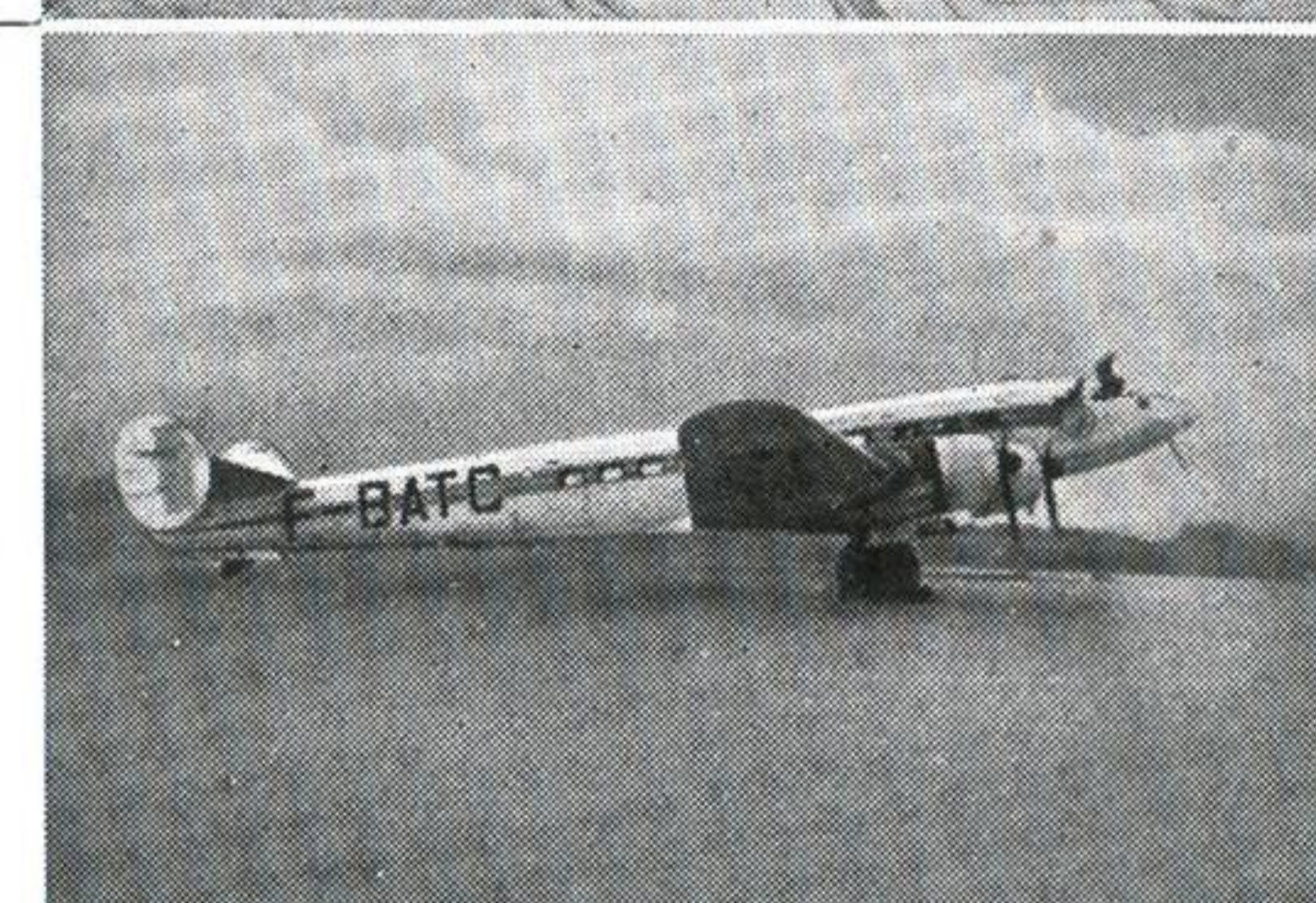
S.N.C.A.S.E. LANGUEDOC 161 (Transport) (Four P. & W. R.1830 engines) Span 96' 6" Length 79' 7"
