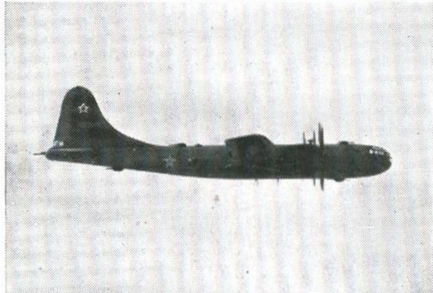
B-29 (Russian-built (Bomber) (Probably Four Russian built W. Cyclone engines) Span 103' 9" Length 74' 9"
