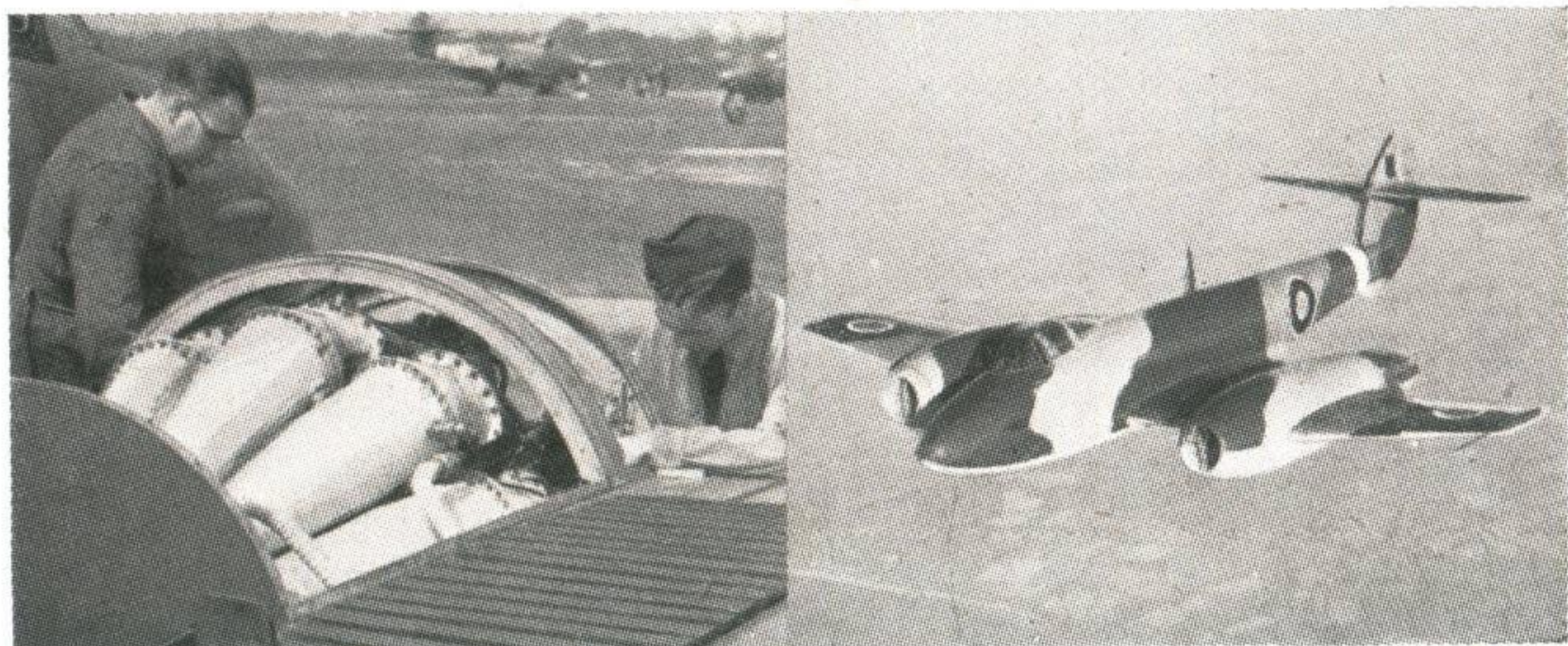
The photograph on the left shows an uncovered Rolls-Royce Derwent turbojet in the starboard engine nacelle of a Gloster Meteor Mk. 3. On the right is a view of the Meteor Mk. 4 showing the centrally-mounted turbojets.
