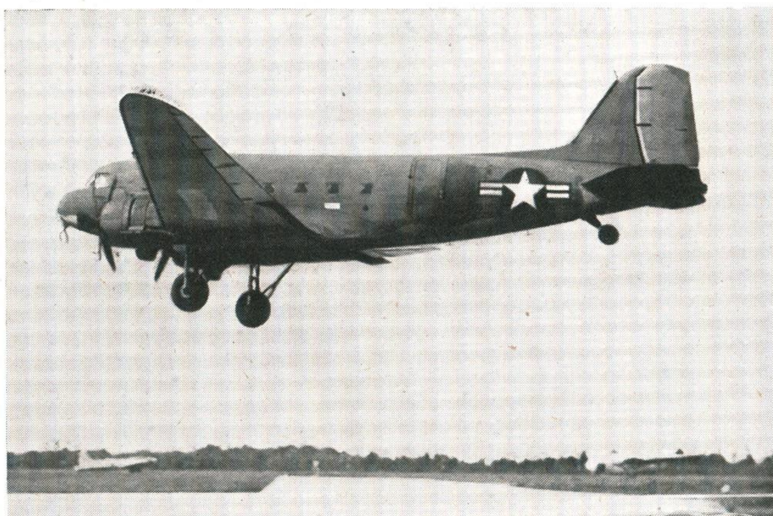
The Douglas C-47 Dakota has a "bicycle" undercarriage of the retractable type. Incidentally, this photograph shows very clearly the exaggerated (apparent) sweep-back of the wing, which has in fact a straight trailing edge. The illusion is due to sharp angle of dihedral in the wing.
