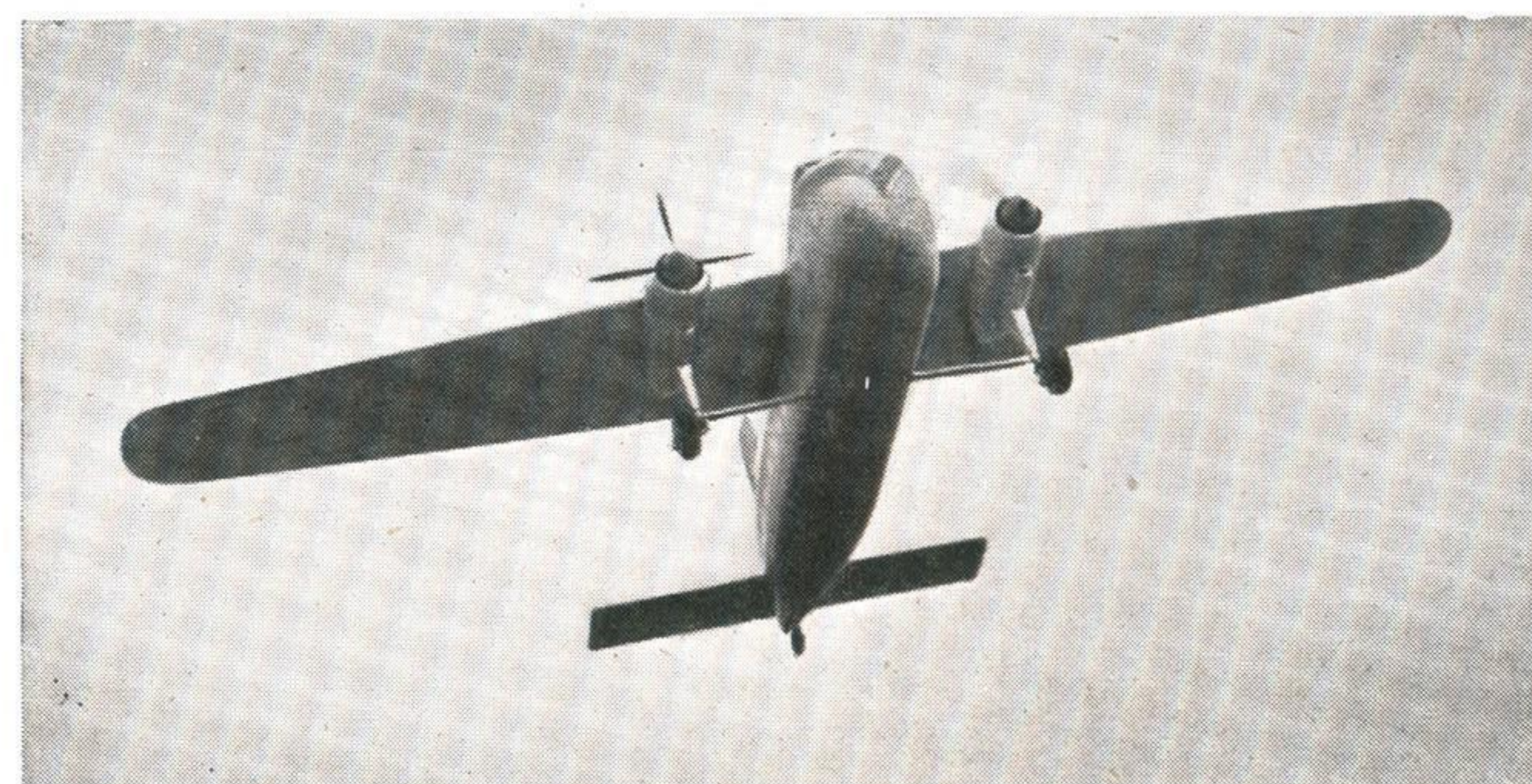
This is a photograph of the new type Bristol 170 Freighter climbing with one engine stopped. The view shows a characteristic aspect of a radial engine and its nacelle. In this aeroplane the engines are close-set (to the fuselage.)
