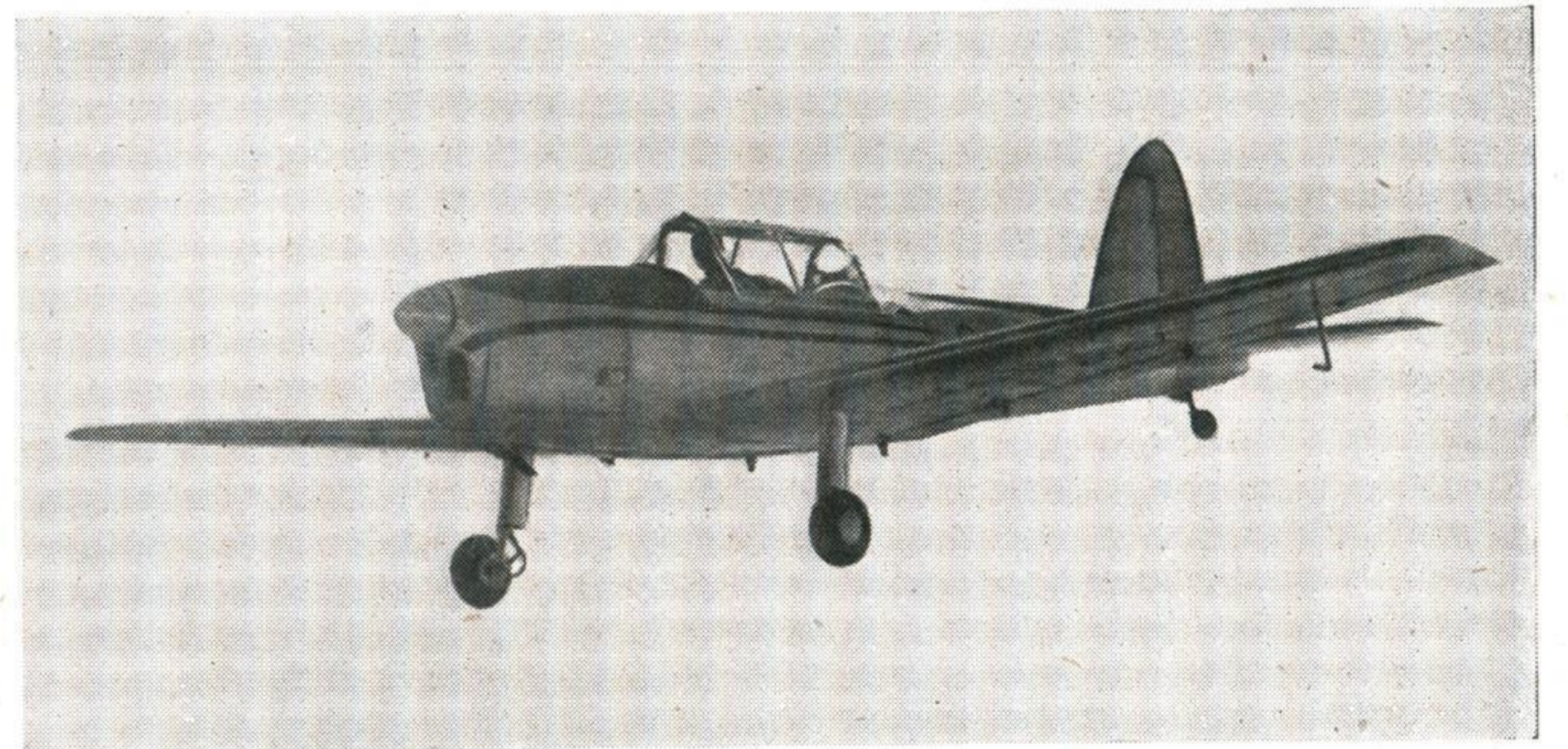
The Bristol Wayfarer (above) and the De Havilland Chipmunk (below) have fixed undercarriages of the bicycle type which are a distinct aid to recognition.
