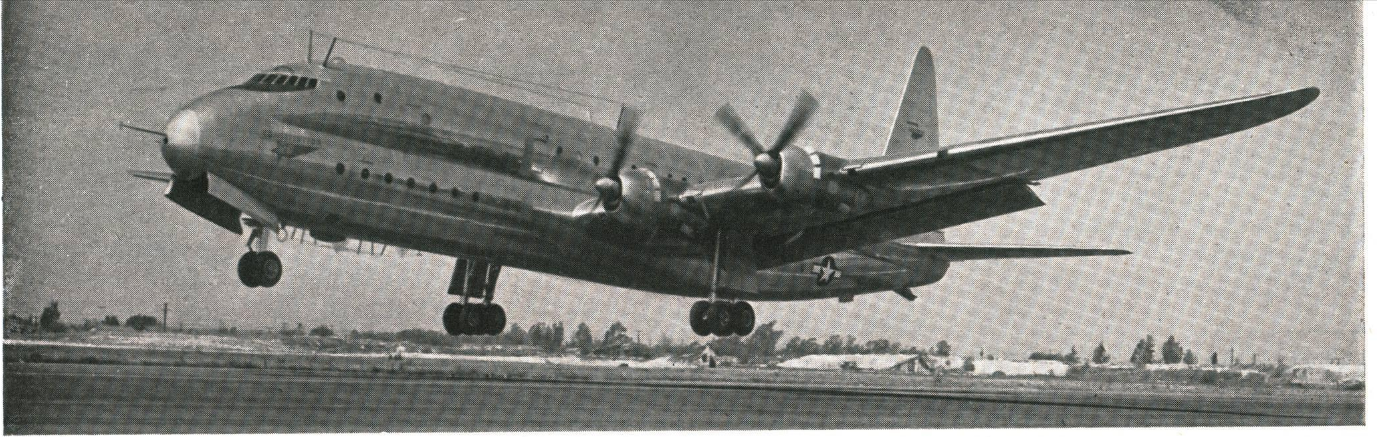
The Lockheed Constitution has a multi-wheel tricycle undercarriage consisting of two pairs of main undercarriage legs each carrying four wheels, and double nose-wheels on a single leg.
