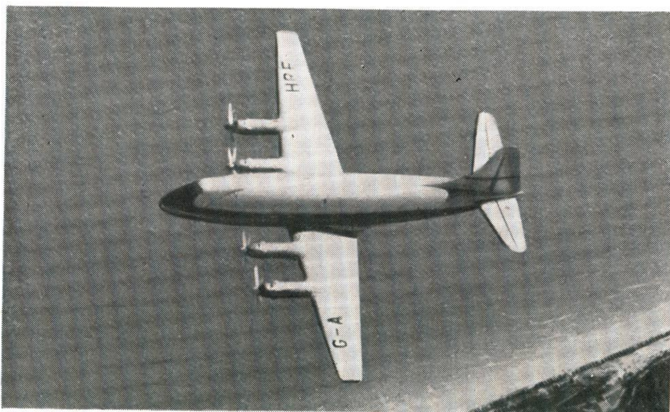
The distinctive "Dart" installation in the Vickers Viscount is shown clearly in this photo. The engines look like four rather thick pencils and have extraordinary length.
