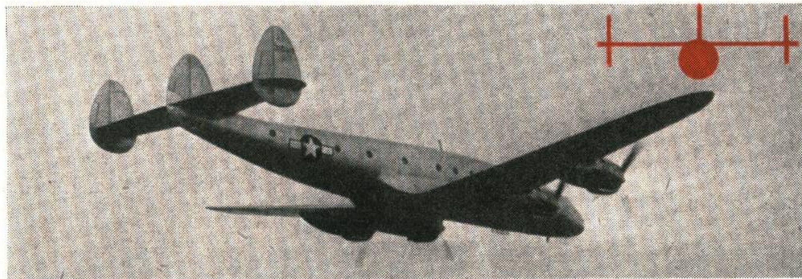
The Lockheed Constellation has the "triple fin and rudder" type, the outer surfaces being inset from the tailplane tips.
