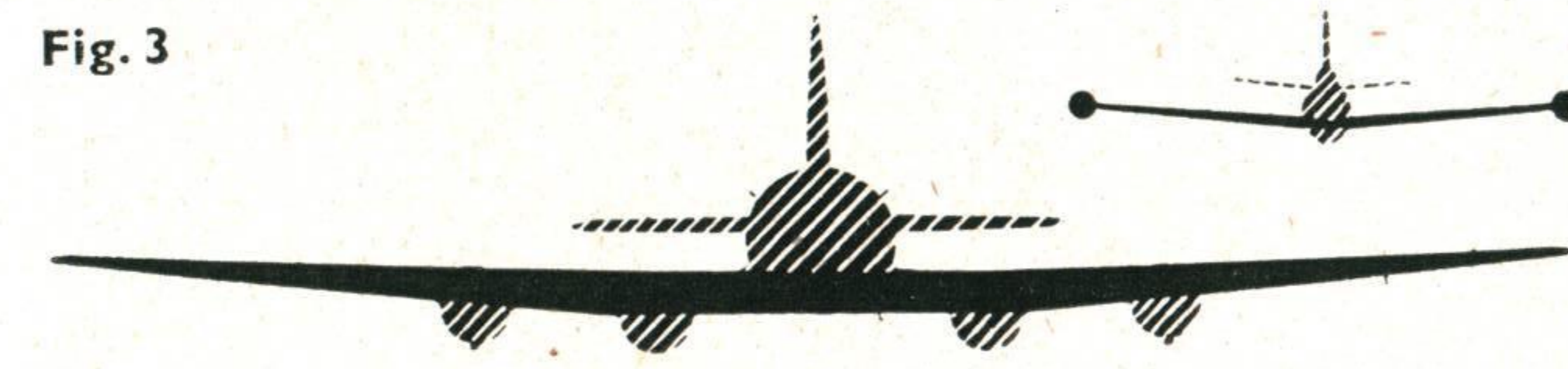
The thick wing of the Handley Page Hastings transport (larger silhouette) is compared with the very thin wing of the Republic F-84 fighter. With a fuselage full of turbojet and such thin wings, the F-84 cannot carry enough fuel internally. Its wing-tip tanks, to give it range, are to some extent a help in recognition.
