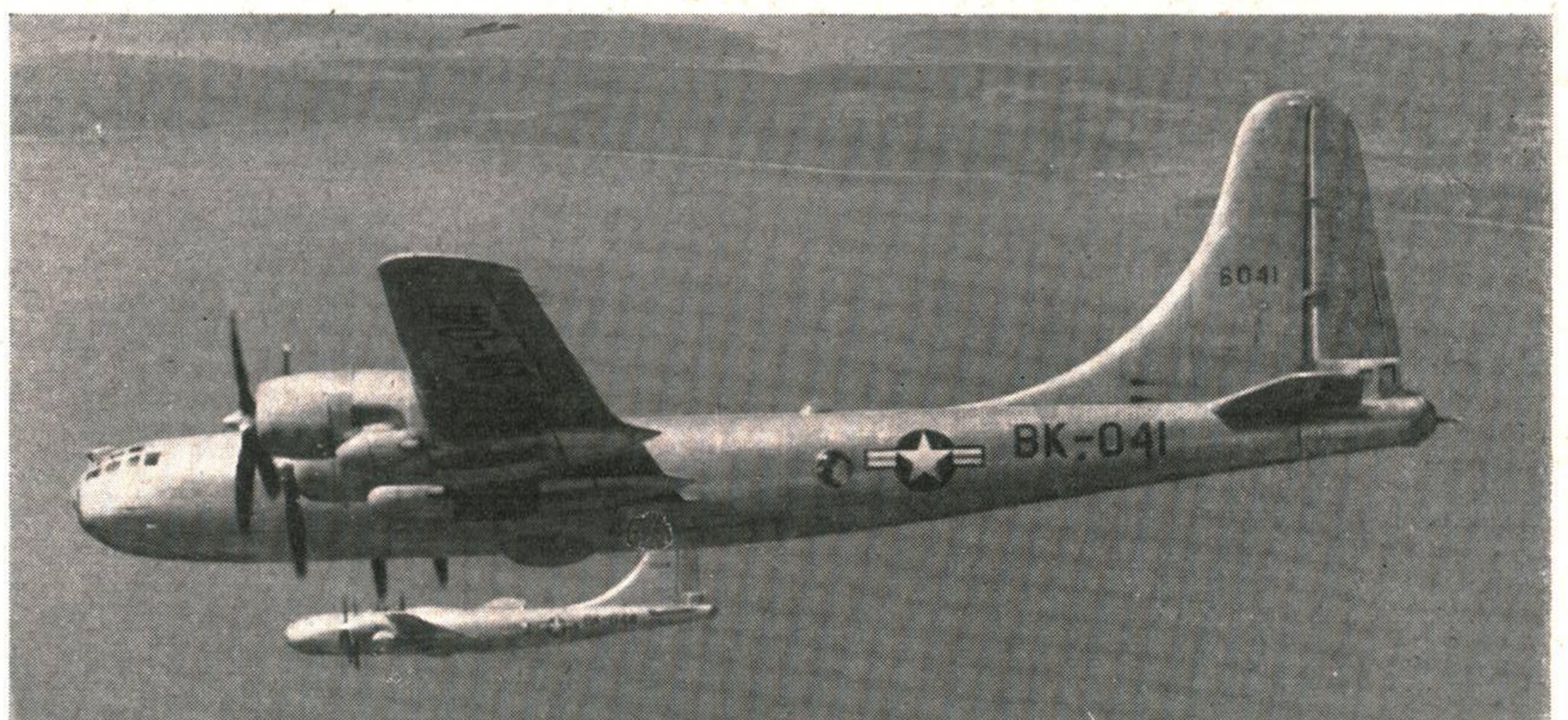
Big-finned Boeing B-50 super-superfortress bombers on a test flight near Seattle (home of Boeing) display great elegance of line and form as they turn. Note detail of engine installation (four Pratt-Whitney Wasp Major radials of 3,500 h.p. each). If you can imagine 14,000 horses in a large field (frankly we can't!) hauling an airframe such as this, you will have some idea of the power they use and not marvel too much at a top speed of over 400 m.p.h. for a bomber of this size. The next instalment in this exciting series of aeroplanes will be the Boeing XB-54 (powered by Wasp Compound engines).
