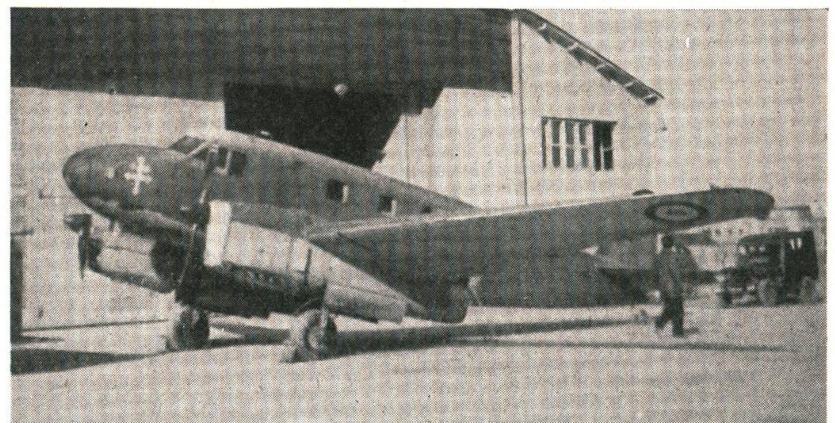
Goeland's (light transport) points are high-riding fin and rudder far behind back-tapered tail-plane; sharply cut back wing panels, and two long narrow boat-like engine nacelles. The Goeland looks rather severely cut generally. (Silhouette: June, 1943 Journal ).
