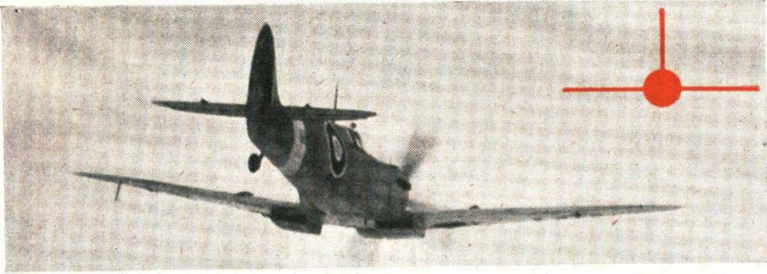
The Spitfire's tail-unit is of the simplest and most common type—horizontal and vertical surfaces intersecting.
