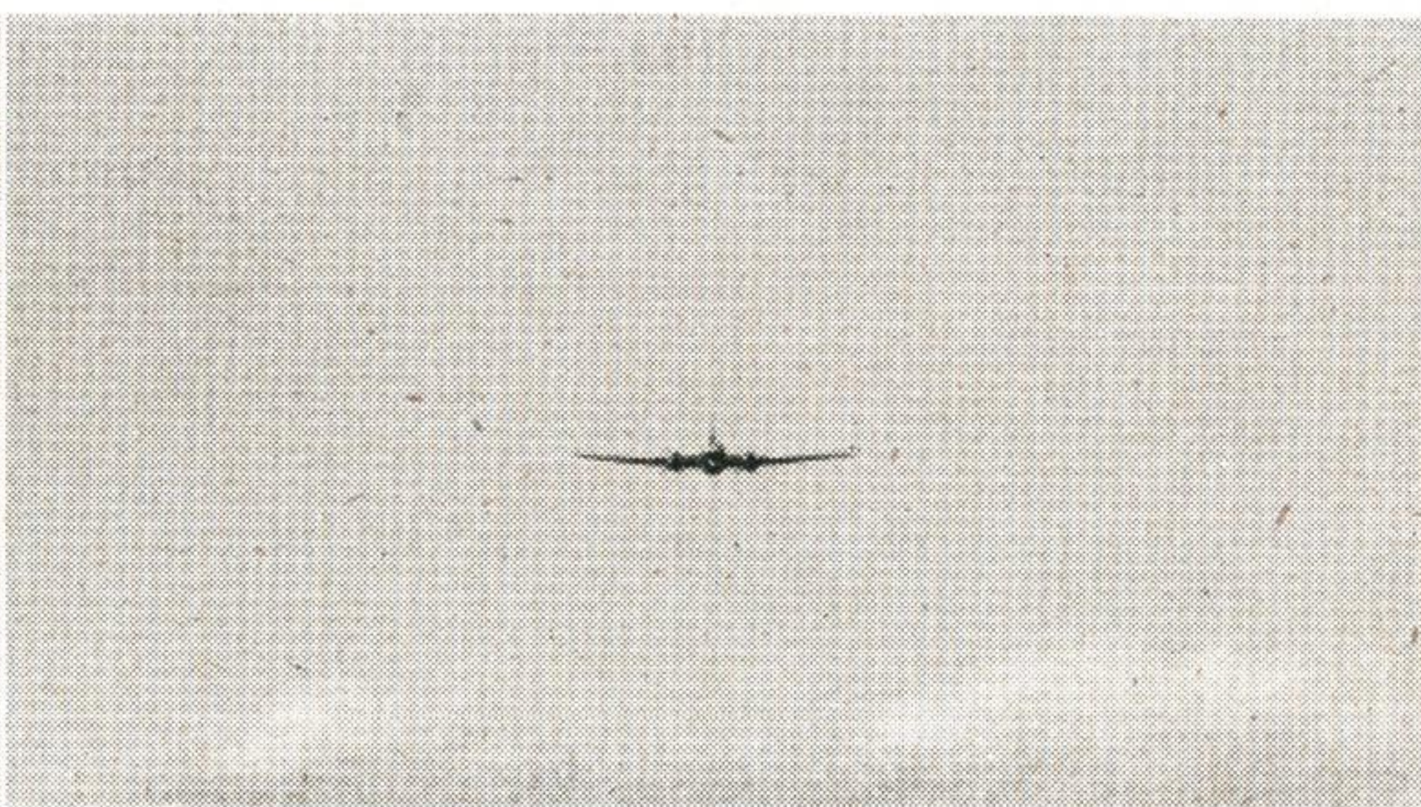
close-set engines—slight dihedral after all—single fin and rudder—
