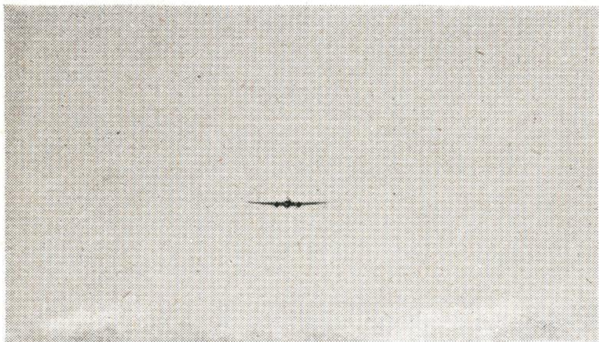
Twin-engines centrally-mounted—wide-span wing—no dihedral angle—
