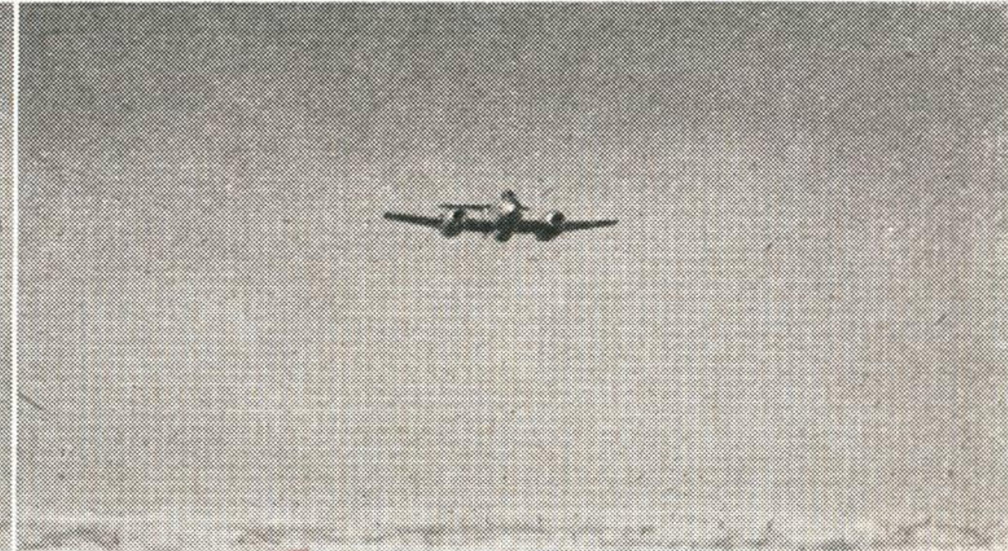
turbojets—low-wing after all, belly-tank on fuselage—small cockpit on nose—
