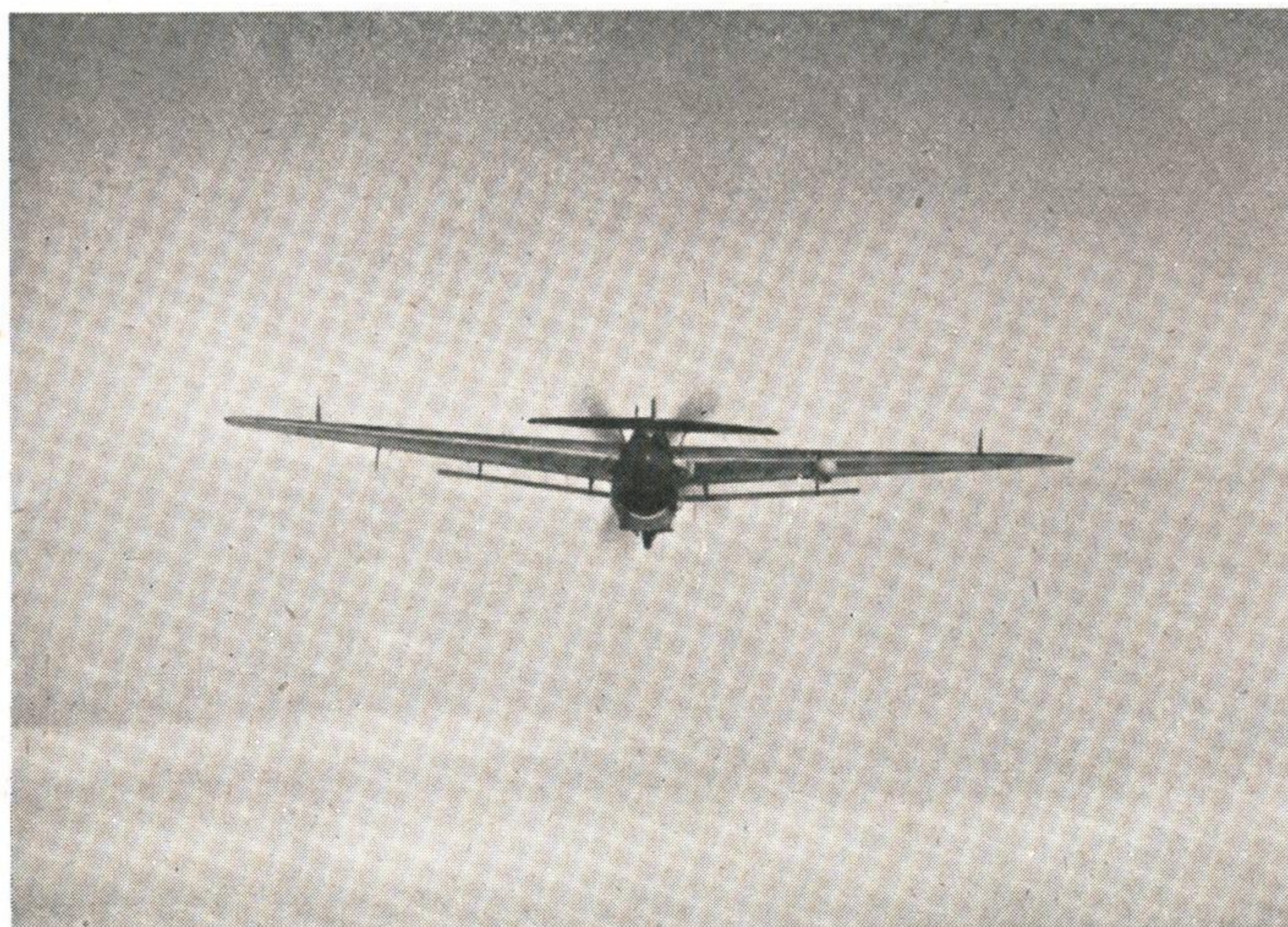
Dark Shark , or Ryan XF2R-1, for research on airscrew-turbine and jet-turbine combination for U.S. Navy. Tests are not yet complete. Prop-turbine is G.E. XT-31, turbojet is G.E. J-31.
