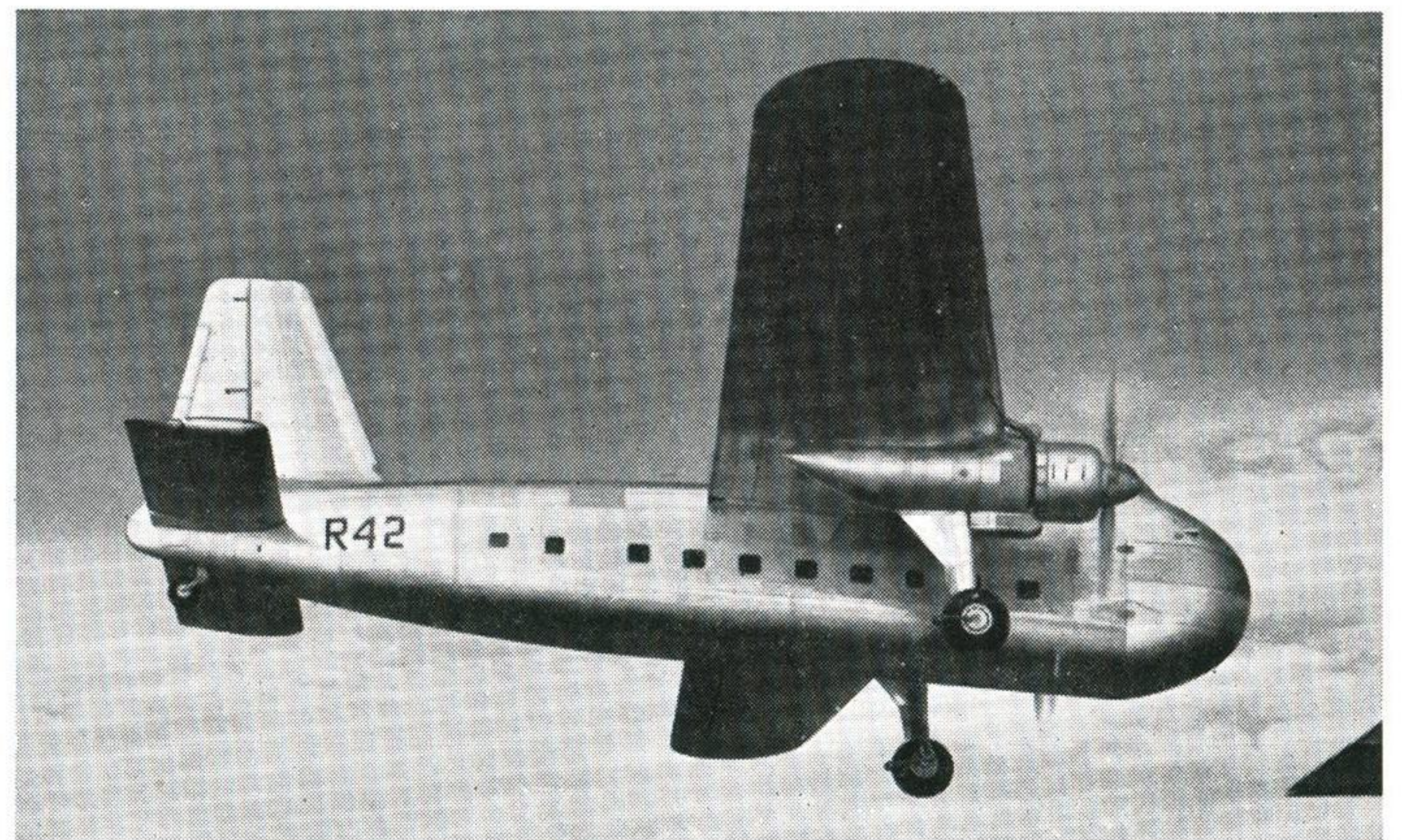
The Bristol 170 Wayfarer with extended and rounded wingtips.
