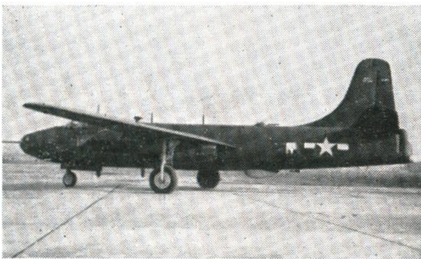
Main characteristics of the Martin XP4M-1 are: wide span narrow chord wing, blunt wing and tail surface tips, high fin and rudder with small fin fairing. The lower intakes behind engines retract. Top speed 398 m.p.h.
