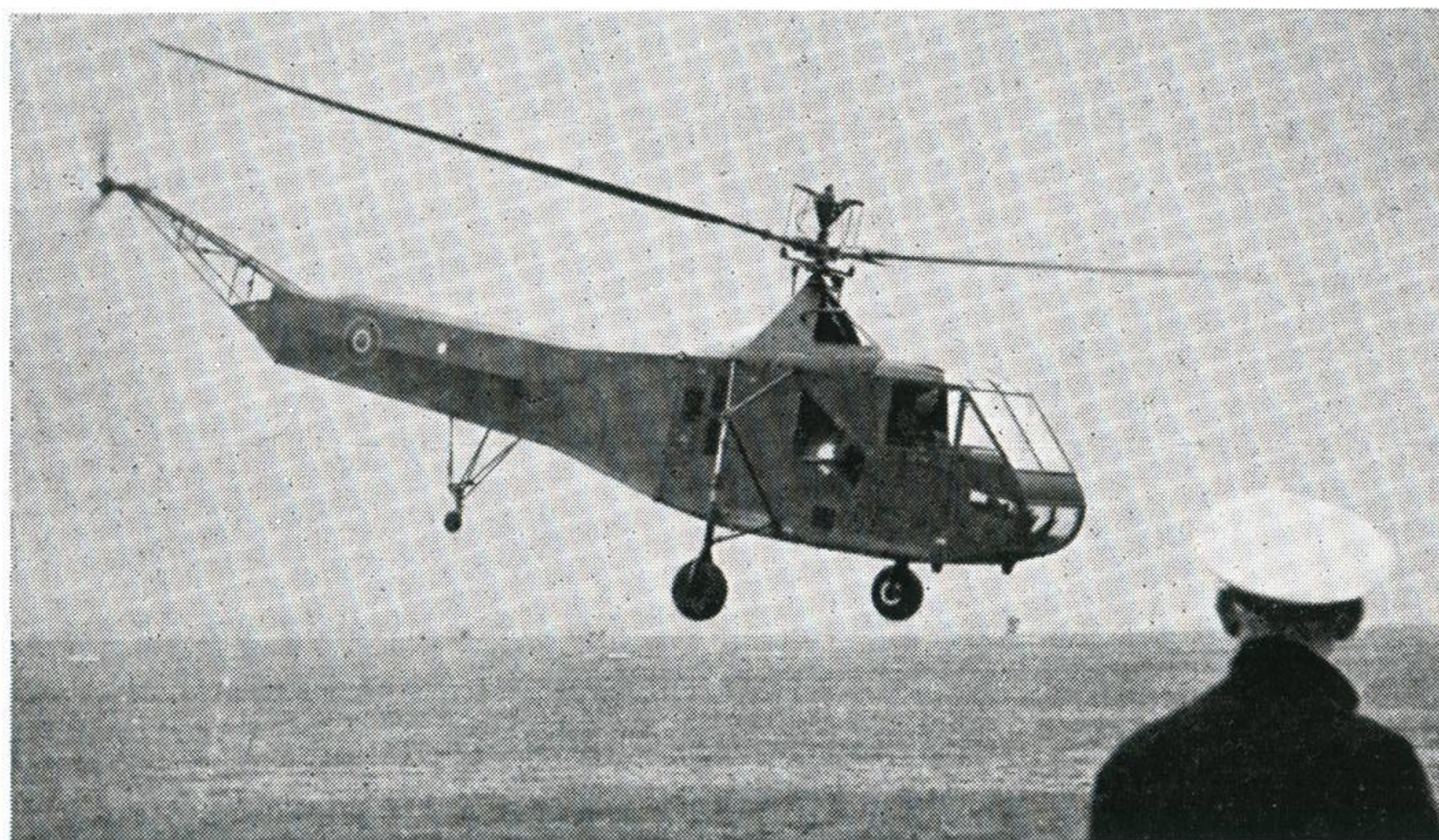
(Above) Forward Lifting : The Sikorsky Hoverfly I is in service with the Royal Navy and R.A.F. This one is dipping its nose as it moves forward. The coarser pitch of the rotor blades as they cross the tail-rotor-boom produces some extra lift at the rear, thus canting the Helicopter on its nose and moving it forward. (Rotor diameter 38 ft.)
