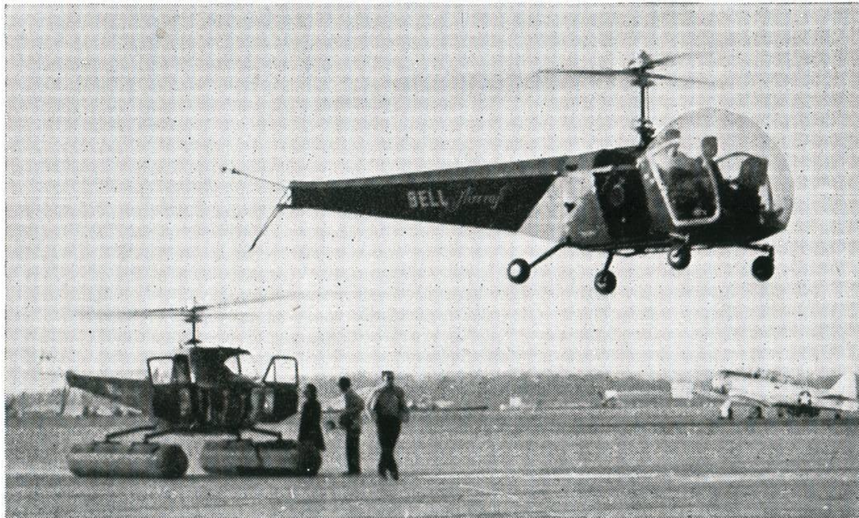
Bubble Nose : In production for the U.S.A.A.F. is the Bell YR-13 helicopter ex Bell 47. This single rotor type with torque-balancing tail-rotor, has only two blades to its main rotor. The blades though "non flapping" are universally mounted and can thus "see-saw", and produce the same result. The gadget rotating beneath the rotor is the stabilizing bar—a device for damping vibrations in the rotor. (Rotor diameter 33 ft. 6 in.)
