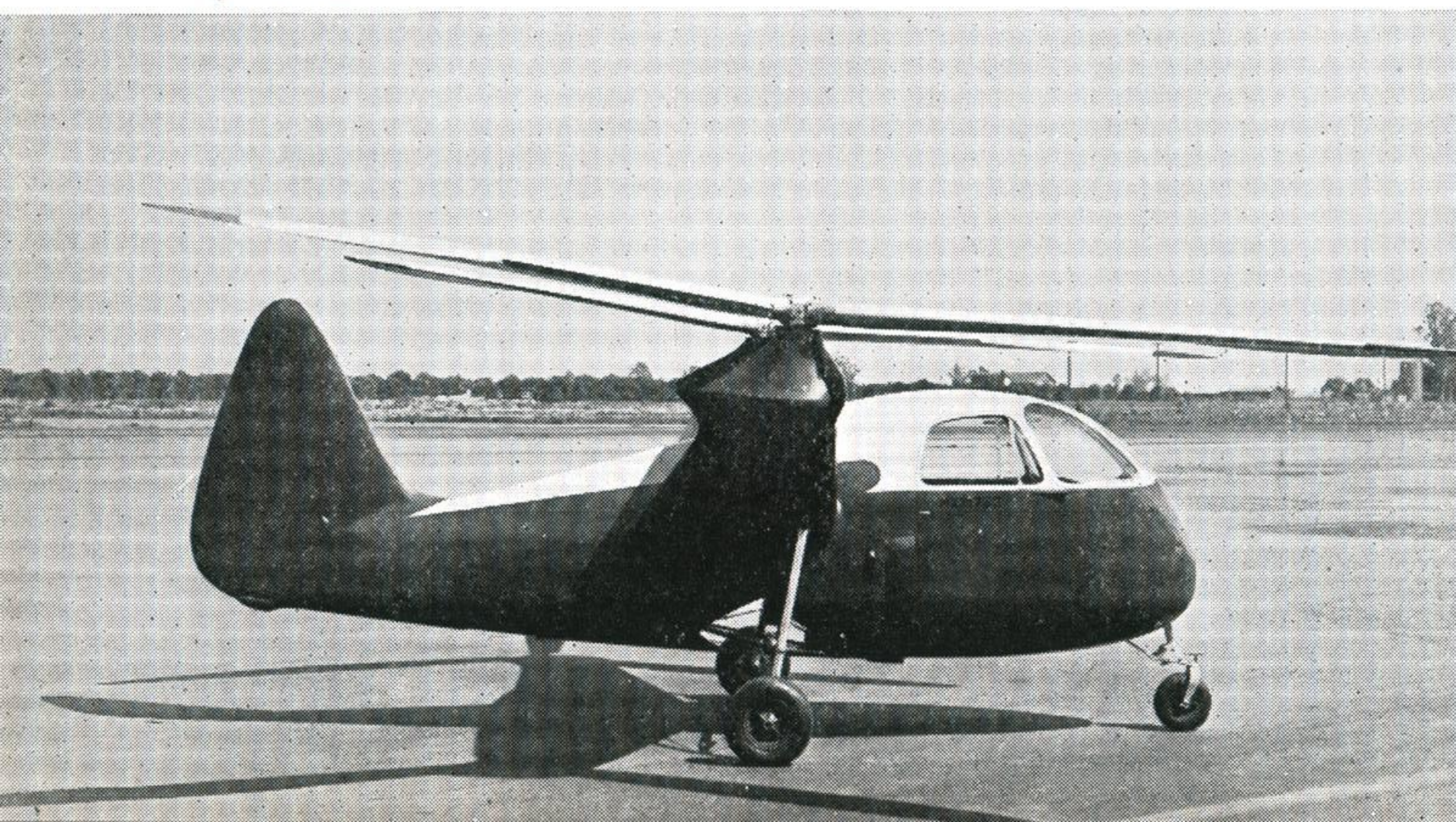
(Below) A neat little single-seat helicopter. The Landgraph H-2 has two side-by-side synchronized inter-meshing rotors. Interesting points: blade pitch is fixed, but ailerons are fitted to blades for control; it has a retractable undercarriage. (Rotor system span 27 ft.)
