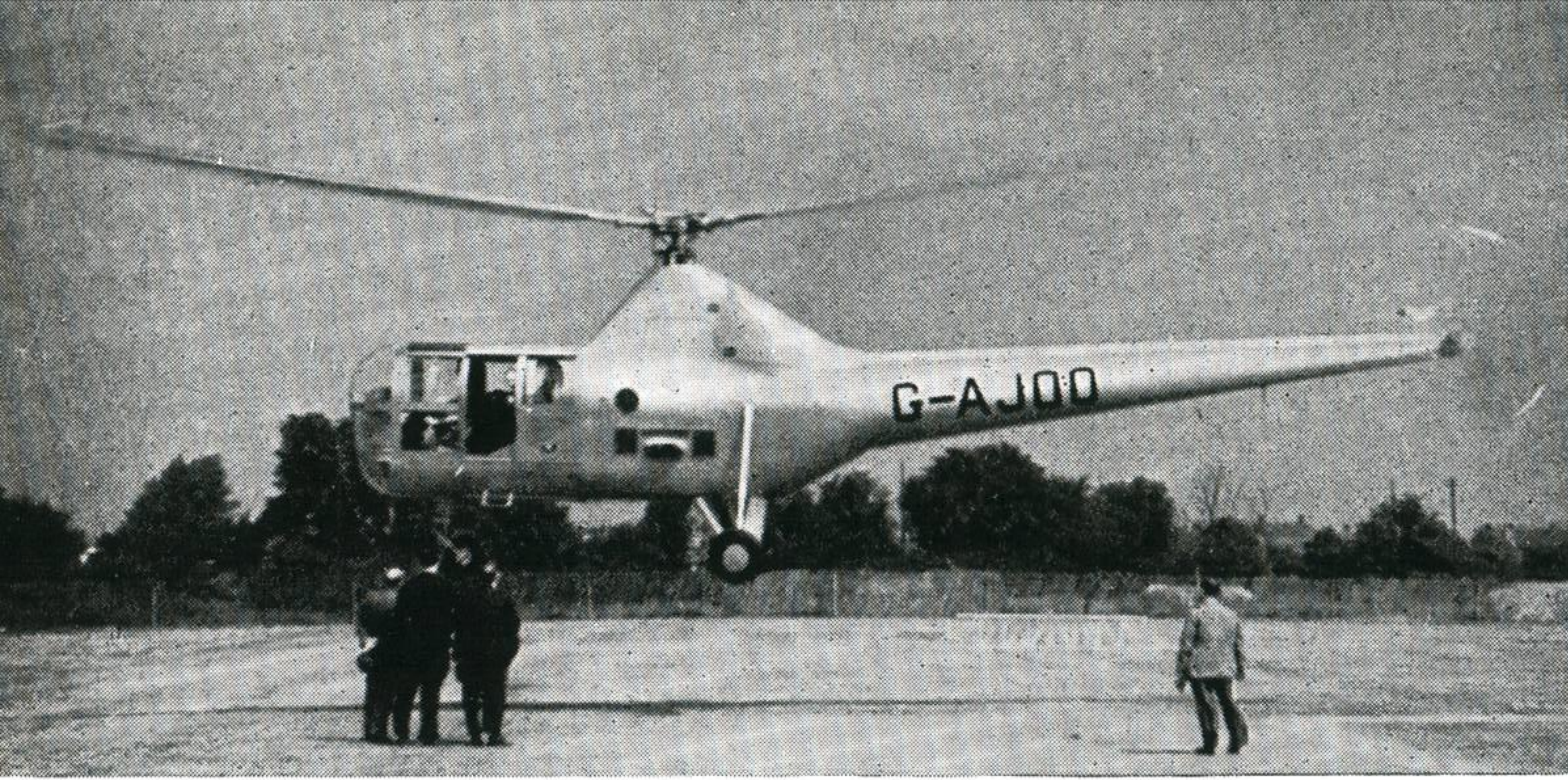
Coning Angle : A Sikorsky S-51 hovering. The down draught from the main rotor causes a "flap" amongst the spectators. This type of helicopter is to be built in Great Britain by Westland Aircraft. The engine in this particular model is the Pratt and Whitney Wasp Junior Radial. The Westland-Sikorsky S-51 will have the Alvis Leonides radial engine of 500 h.p. (Rotor diameter 48 ft.)
