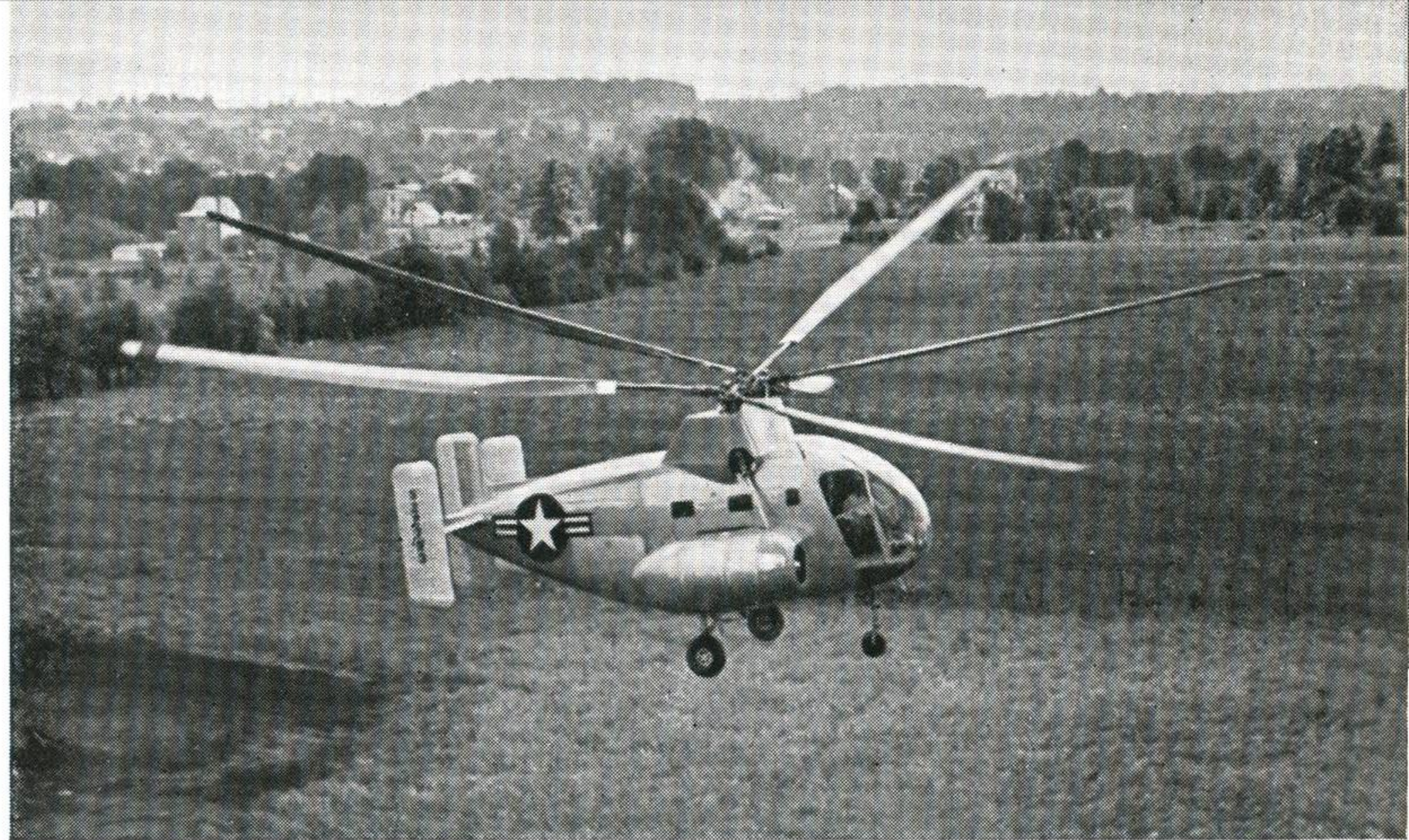
The Kellett XR-10, twin-engine transport helicopter, can carry up to ten passengers. Its cruising speed is 90 m.p.h. straight and level, and it has a range of 350 miles. The radial motors are in nacelles—one each side of the fuselage—they look very much like jet units, but are not. Rotors are synchronised and closely intermeshed—uncomfortably so, it might appear from this picture. (Rotor system span 65 ft.)
