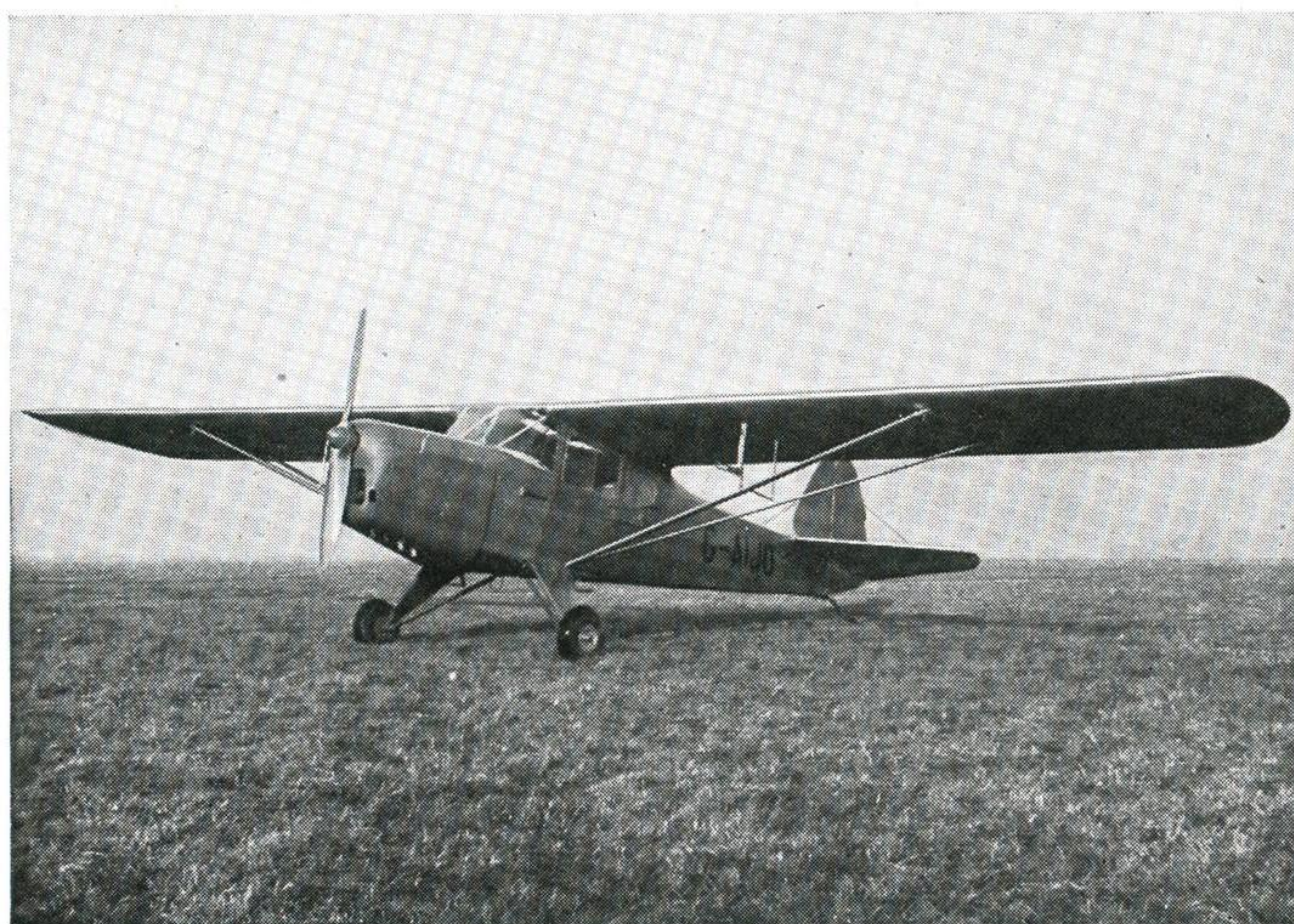
The Youngest. Very similar to the rest of its family is the new 2-seater Auster J/4 (190 h.p. Blackburn Cirrus). Designed for use as a club machine, the J/4 has dual control and side-by-side seating. Its maximum speed is 108 m.p.h., it cruises at 90 m.p.h., and stalls at 37 m.p.h.
