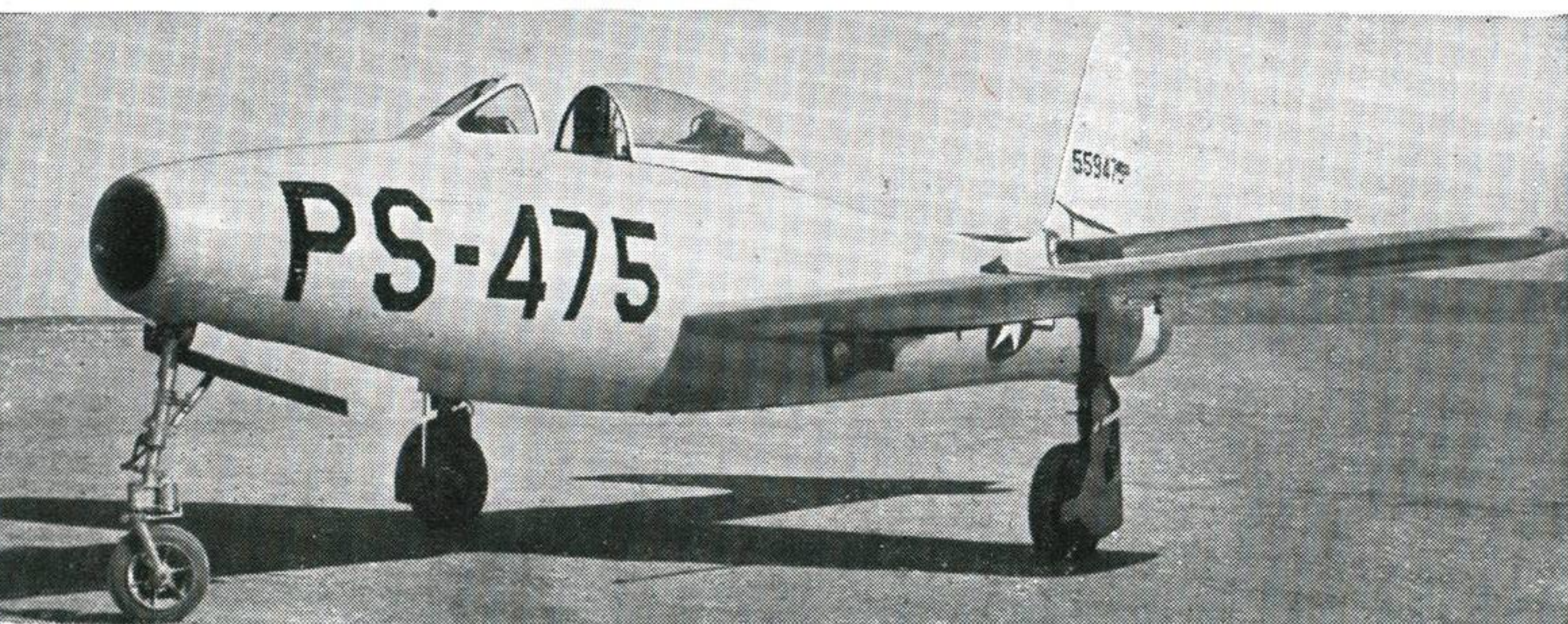
(below) This USAAF picture taken at Muroc of the Republic XP-84 Thunderjet high speed record hope of the USAAF indicates that the machine has a bottle shaped body form. At present it is being groomed for another record attempt. The P-84 is in production for the USAAF. (Span 36 ft. 5 ins.)
