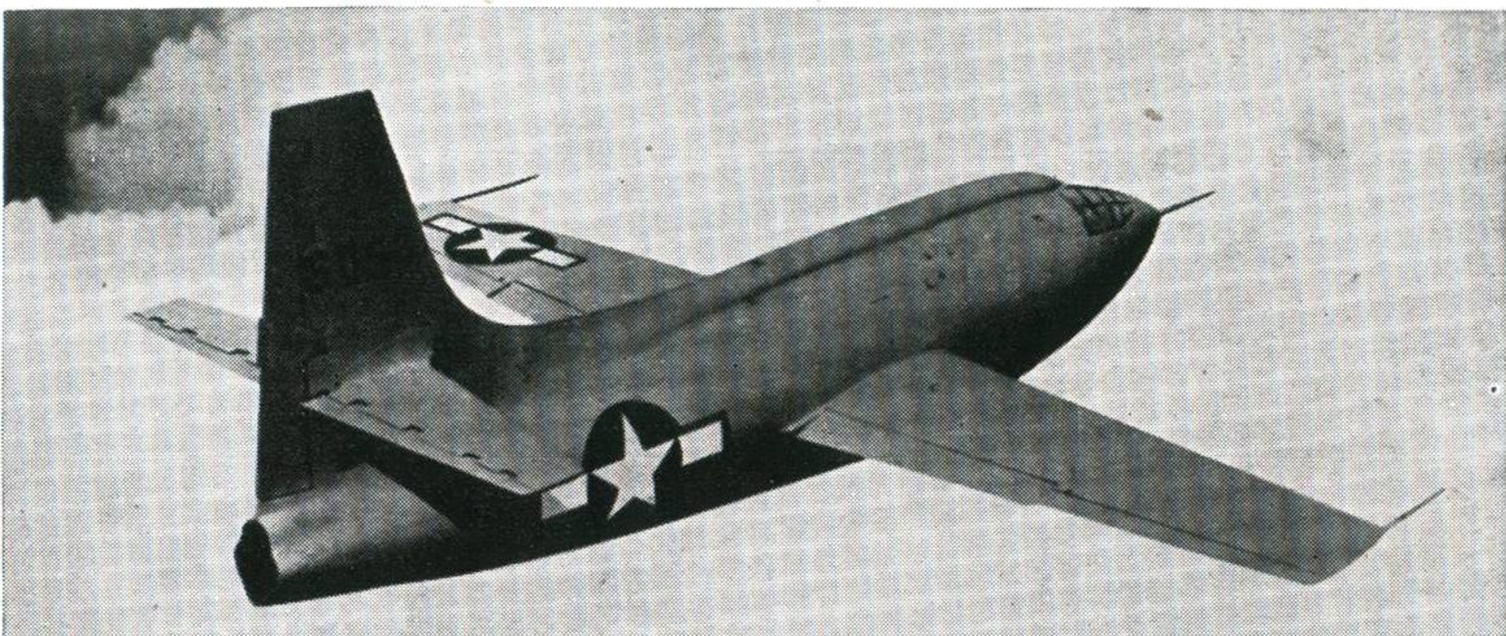
A USAAF photo of the Bell XS-1 supersonic aircraft designed for speeds up to 1,700 m.p.h. Its rocket motor, based upon a German design, lasts only from three to four minutes so the XS-1 has to be taken to its operating altitude by Superfortress and released. Some trial flights have been made at very high speeds—not supersonic—as yet. (Span 38 ft. 1 in.)
