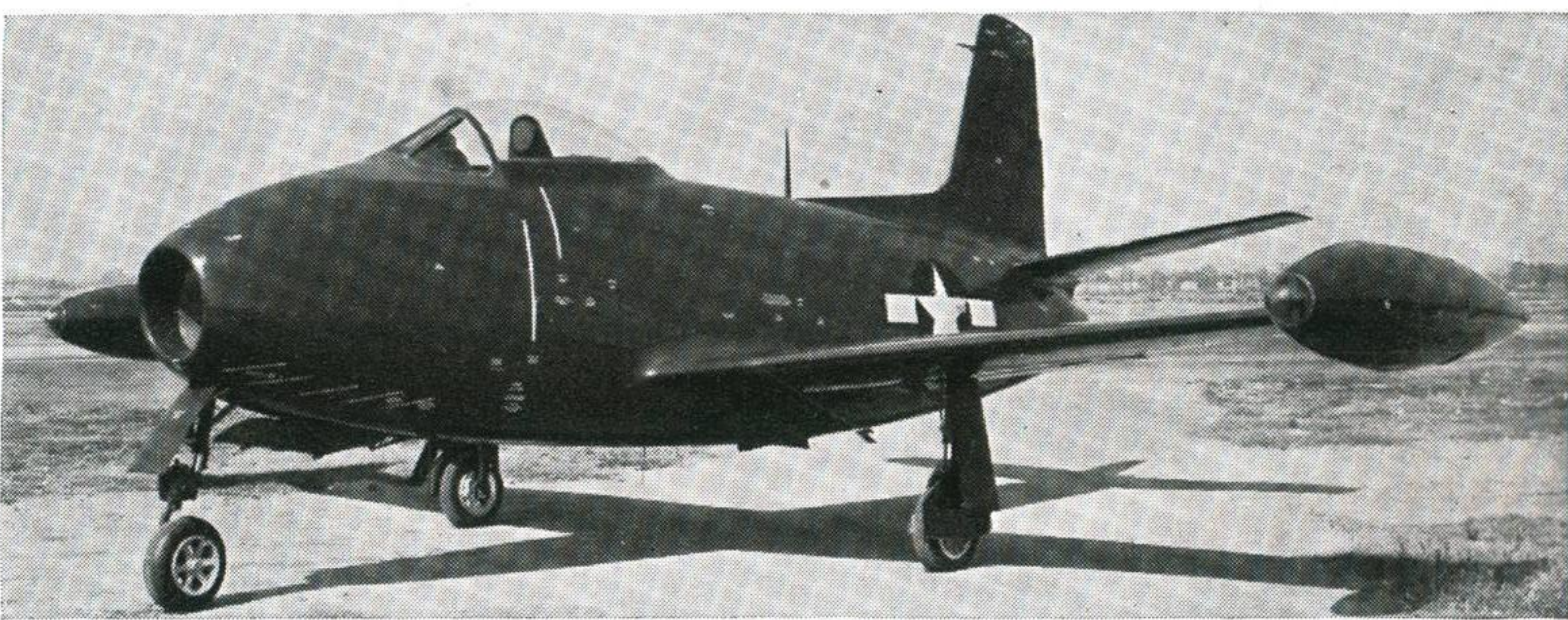
(above) North American XFJ-1 jet-propelled U.S. Navy fighter, known also to the USAAF as the XP-86, is about to be tested. Fashionable wing-tip tanks do not appear "droppable" as navigation lights are fitted to them.
