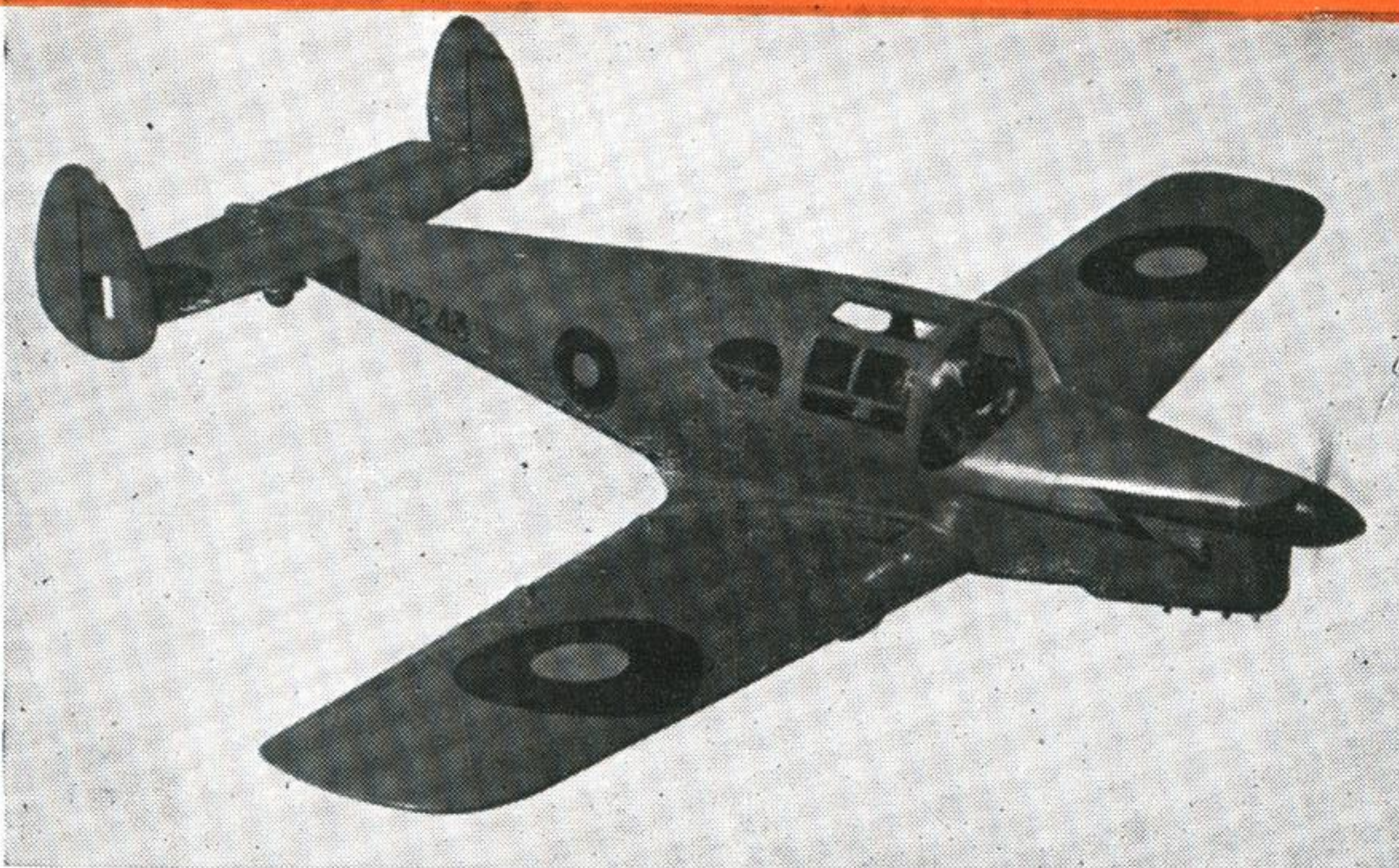
At least four Miles M-28 variants have been built. Differences are mainly internal and this shot covers them all recognitionally. A four seat, light transport, of obvious Miles origin, it is powered by a D.H. Gipsy Major. (Span 30 ft. 8 ins.)
