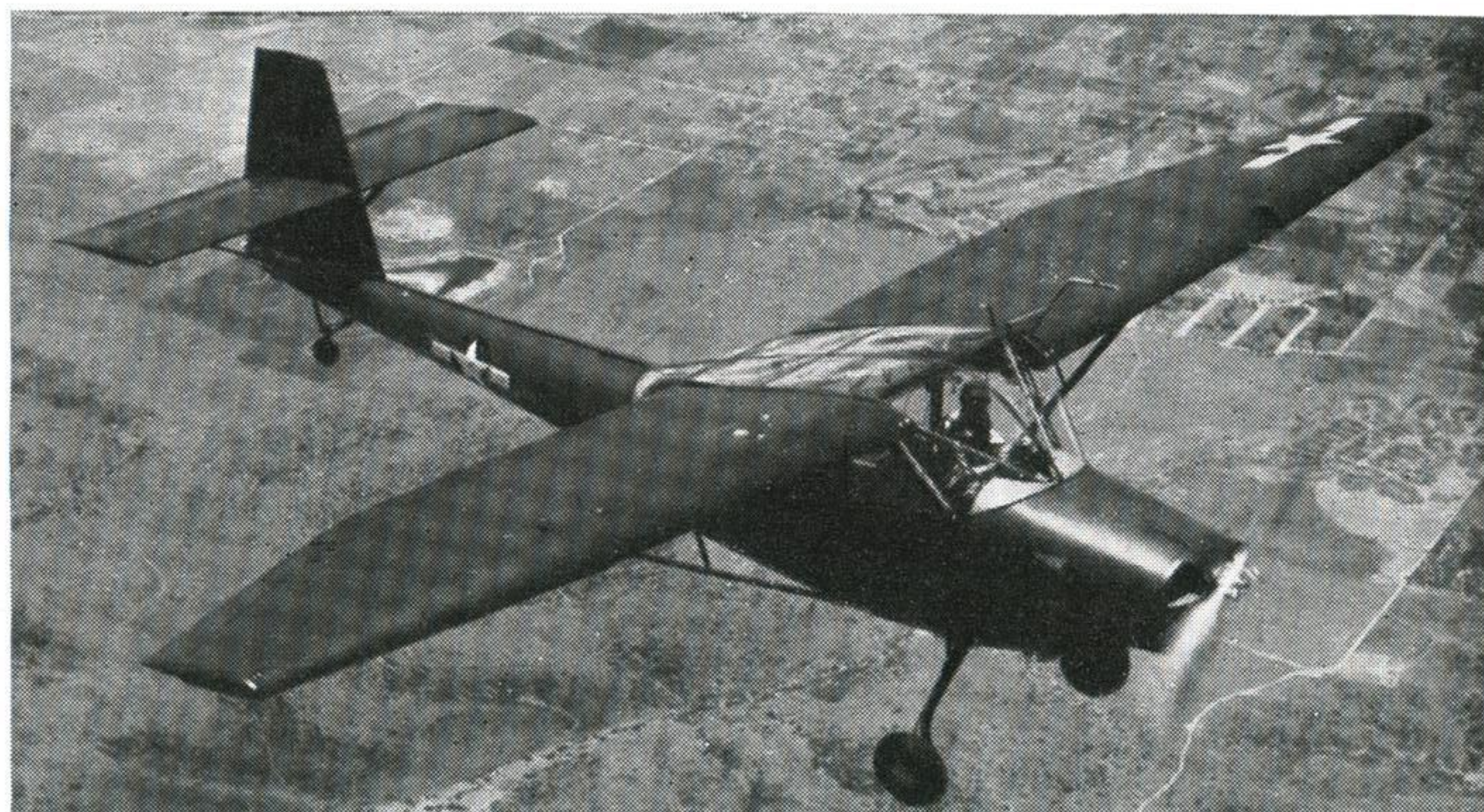
The XBT2C-1, alias Experimental Bomber-Torpedo second design by Curtiss, first one built, conforms to the pattern of its class, deep fuselage, blunt nose, (Wright Cyclone), high tail (see Helldiver) and squared off wing tips.
