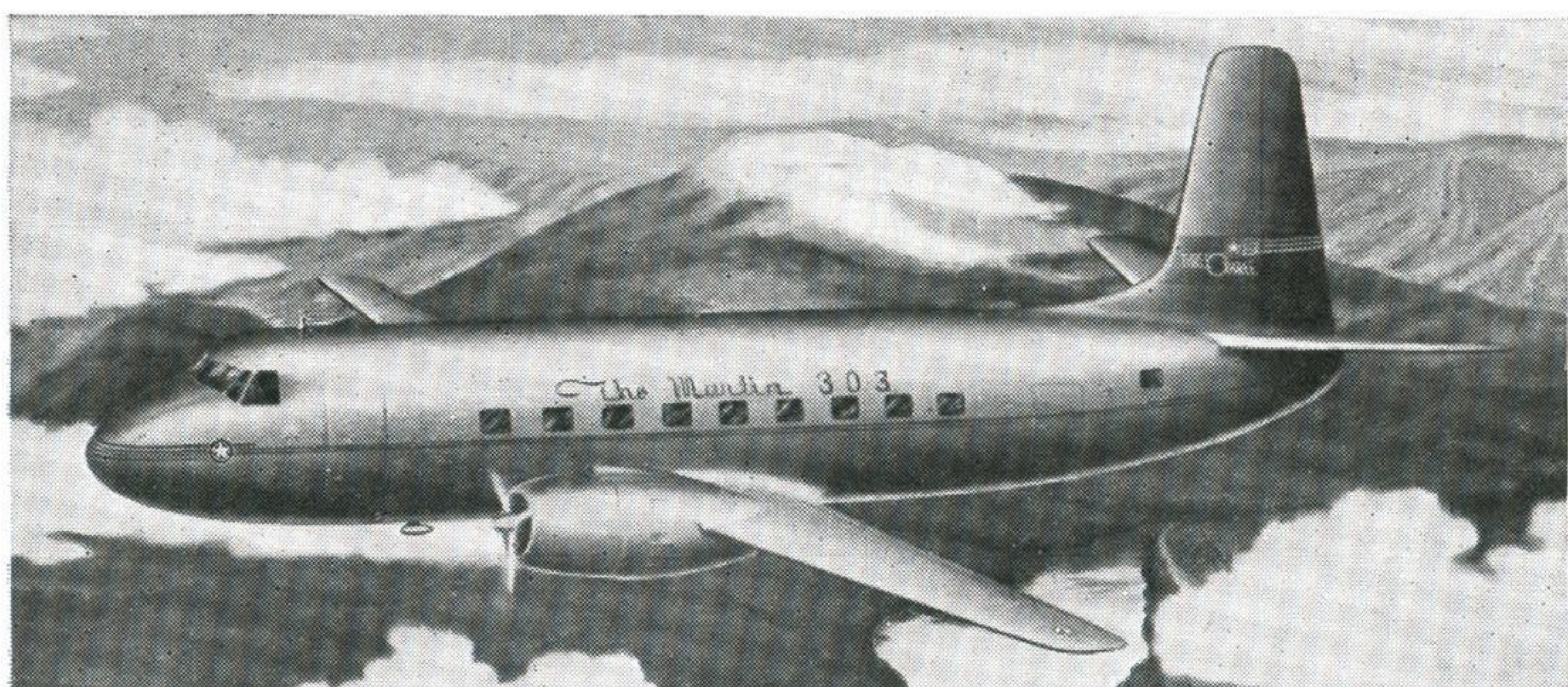
An impression of the Martin 3-0-3 built for internal airline work. K.L.M. have ordered some. Pratt and Whitney Radials will have "jetted" exhausts to augment thrust. (Span 89 ft. 4 ins.)
