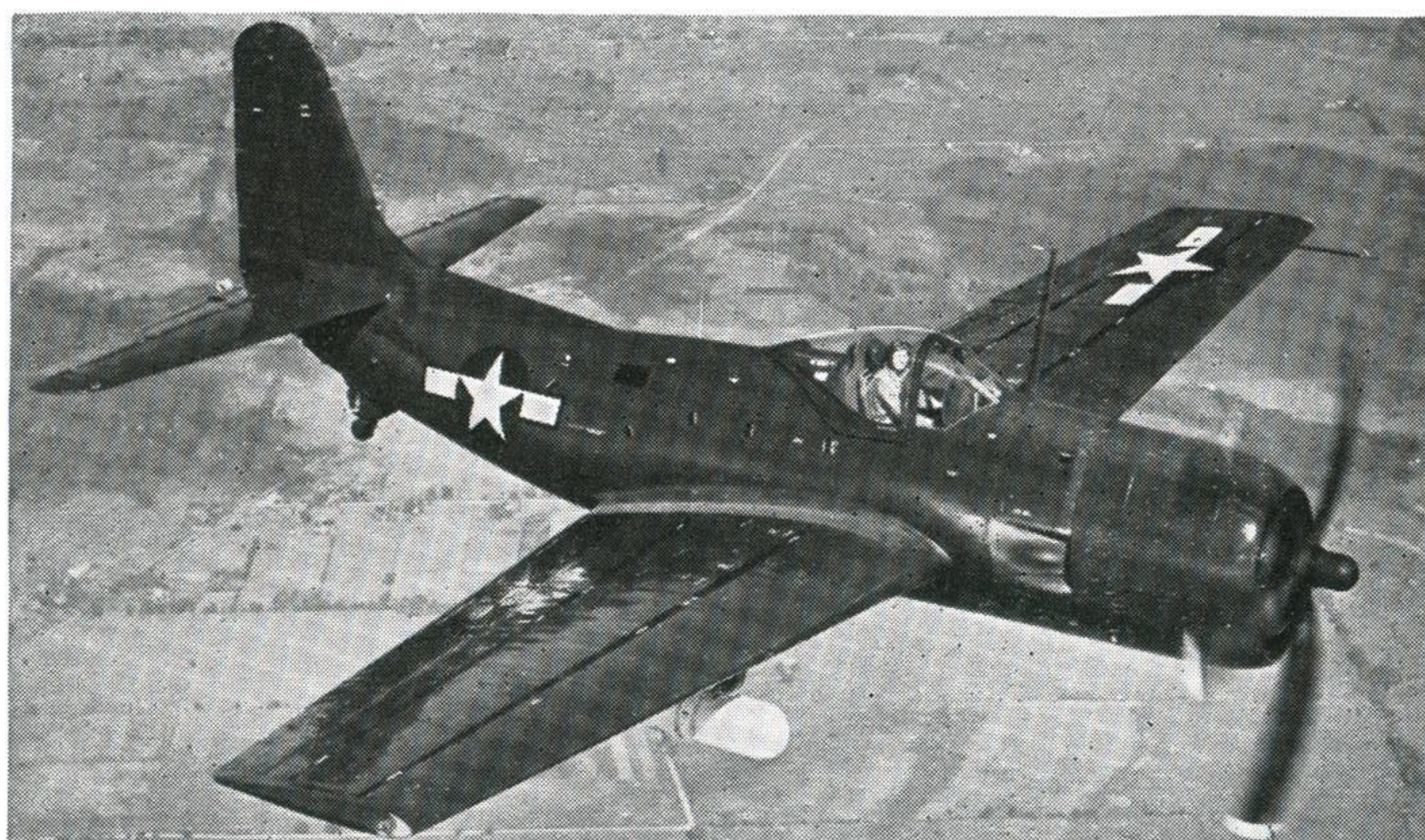
The XBT2C-1, alias Experimental Bomber-Torpedo second design by Curtiss, first one built, conforms to the pattern of its class, deep fuselage, blunt nose, (Wright Cyclone), high tail (see Helldiver) and squared off wing tips.
