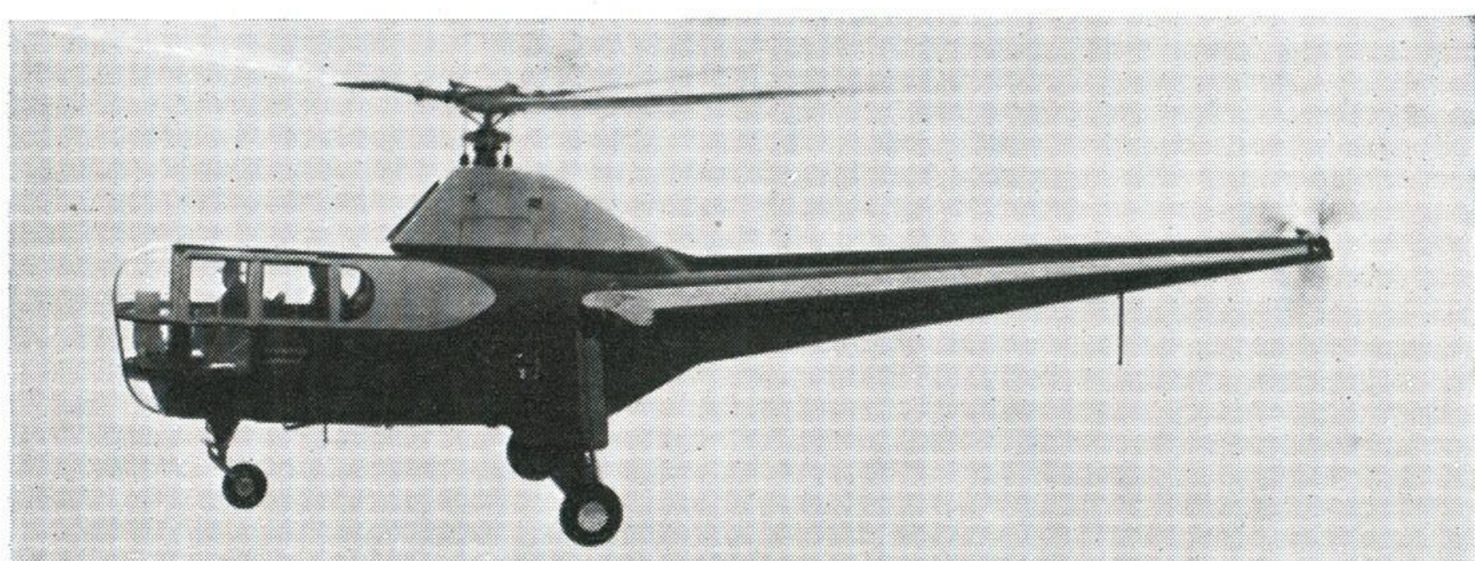
Already in regular service the Sikorsky S-51 4-seat helicopter is one of a large number of helicopters flying in America. The enclosing of its mechanism within fairings at least provides some tangible and recognizable structure forms so uncommon in helicopters. Other designers please note.
