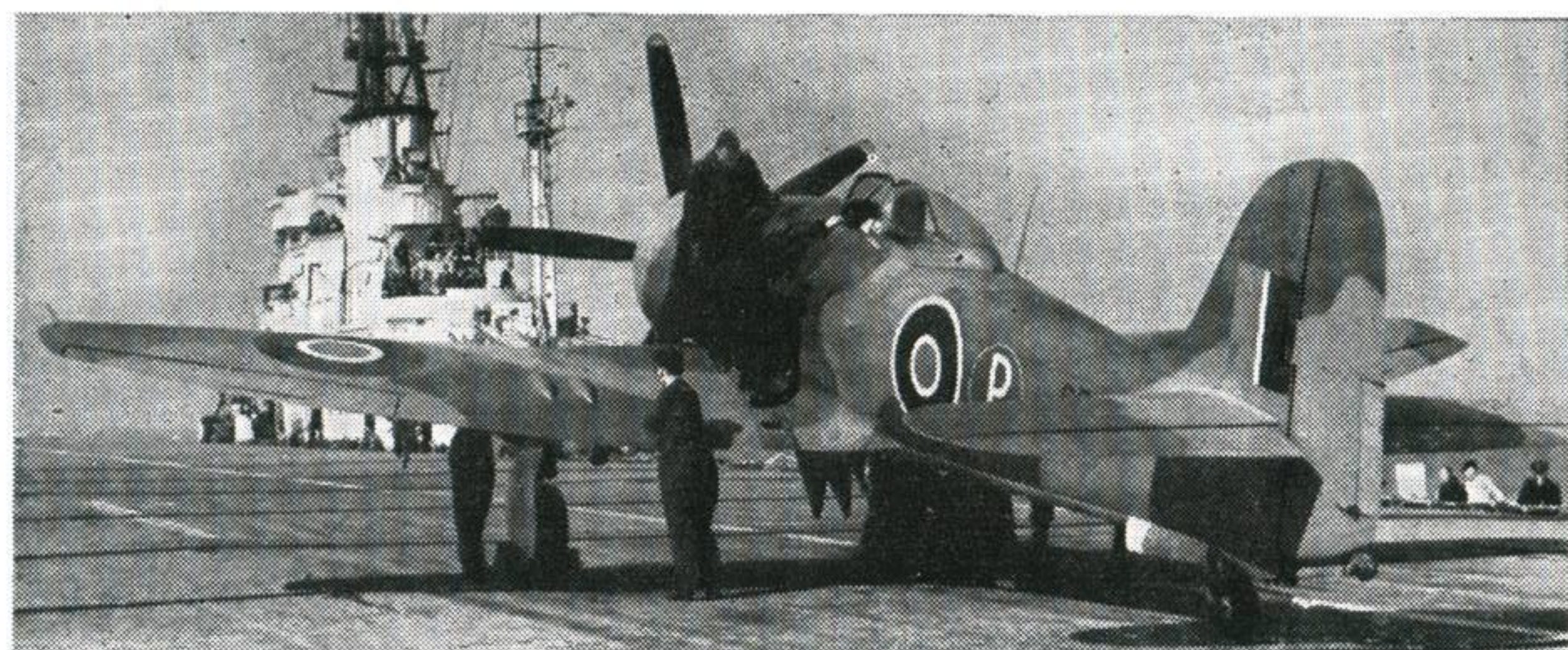
↑ "Hell knows no Fury like a Sea Fury X ". The Hawker Sea Fury X ranged on a carrier's deck. Note tail unit and arrester-hook details. (Span 38 ft. 5 ins.).
