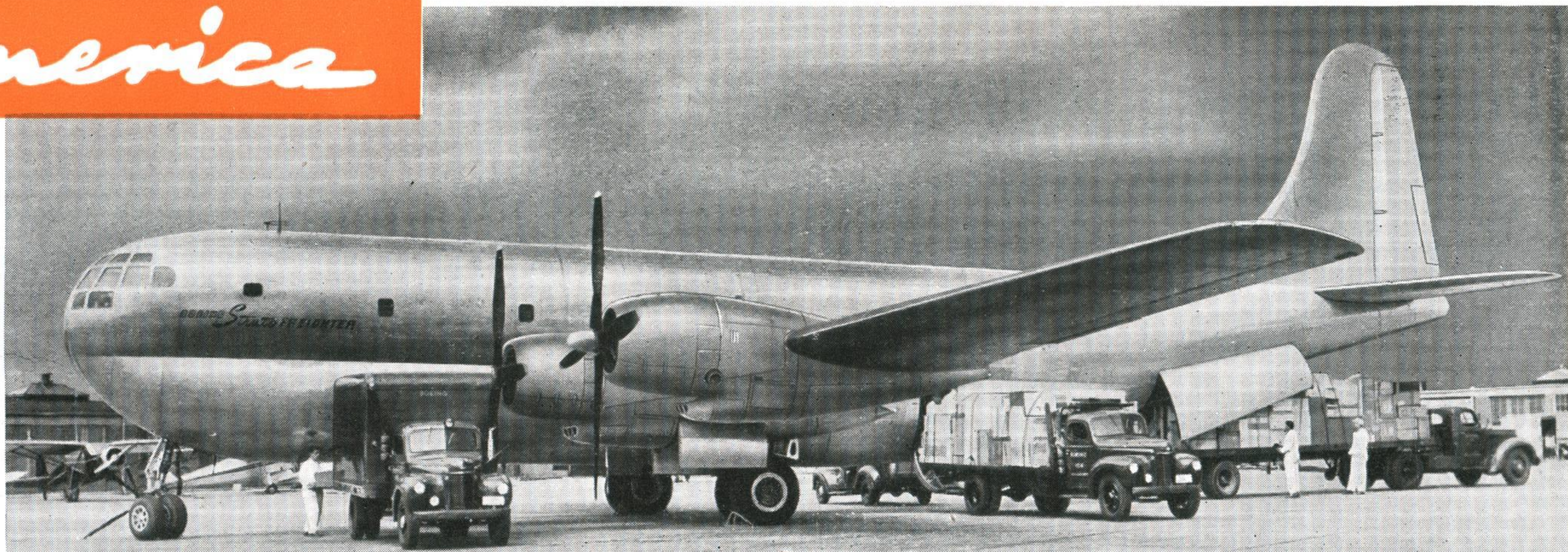
Boeing's big Stratofreighter cargo version of the Stratocruiser, has four Pratt and Whitney Wasp Major radials. The USAAF have a transport version, the C-97. Wings and tail unit are similar to those of the Superfortress. (Span 141 ft. 3 in.)
