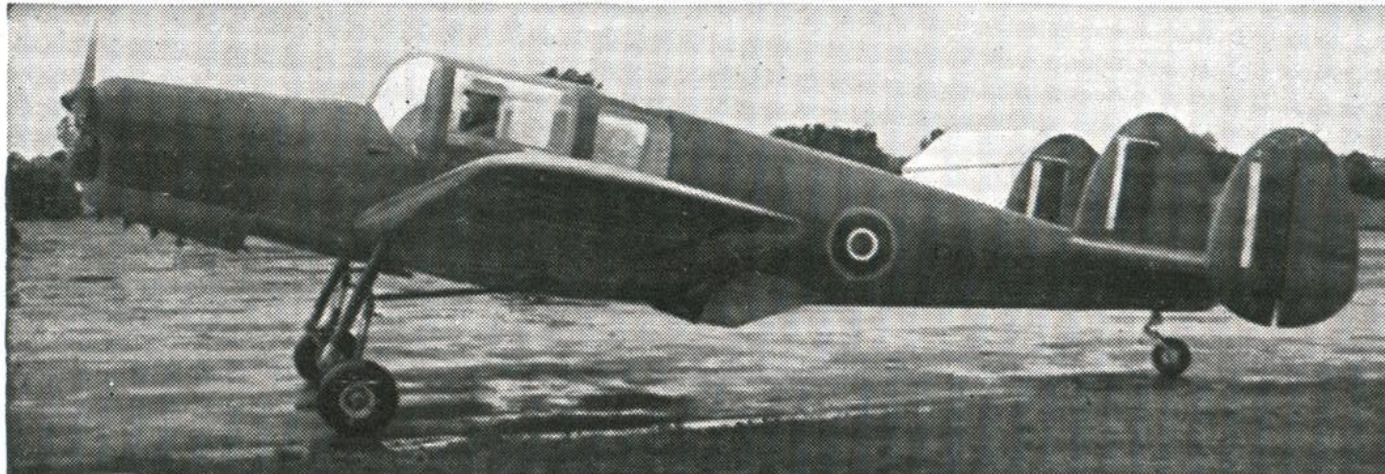
Fin Formation —A Miles Messenger on Communication Duties—and another gift to the brotherhood of spotters. That is, provided you can see the three fins, or the flaps, or the fixed undercarriage which, together with the "Miles" appearance, all add up to the Messenger. With 3 or 4 people aboard, its Blackburn Cirrus III engine gives a top speed of 135 m.p.h.—range is 460 miles. (Span 36 ft. 2 in.)
