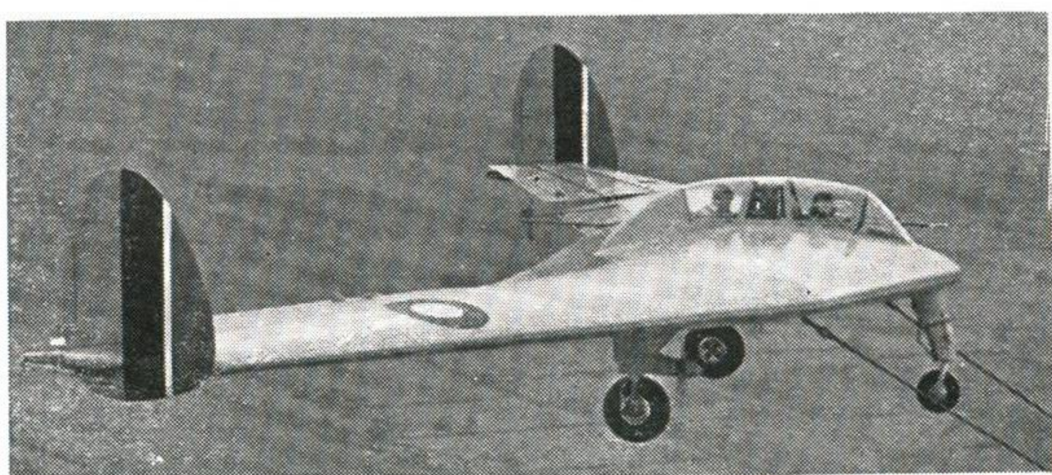
Above is the Armstrong Whitworth A.W.52G experimental glider, which is in the "flying wing" class. By dispensing with the fuselage and tail unit, both weight and drag are reduced. The small propellers on the undercarriage legs drive generators for providing power for the aircraft's electrical services.
