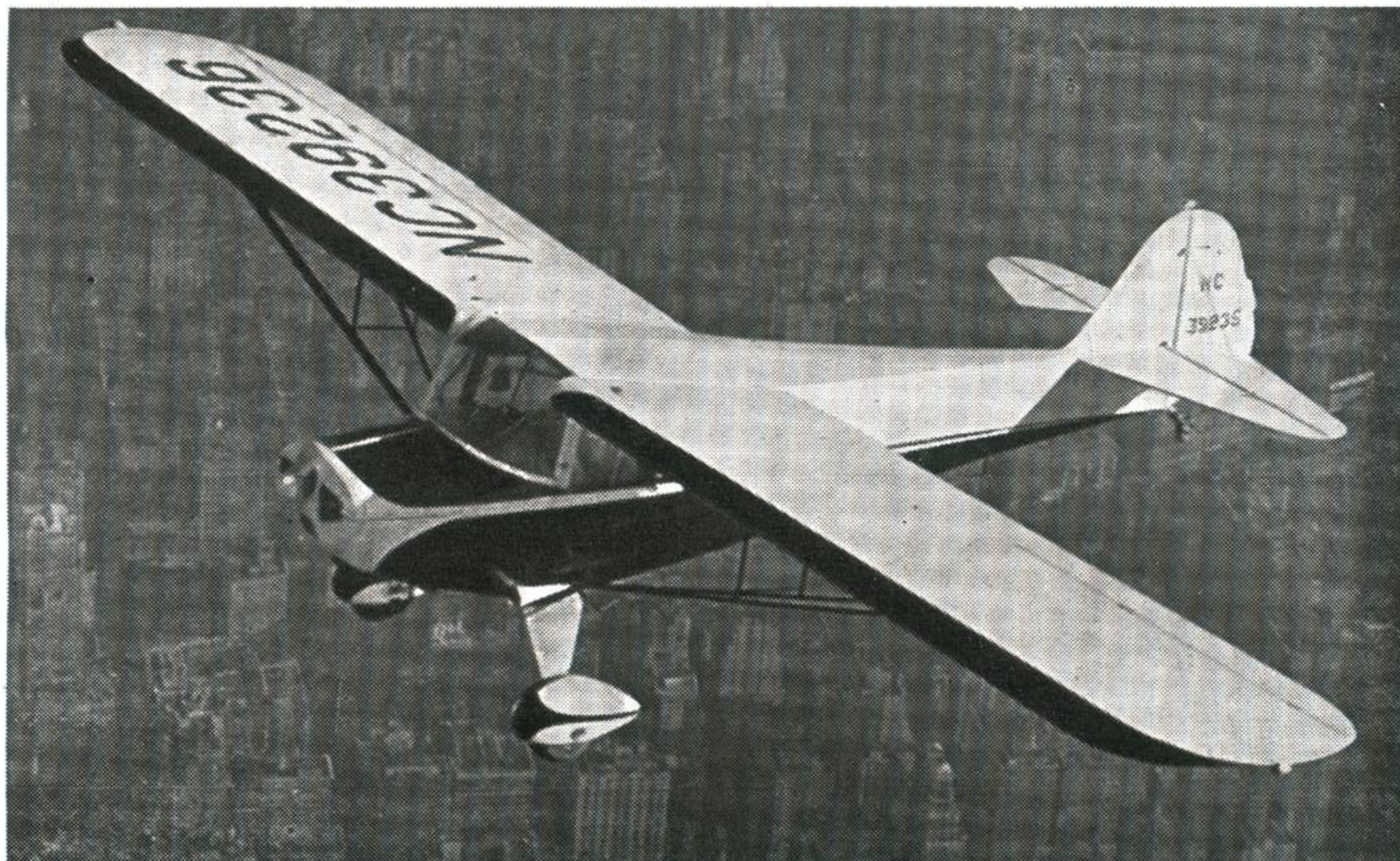
The American Way —The Taylorcraft BC 12D is blood brother to our own Auster, since the British Auster Aircraft firm was originally an offshoot of Taylorcraft of U.S.A. It is now "on its own". The American has a "solid" cabin roof, spats, and a 65 h.p. Continental engine; otherwise, the similarity of shapes and forms is obvious. The top speed of the 12D is 117 m.p.h. (Span 36 ft. 0 in.)
