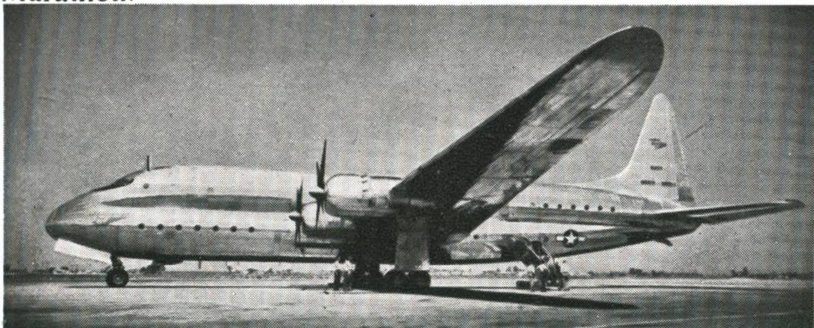
LOCKHEED CONSTITUTION. This 92-ton double decker aeroplane will take 180 passengers for 6,000 miles at 300 m.p.h. The total horsepower is 14,000 from 4 Pratt and Whitney Wasp Majors. Its highest peak, the fin-tip, is 52 ft. from the deck.
