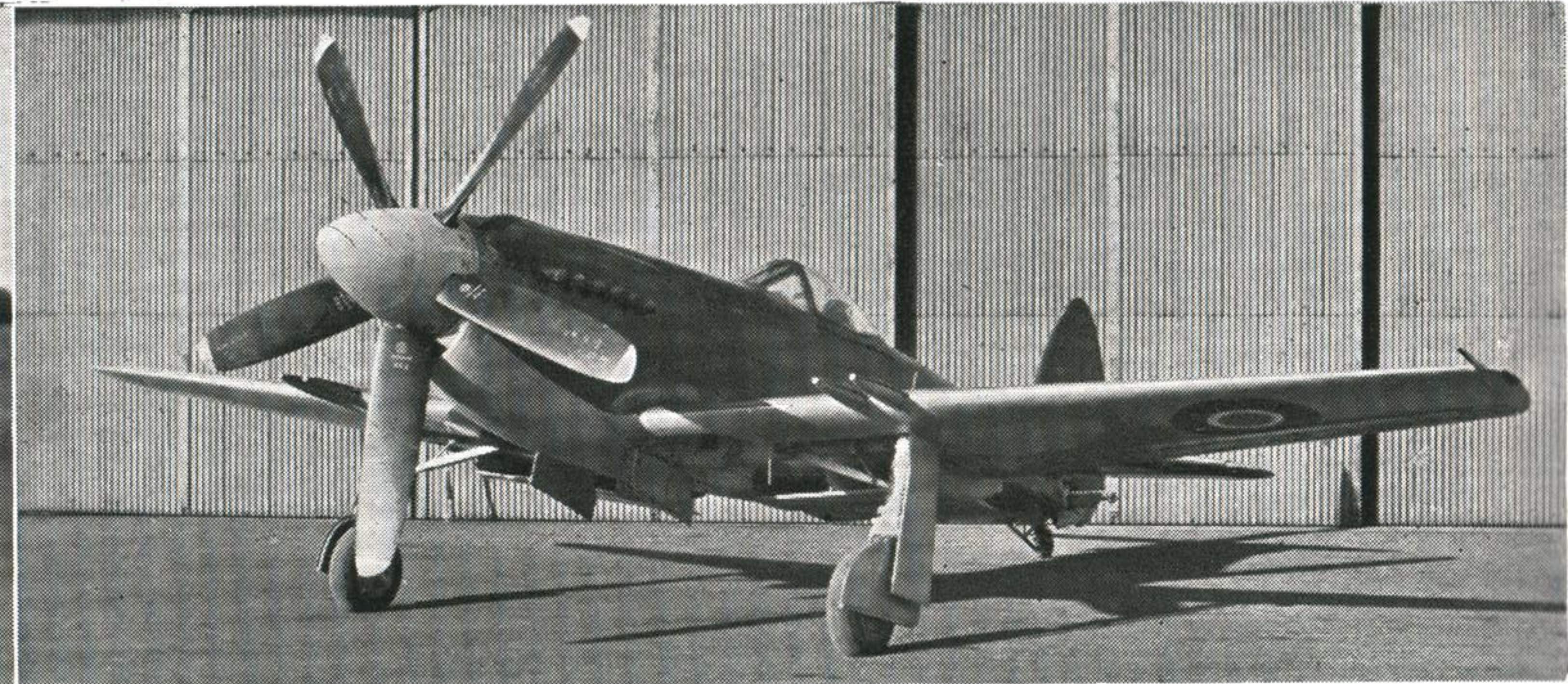
SUPERMARINE SEAFANG F.Mk.32 (Rolls Royce Griffon 69, 1,540 h.p.)—Differs from Seafires in its angular wing, shallow radiators, inward-retracting wheels, and larger tailplane.
