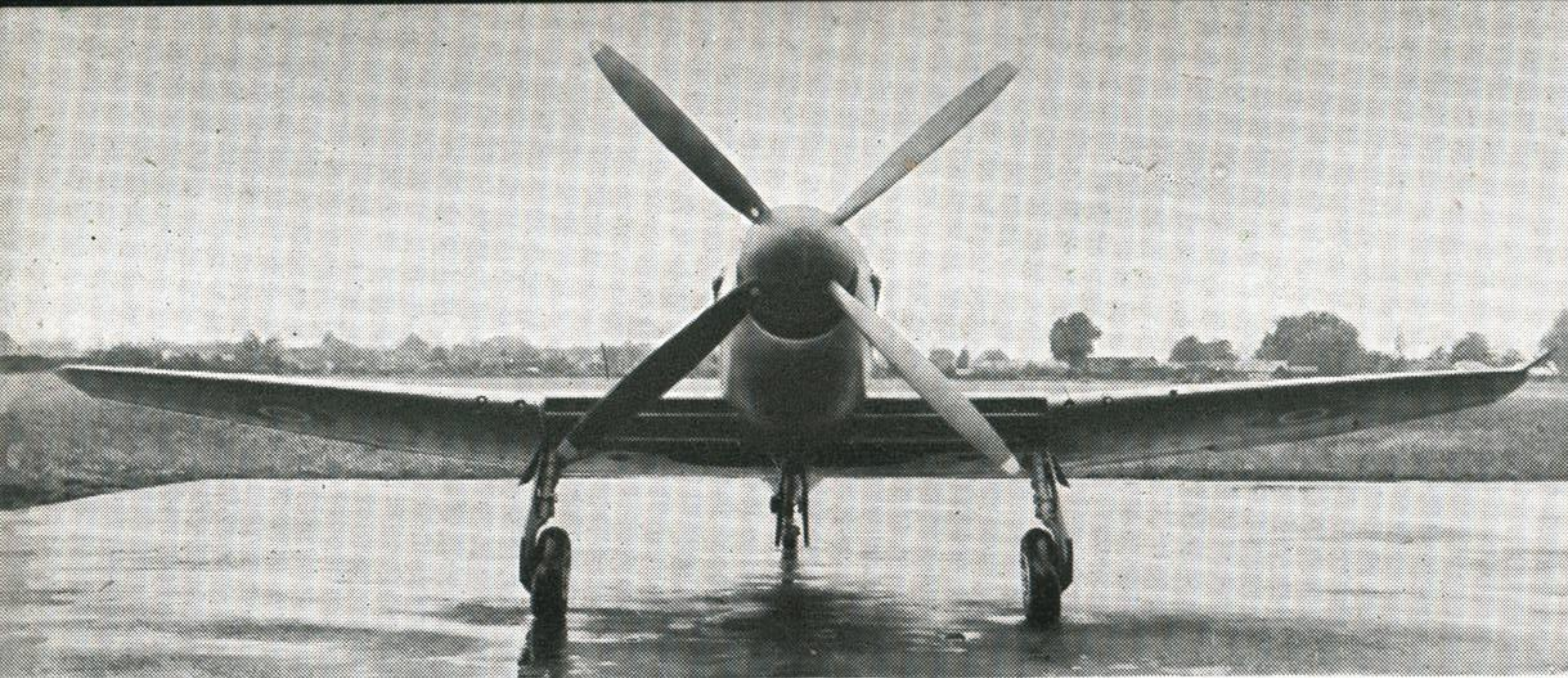
HAWKER FURY F.Mk.I (Napier Sabre VII, 3,000 h.p. plus)—Leading edge "slot" type radiators reduce frontal area and permit neater and closer engine cowling.
