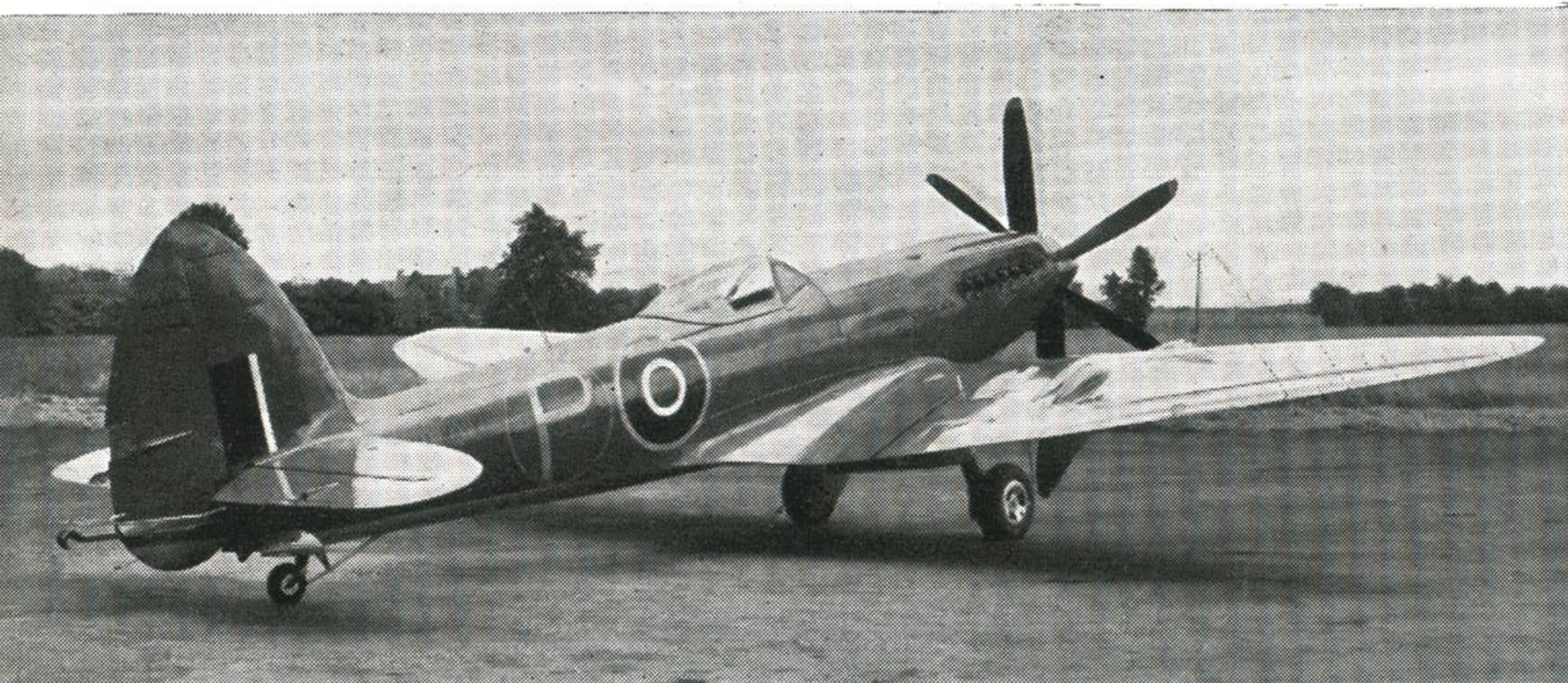
SUPERMARINE SEAFIRE F.Mk.47 (Rolls Royce Griffon 88, 2,050 h.p.)—Embodying lessons of Seafire 45 and 46, the wing fold is now outside the cannon.
