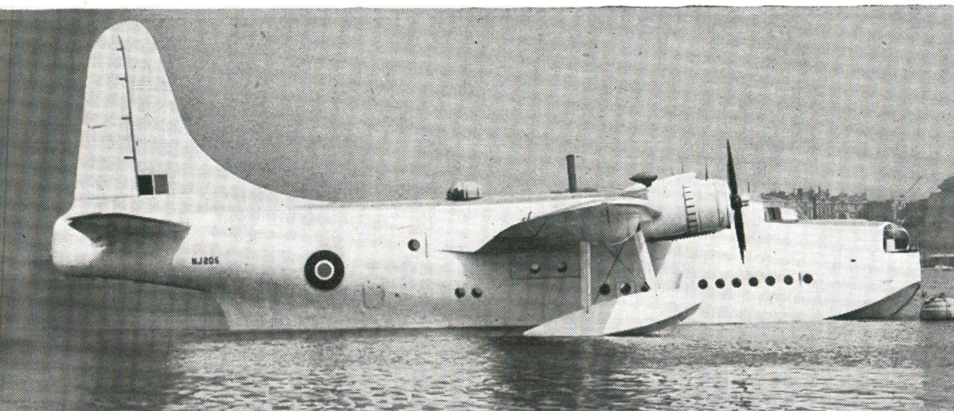
SHORT SEAFORD Mk.I (Bristol Hercules XVII, 1,740 h.p.)—Originally the Sunderland IV; has enlarged fin and rudder and a longer rear step, among other things. Civilianized, it is the Solent.
