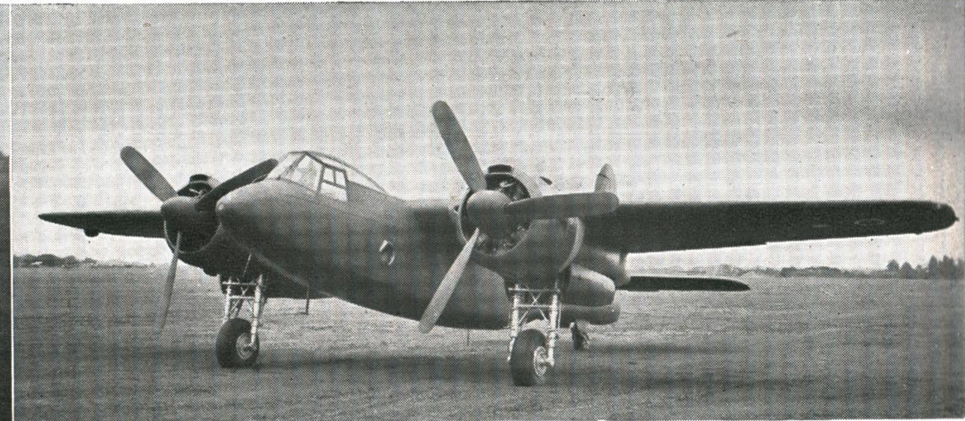
MILES MONITOR T.T. Mk. II (Wright Cyclones, 1,750 h.p.)—This mark of Monitor target tug for the Navy differs from the R.A.F.'s Mk. I in its naval equipment, dive brakes and a different cupola.
