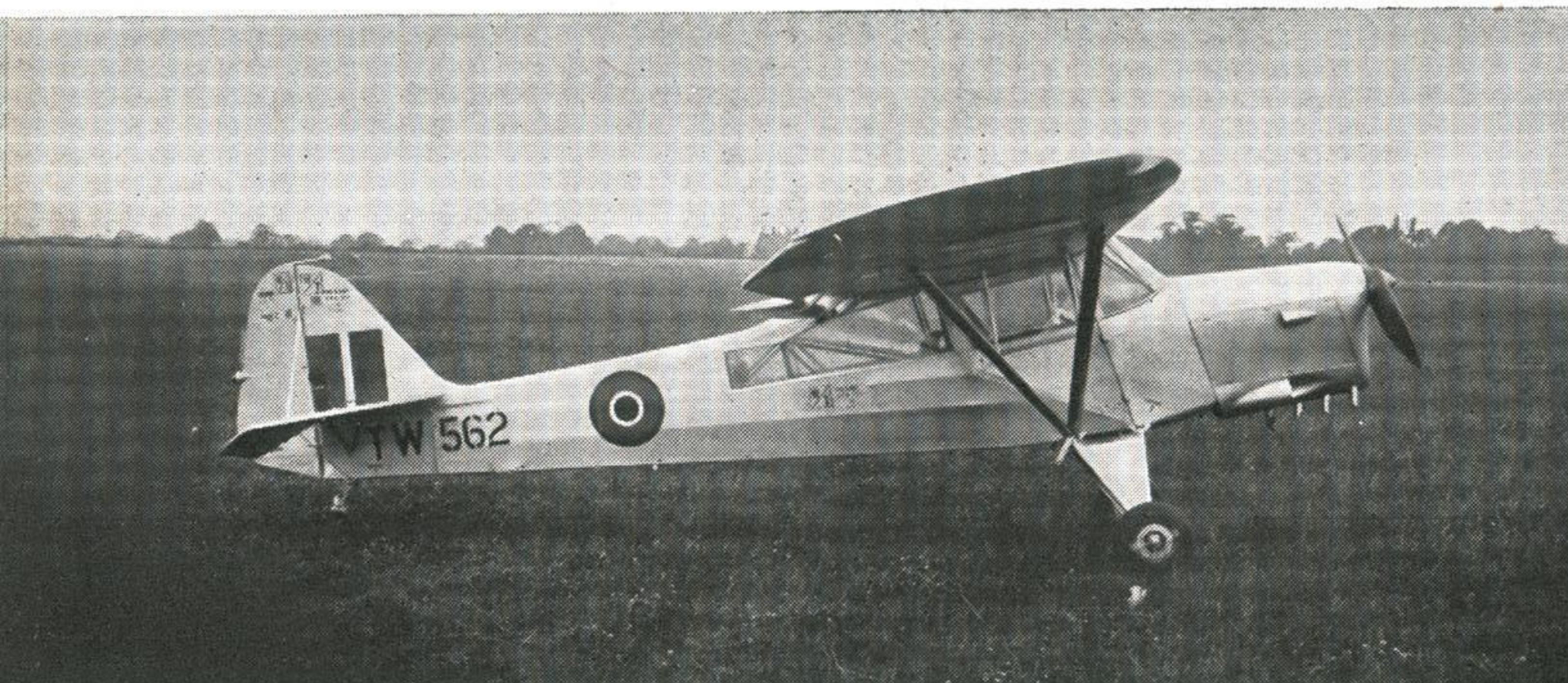
AUSTER Mk. VI (D.H. Gipsy Major VII, 142 h.p.)—A taller undercarriage, slightly revised cabin and large, projecting flaps distinguish this model of the Auster.
