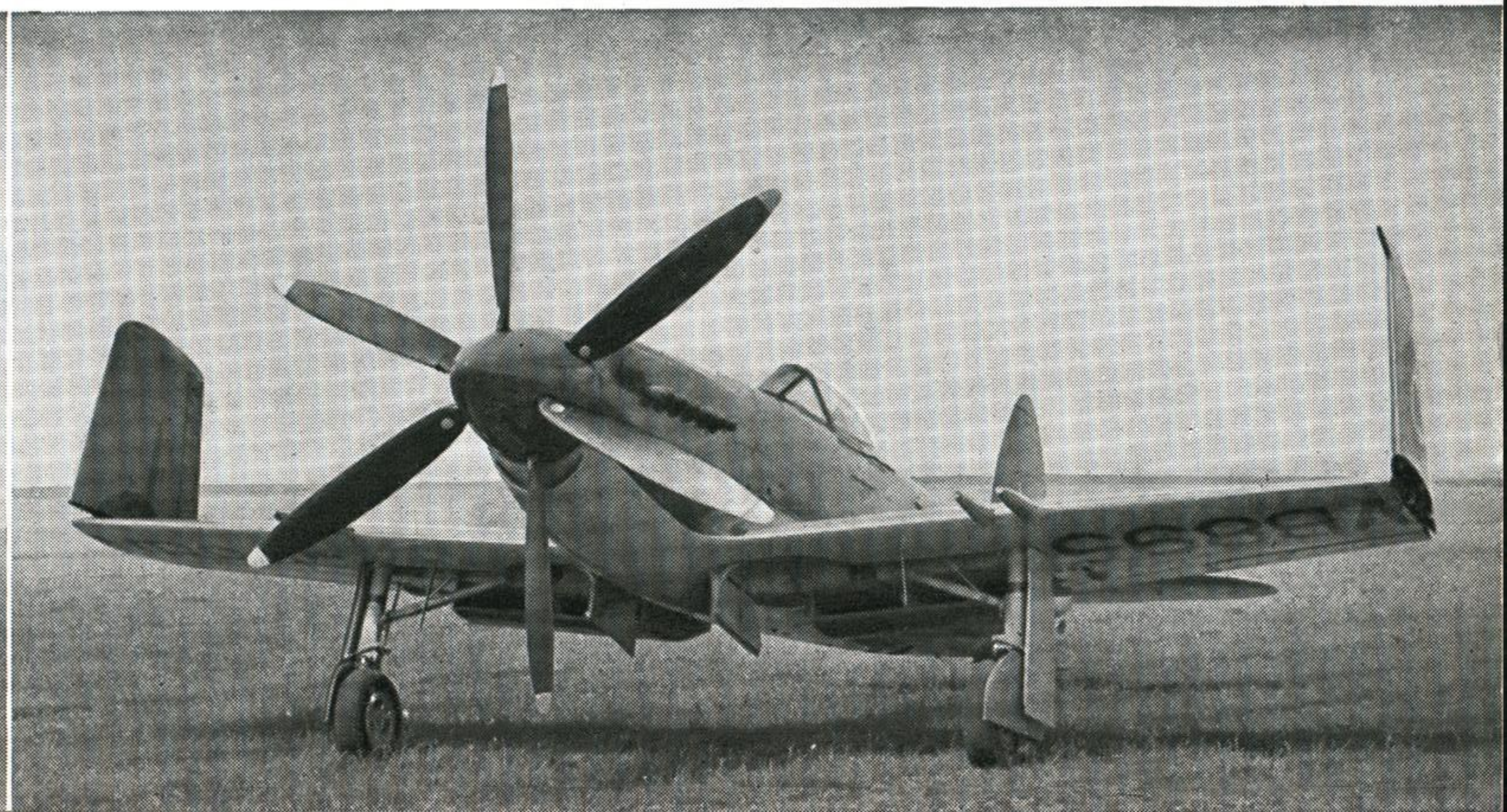
Wing tip folding only is necessary in the Seafang F.R. Mk. 32.
