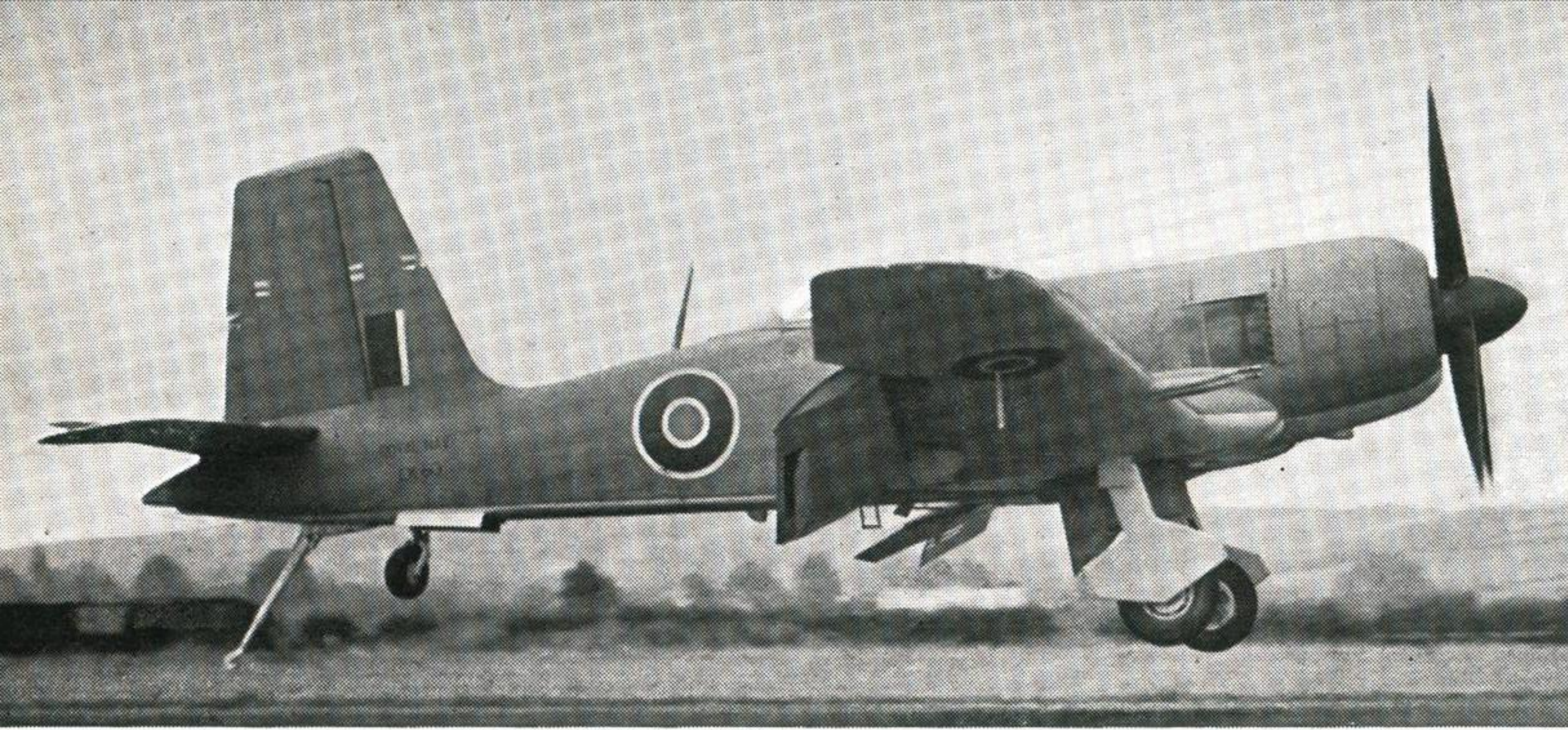
Hook out, wheels out, flaps out—The Firebrand IV about to touch down.
