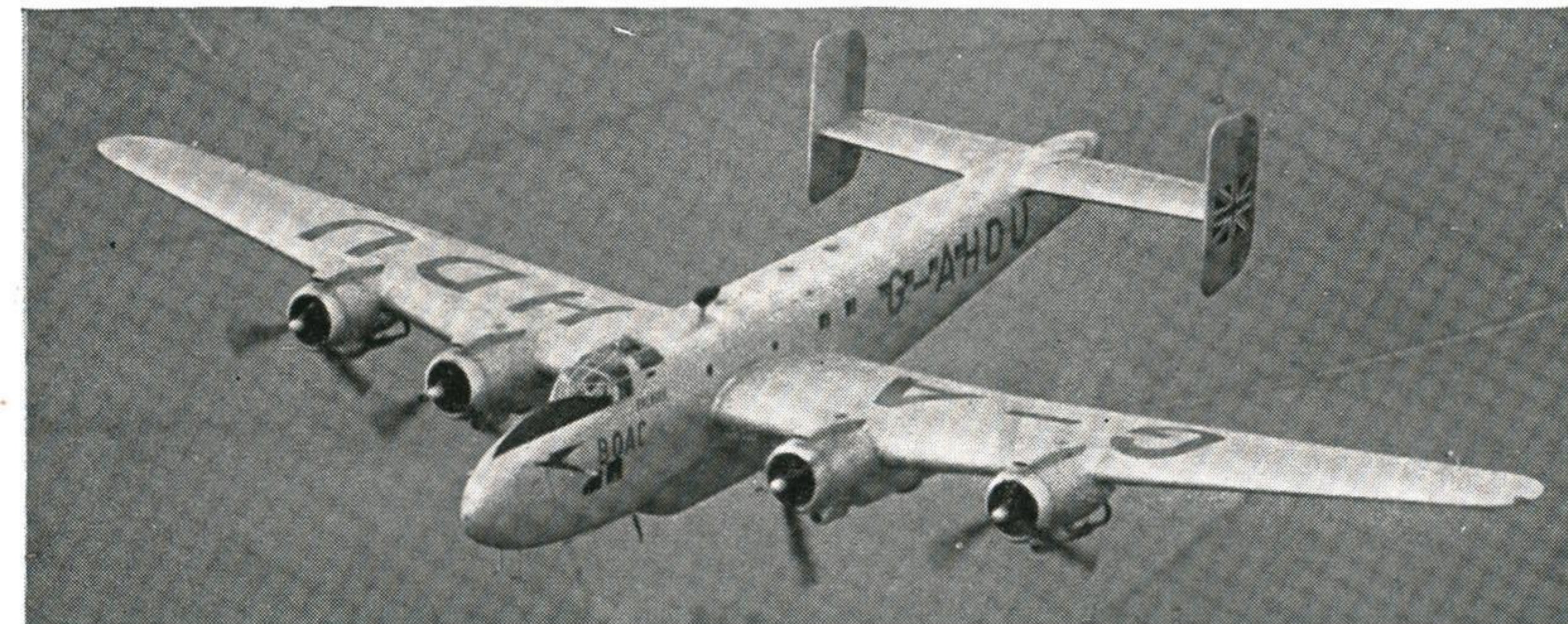
HANDLEY PAGE HALTON —Here is the first of twelve for B.O.A.C., named the "Falkirk." Although the turrets have gone and the finish and markings are civilian, the Halifax appearance is still there.
