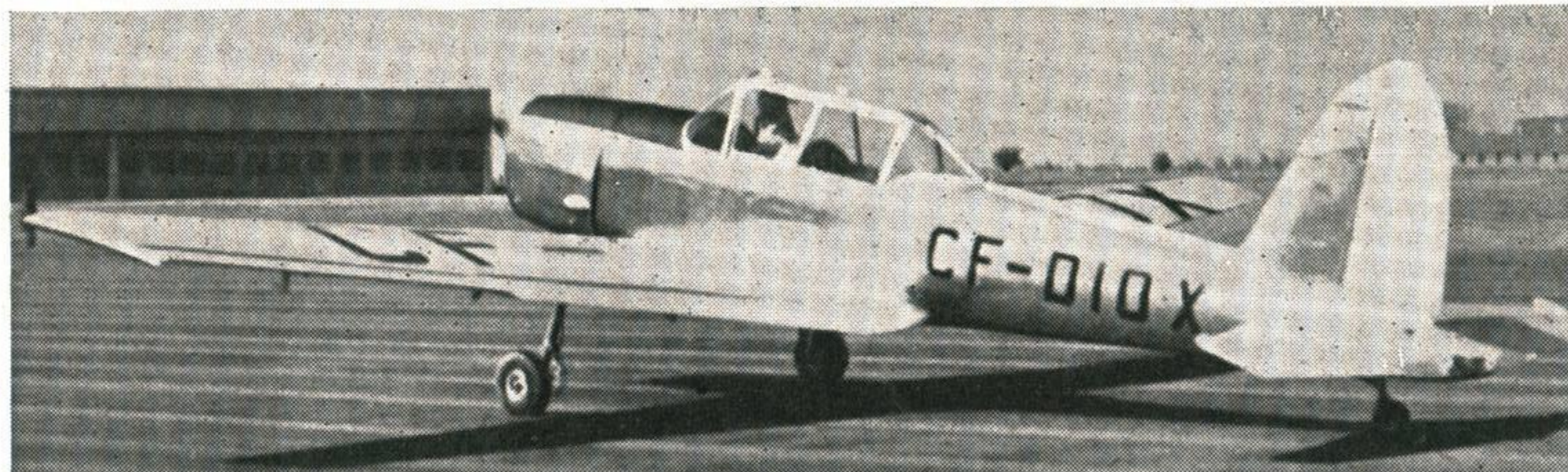
Tiger Moth Successor? —The Canadian built D.H.C.-1 Chipmunk is a fully aerobatic, low wing, single Gipsy motor monoplane. Two cockpits in tandem are totally enclosed beneath a high hood. D.H. design is evident in the tail unit.
