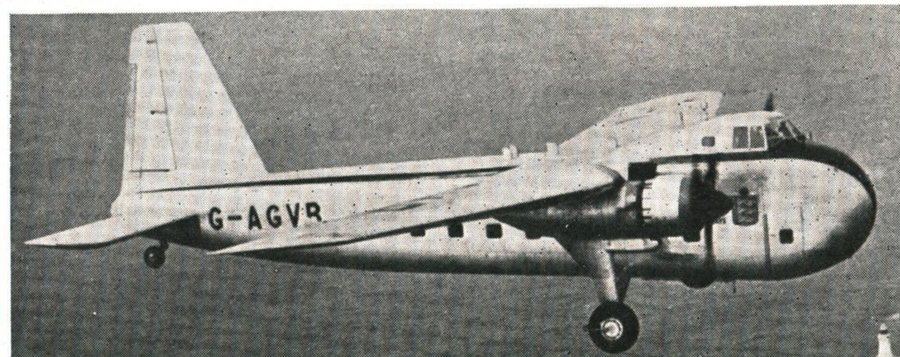
Bristol Wayfarer —This bulky transport, belonging to Channel Island Airways, is seen here on passage to the Islands. Note rectangular windows—those on the Freighter are circular. The fixed undercarriage and angular surfaces facilitate Recognition and simplify production and maintenance.
