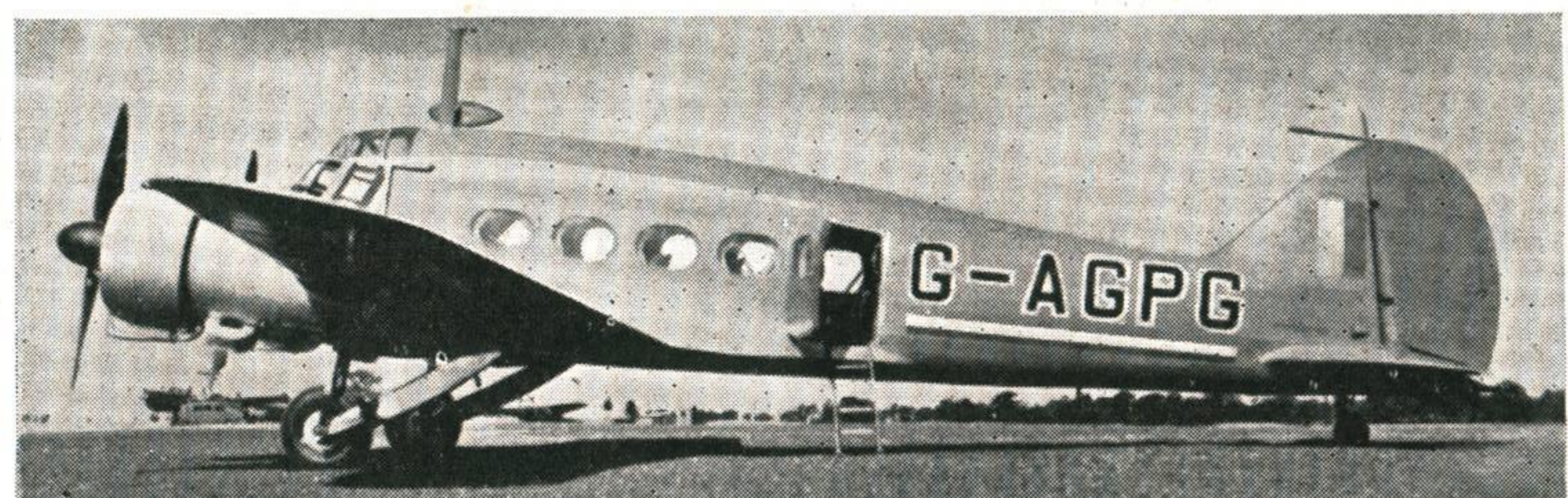
Abiding Annie —The Avro XIX is developed from the Anson. Refinements include more power, hydraulically retracting undercarriage and a deeper fuselage. Recognitionally, it is practically unaltered.
