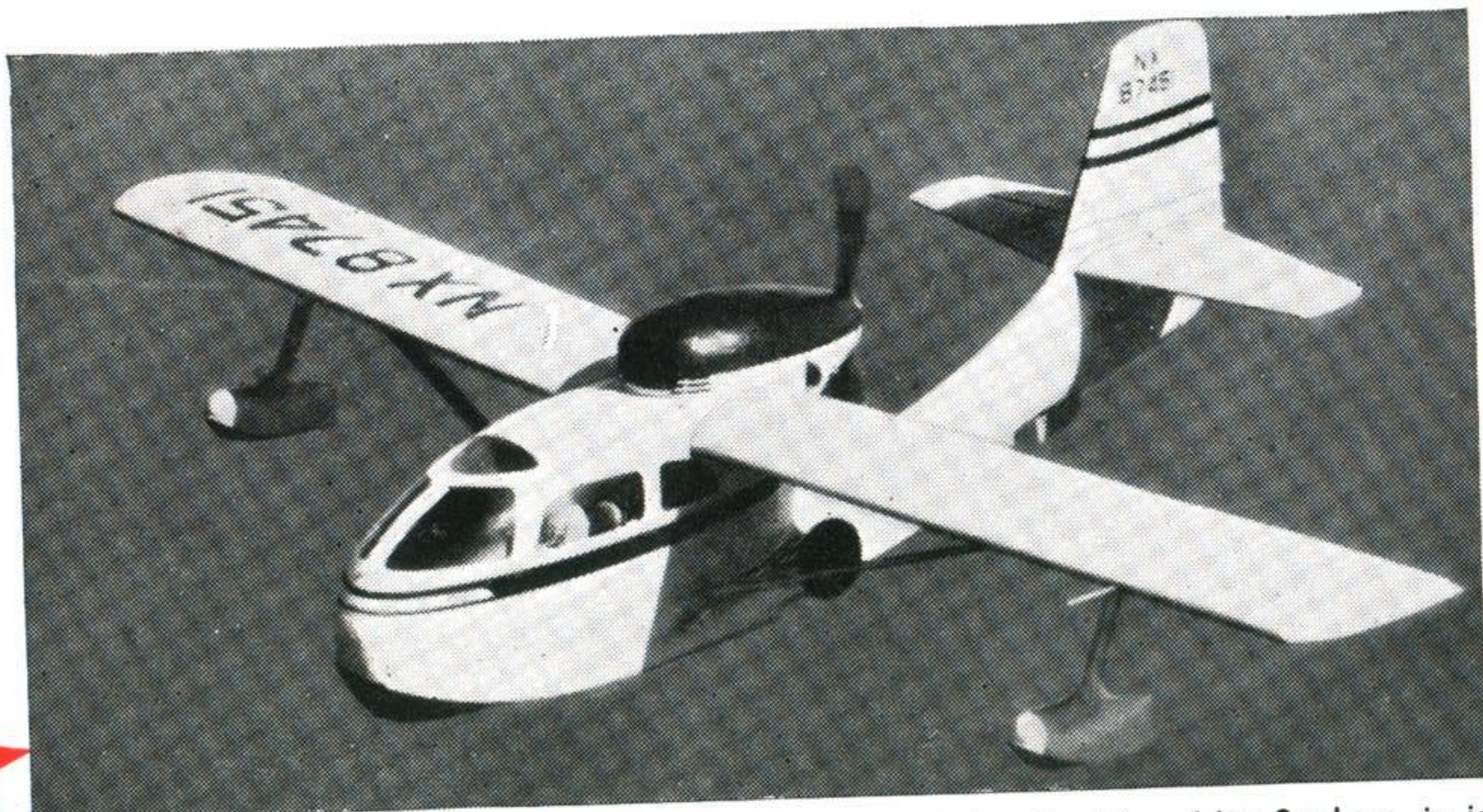
Amphibian A smart little private-owner job, the Republic Seabee is in quantity production in the factory which turned out Thunderbolts during the War. The pusher propeller seems ideal for such an aircraft.
