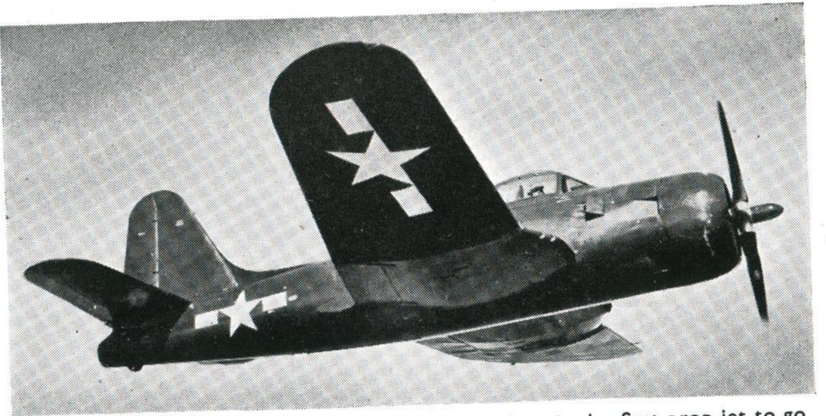
Prop-Jet The Ryan FR-1 Fireball of the U.S. Navy is the first prop-jet to go into regular service. Working together, the two forms of propulsion give it a top speed of 410 m.p.h. Normally, the jet is used only to assist take-off or in combat.
