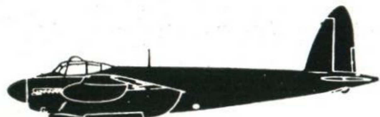
DE HAVILLAND MOSQUITO PR XVI British Photo Reconnaissance (2 Merlin) Span 54ft. 2in.
