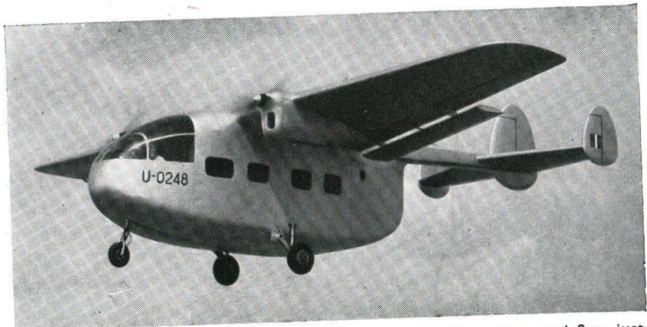
Civvy Delivery The Miles Aerovan, with its fuselage, flaps and fins, just bristles with recognition features. A ton of freight or ten passengers can be carried.
