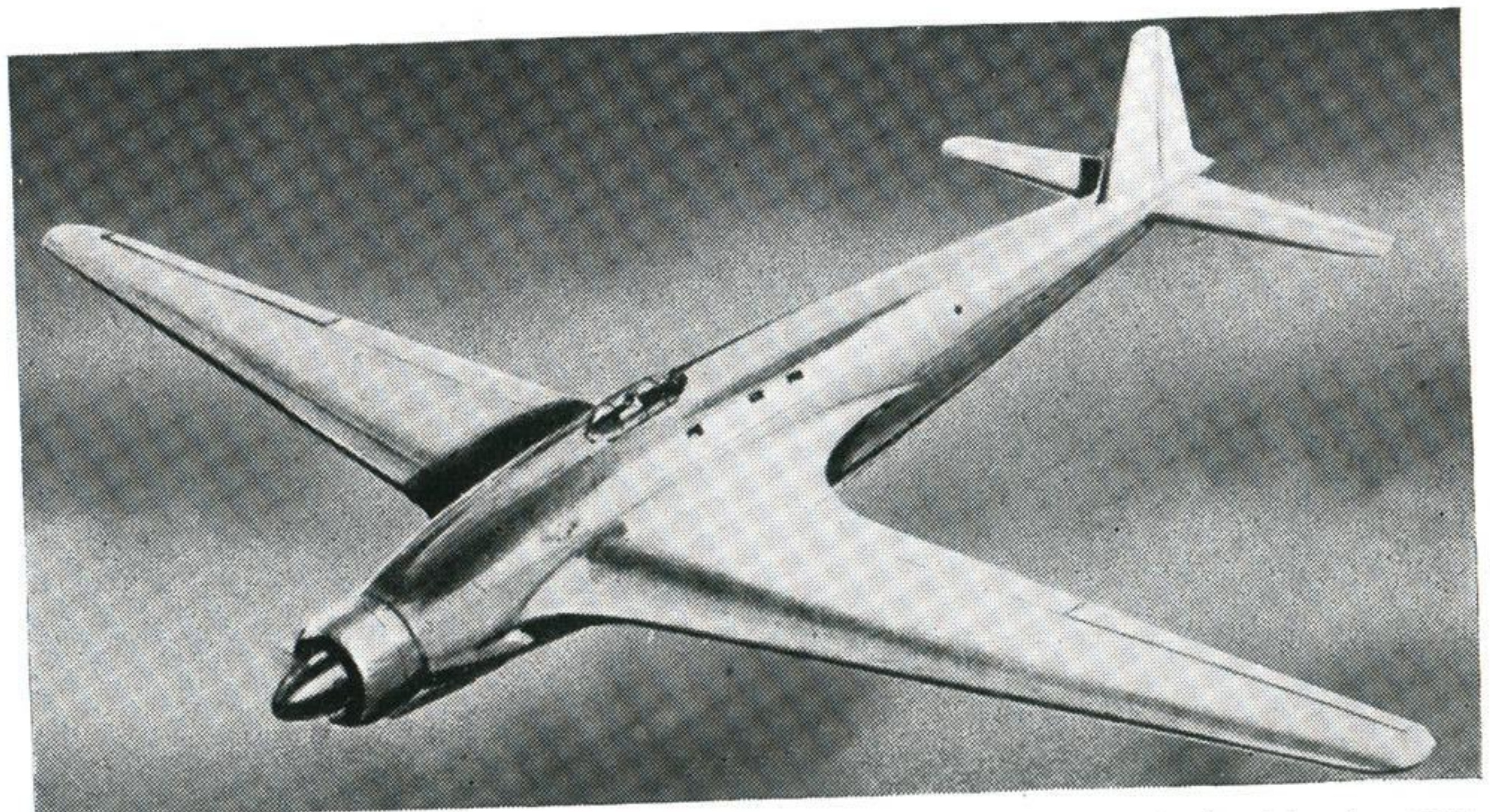
Experimental The French N.C.3021 is intended for high-altitude aerodynamic, meteorological and cosmic ray research and has a suitably pressurized cabin. The engine is a Daimler Benz DB.610 "double" motor of 2,975 h.p.
