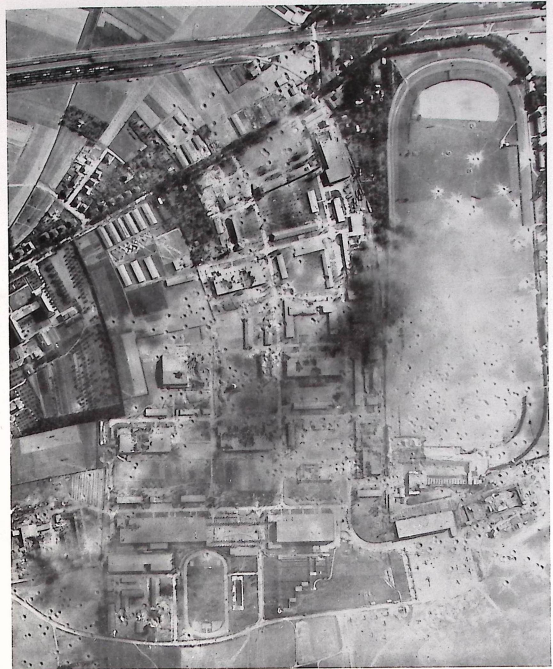
All six main workshops of the fighter assembly factory of Messerschmitt A.G. at REGENSBURG, S.E. Germany, were damaged in a U.S.B.C. daylight attack on 17.8.43. Five of these workshops were severely damaged and nearly all the craters were within the bounds of the factory. Among many other buildings destroyed or damaged were the final assembly shop, gun testing range for aircraft, workshops and offices. The bombers had fighter support part of the way and after the attack flew on to North Africa.
