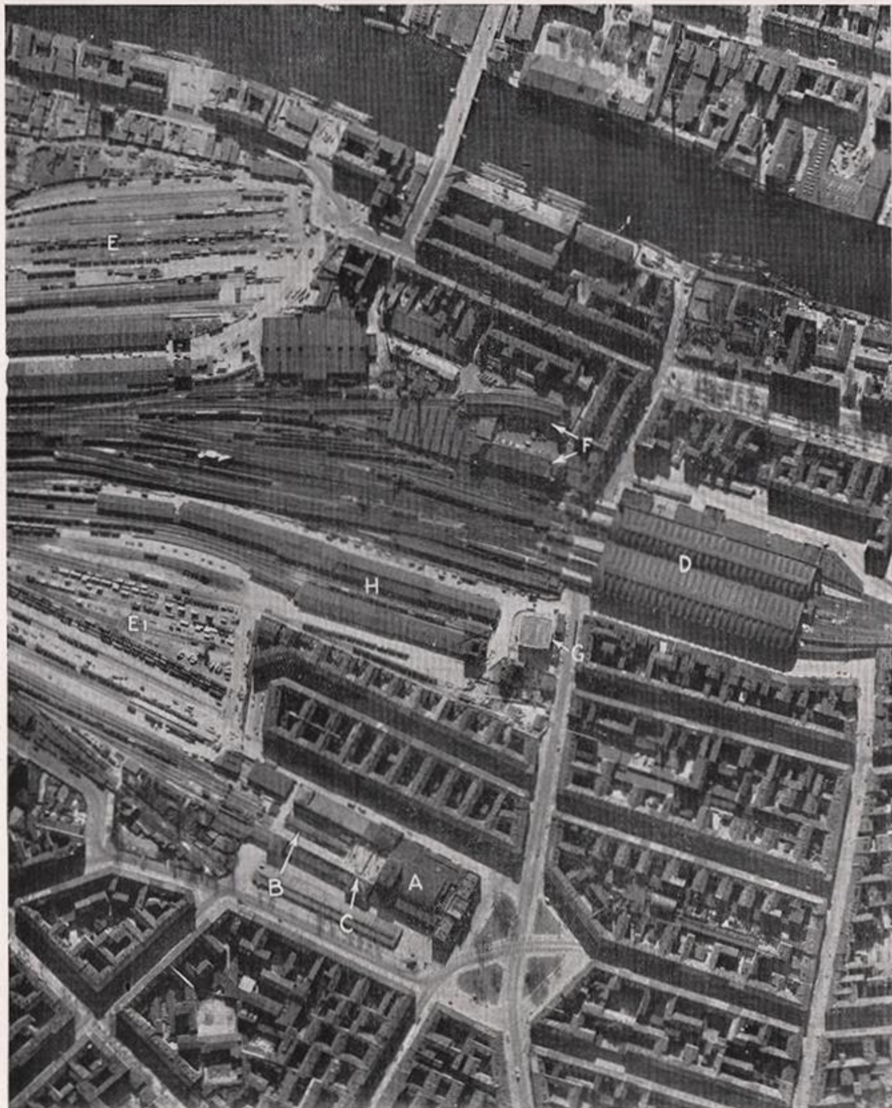
This photograph shows the important SCHLESISCHE Station (D) with its surrounding yards and buildings, which is in E. Berlin; it is an important centre for forwarding supplies to the Eastern Front. The disused Ostbahn Station (A) has had the tracks removed and stores sheds have been erected (B), while foundations for further sheds are visible at (C). The Goods Yards are at (E and E 1 ), with the Postal Dispatch Depot at (F), the Underground railway station building (G) is of a standardised design, while the Wriezener Station (H) is used for suburban traffic.
