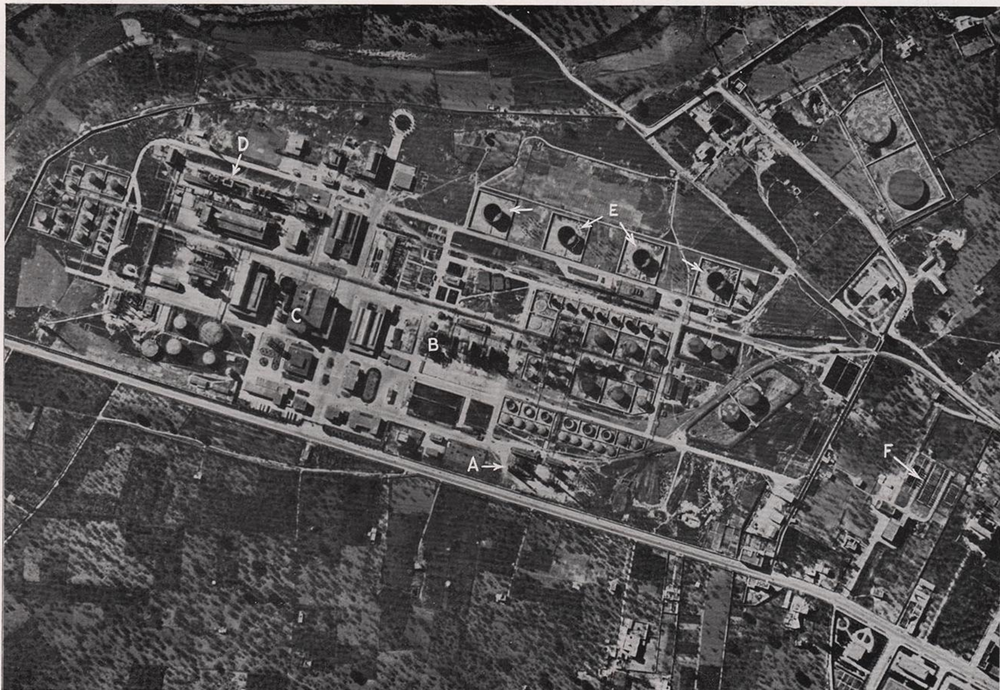
This oil refinery at BARI was designed to deal with crude oil from Albania. It remained inactive for a long period, but has come into use since the heavy damage to the Leghorn Refinery. Distillation Columns (A), Cracking Plant (B), Boiler House (C), Hydrogenation Stalls (D), Tanks with floating roofs (E), Transformer Station (F).
