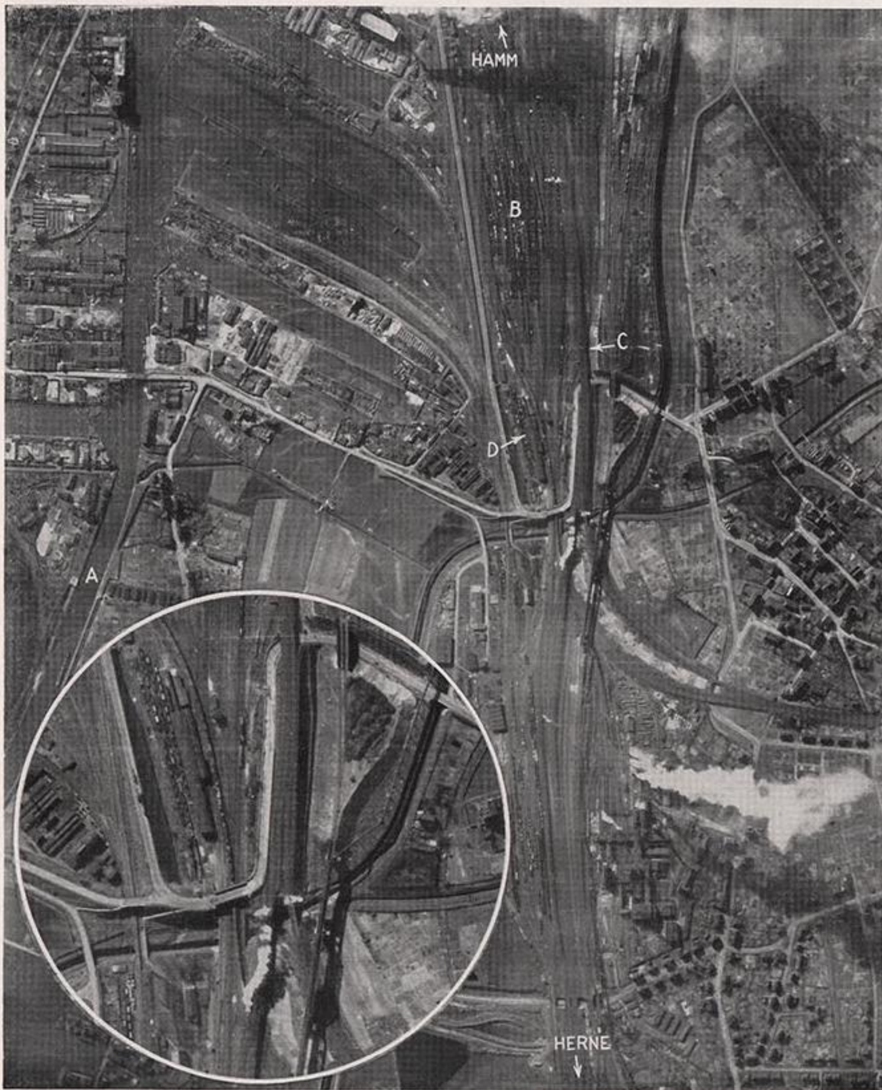
The northern end of the main marshalling yard at DORTMUND. (A) Dortmund-Ems Canal. (B) Main marshalling yard. (C) Through lines. (D) Wagon repair shops. INSET: An enlarged portion showing the road and rail nexus.
