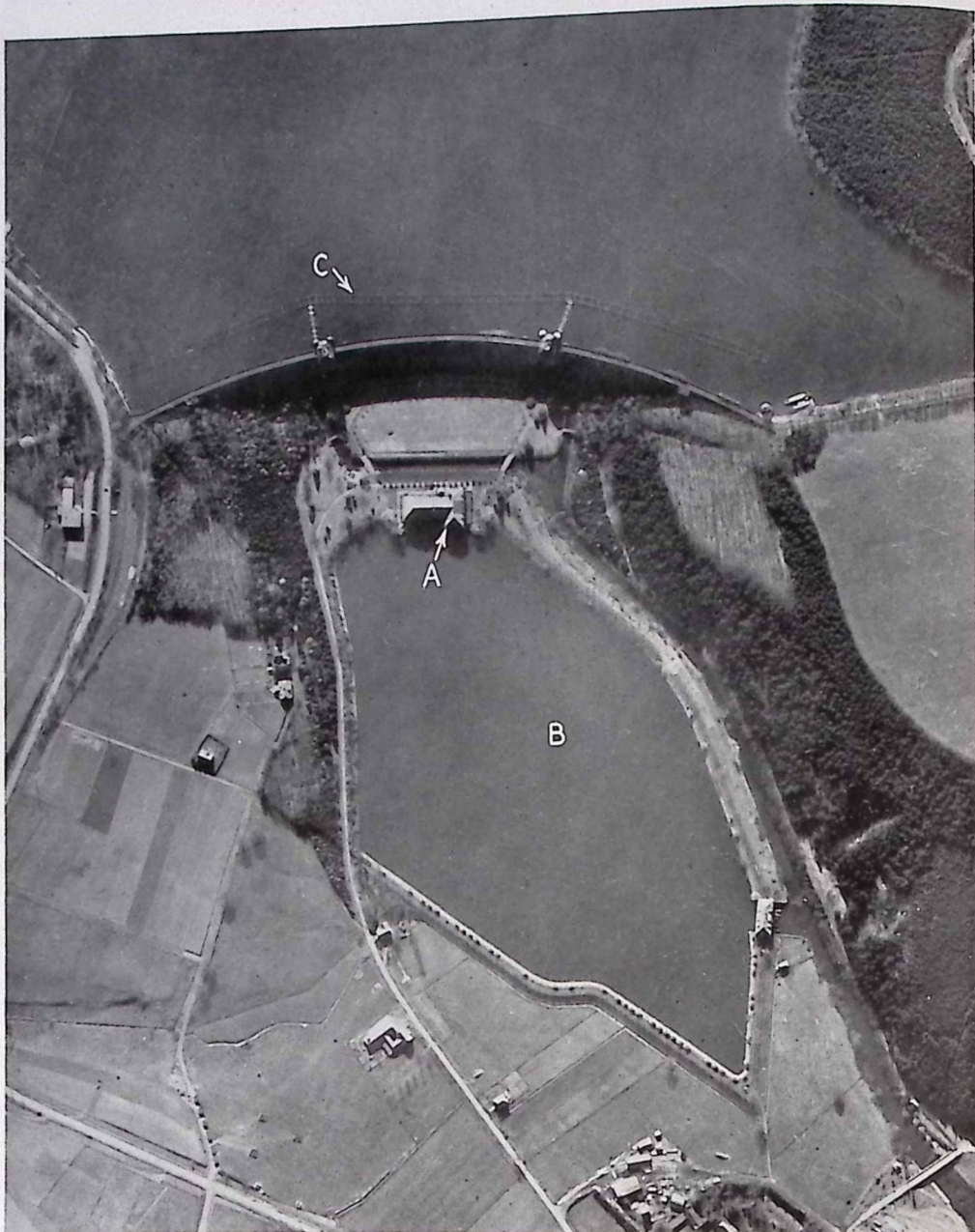
In the early hours of Monday morning, 17th. May, 1943, Lancaster bombers of the Royal Air Force breached the great Moehne and Eder Dams and damaged the Sorpe Dam, vital links in Germany's war production in the RUHR. This photograph, taken before the attack, shows part of the Moehne Lake, the Dam, the main Power Station (A) and Compensating Basin (B). Note the torpedo boom (C) covering the Dam.
