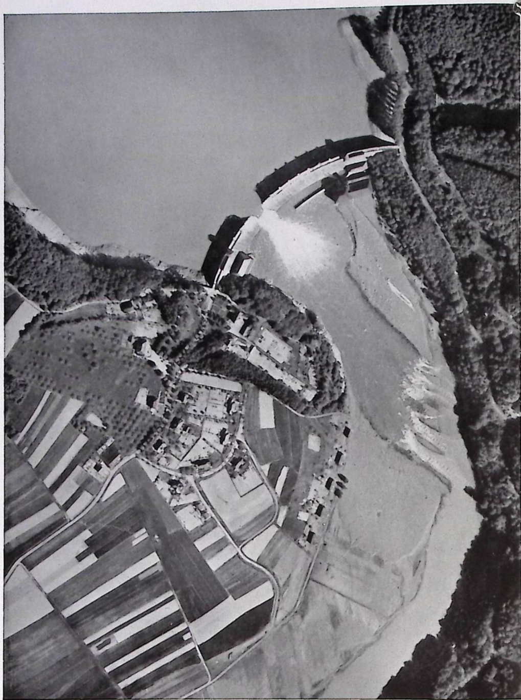
An enlargement of the damaged Eder Dam. The level of Eder Lake had dropped about 75 ft. by the time this photograph was taken (18.5.43). This would represent a loss of seven-eighths of the maximum capacity of the Lake.
