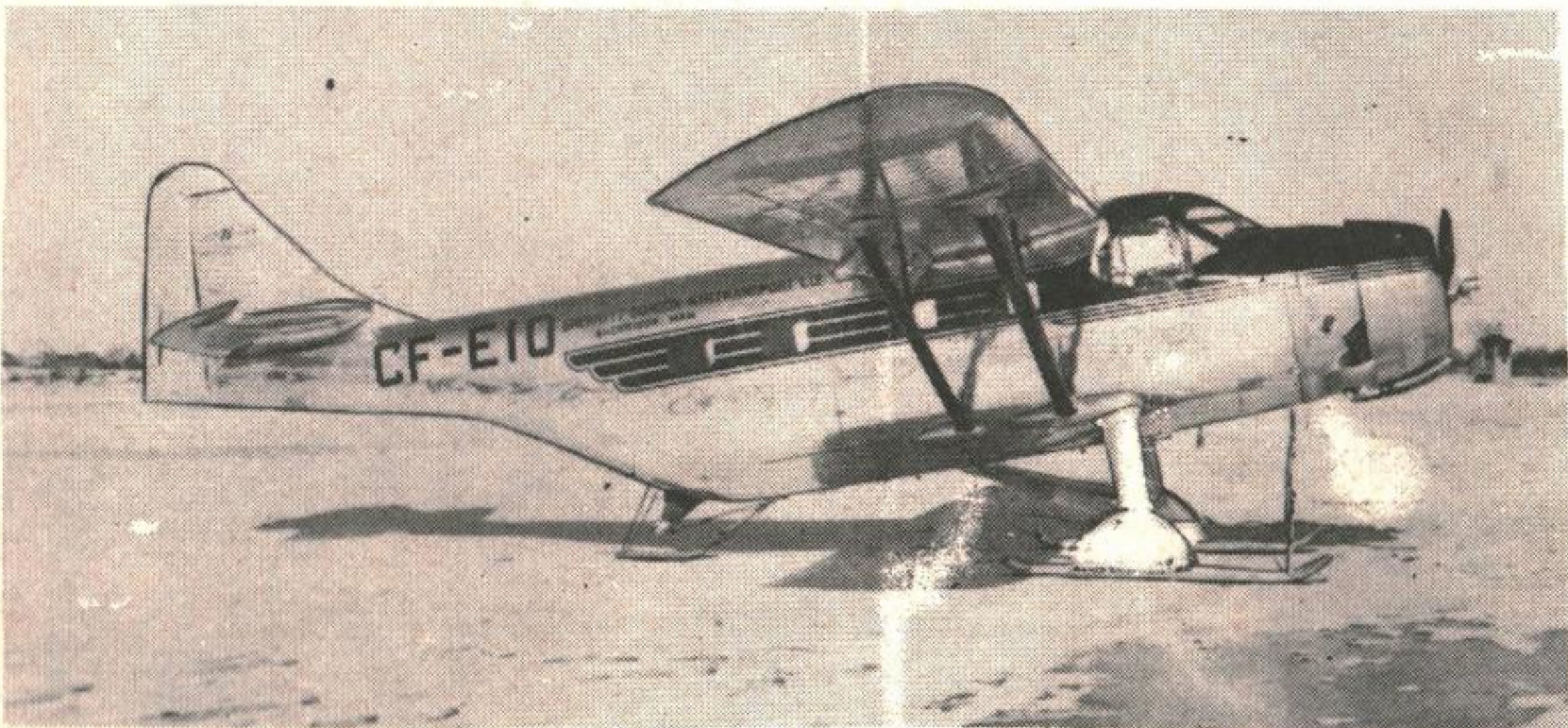
The venerable Husky aircraft used in Canada's Northland for Bush flying operation CF E 10 was owned and operated by Boreal Airways in St. Felicien, Quebec. The motto of this now-defunct outfit was "At Home in the North". With a payload on skis of 1650 pounds, this plane would fly at a lighting speed of 115 miles per hour. Top ceiling: 10,250 feet. Time to climb to a high of 5,000 feet - 10 and 1/2 minutes. Jet Jocks, eat your hearts out!!!
