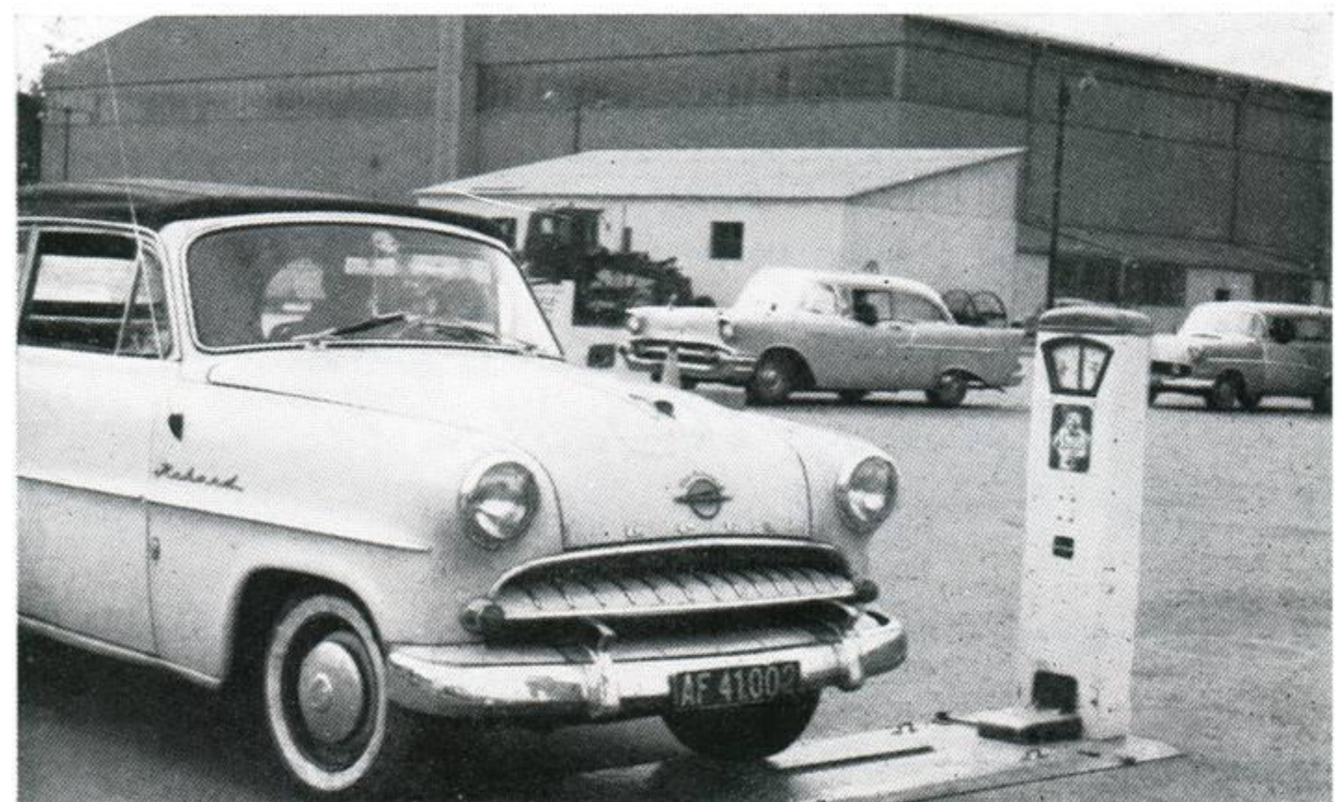
Alignment machine which checks the toe-in or toe-out of the front wheels.
