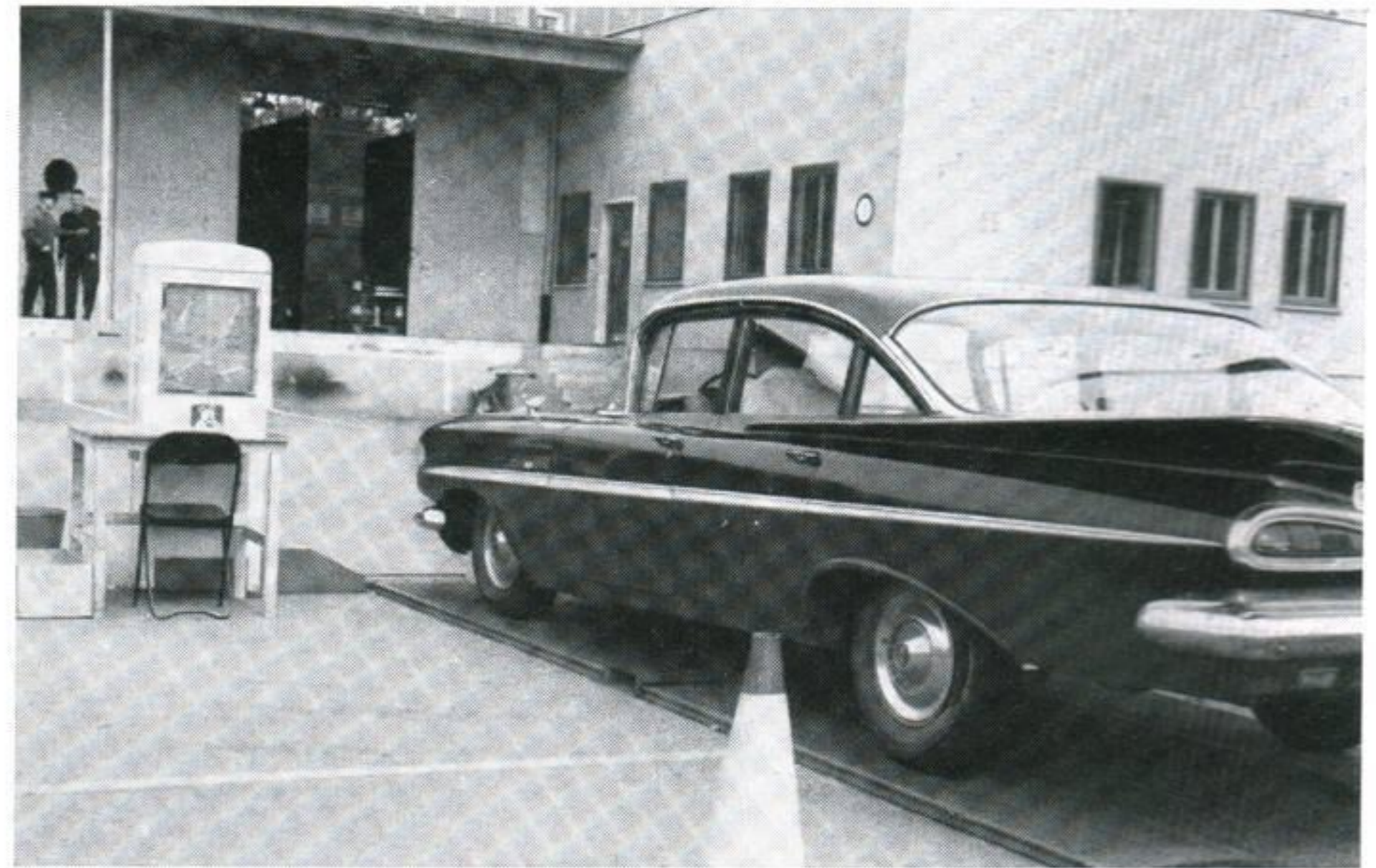
This photograph shows how the brake testing machine measures the braking power of each wheel.
