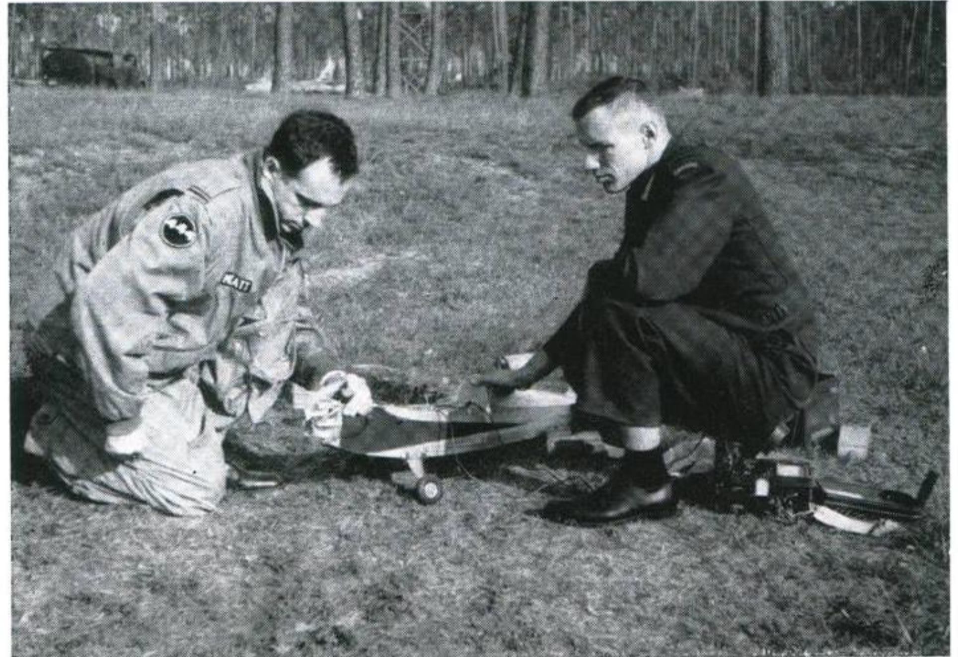
LtoR. F/O's Moffatt and Haip test running the model to check the radio controlled fuel control solenoid.
