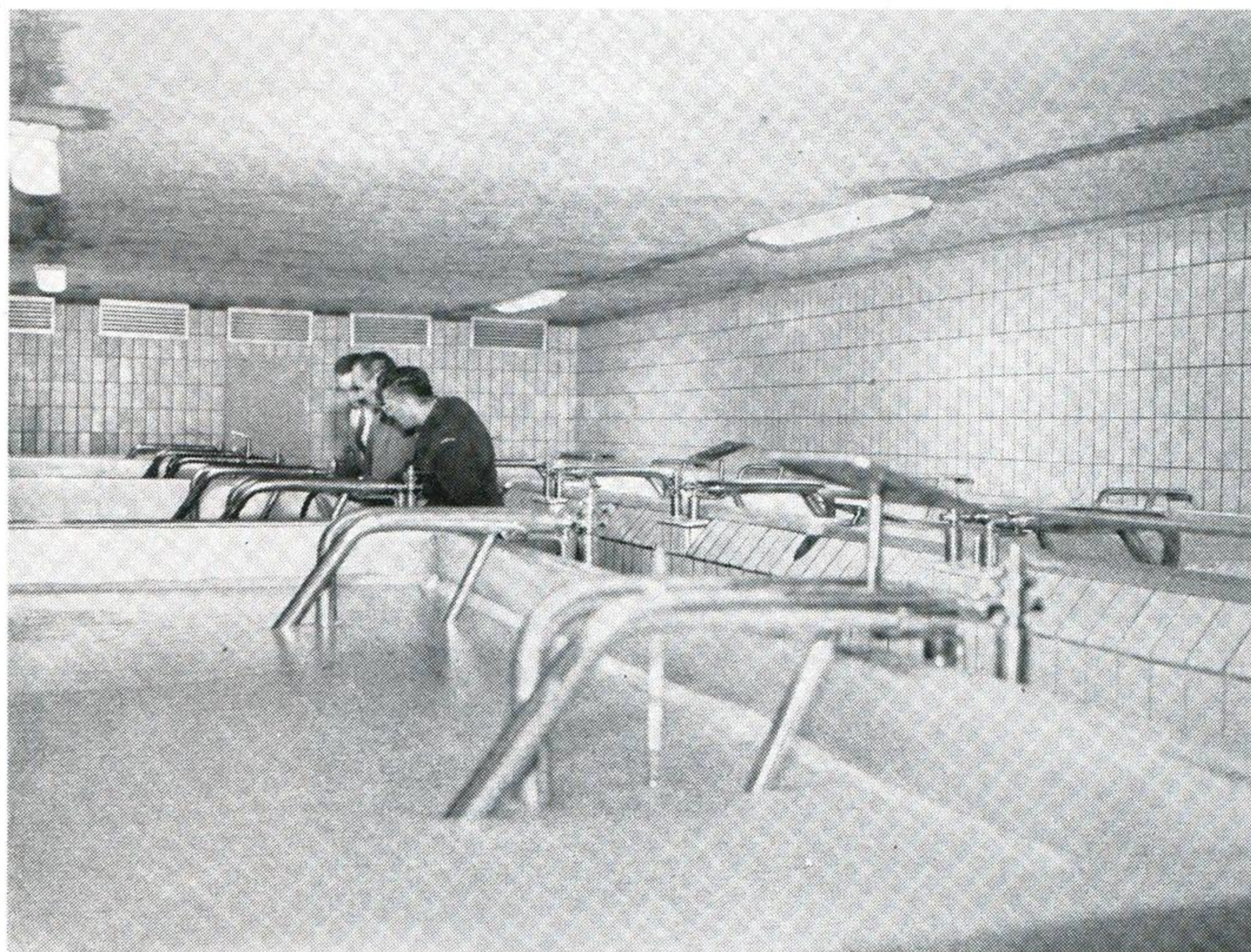
Here in the chrome and aluminium vats yeast is introduced to start the fermentation reaction. A heavy blanket of foam covers the entire surface.
