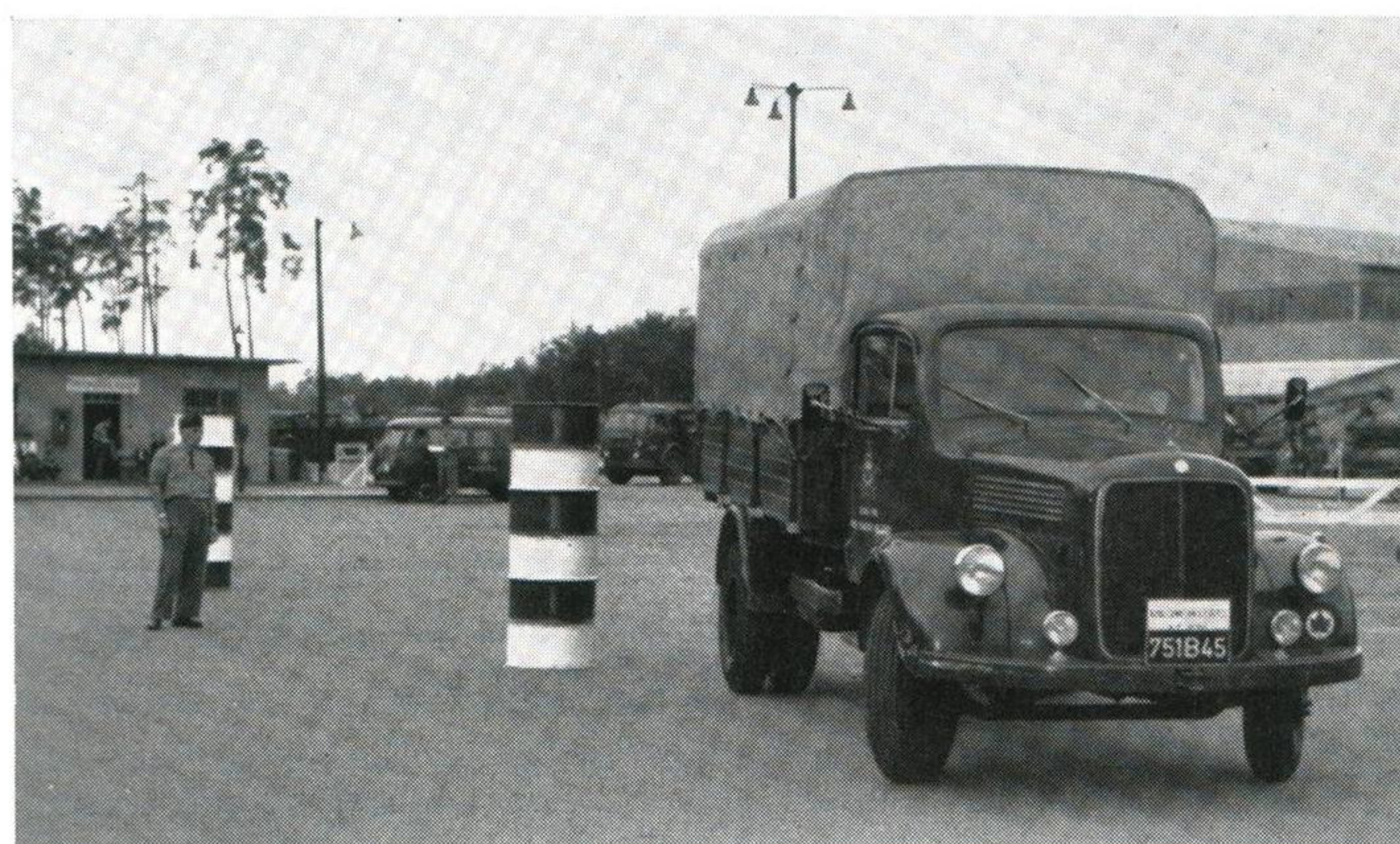
View of the Serpentine test consisting of three sets of drums through which the vehicle must pass forwards and backwards.
