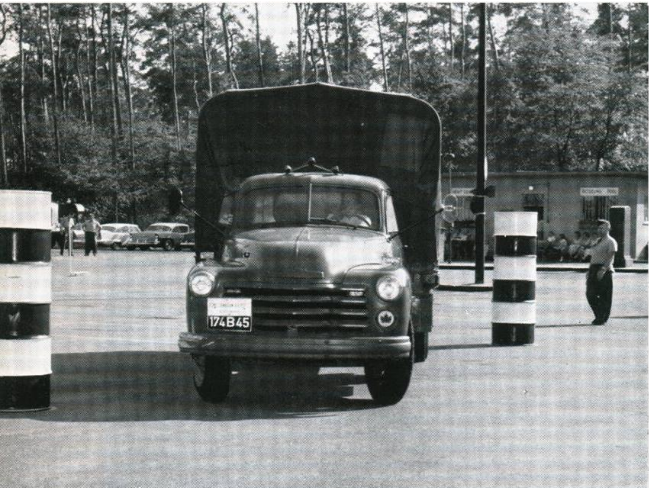
Above is the view of the Serpentine test consisting of three sets of drums through which the vehicle must pass forward and backward.
