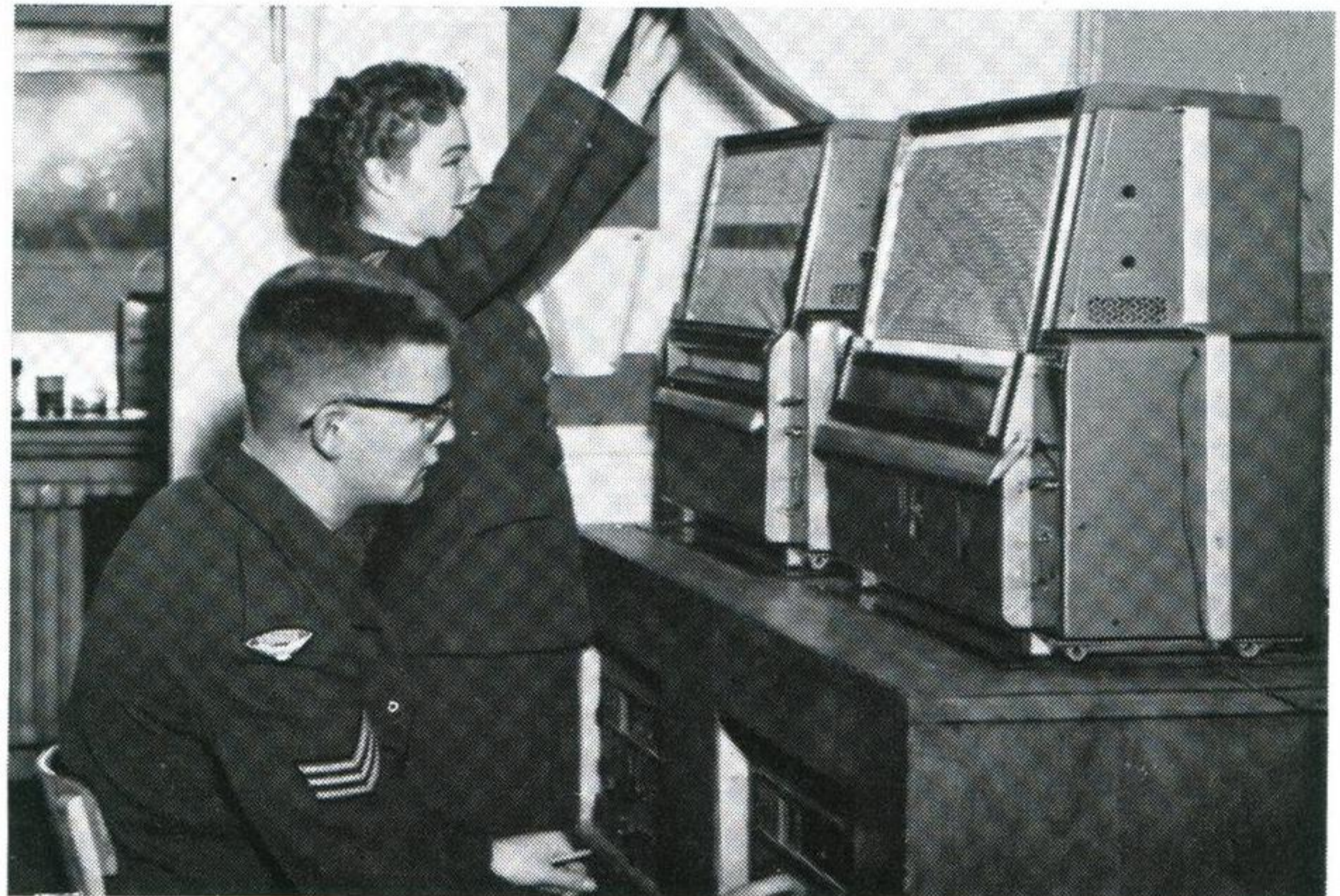
Sgt McLeod is seen tuning in a radio facsimile broadcast, while LAW Gow clears a facsimile chart from the recorder.
