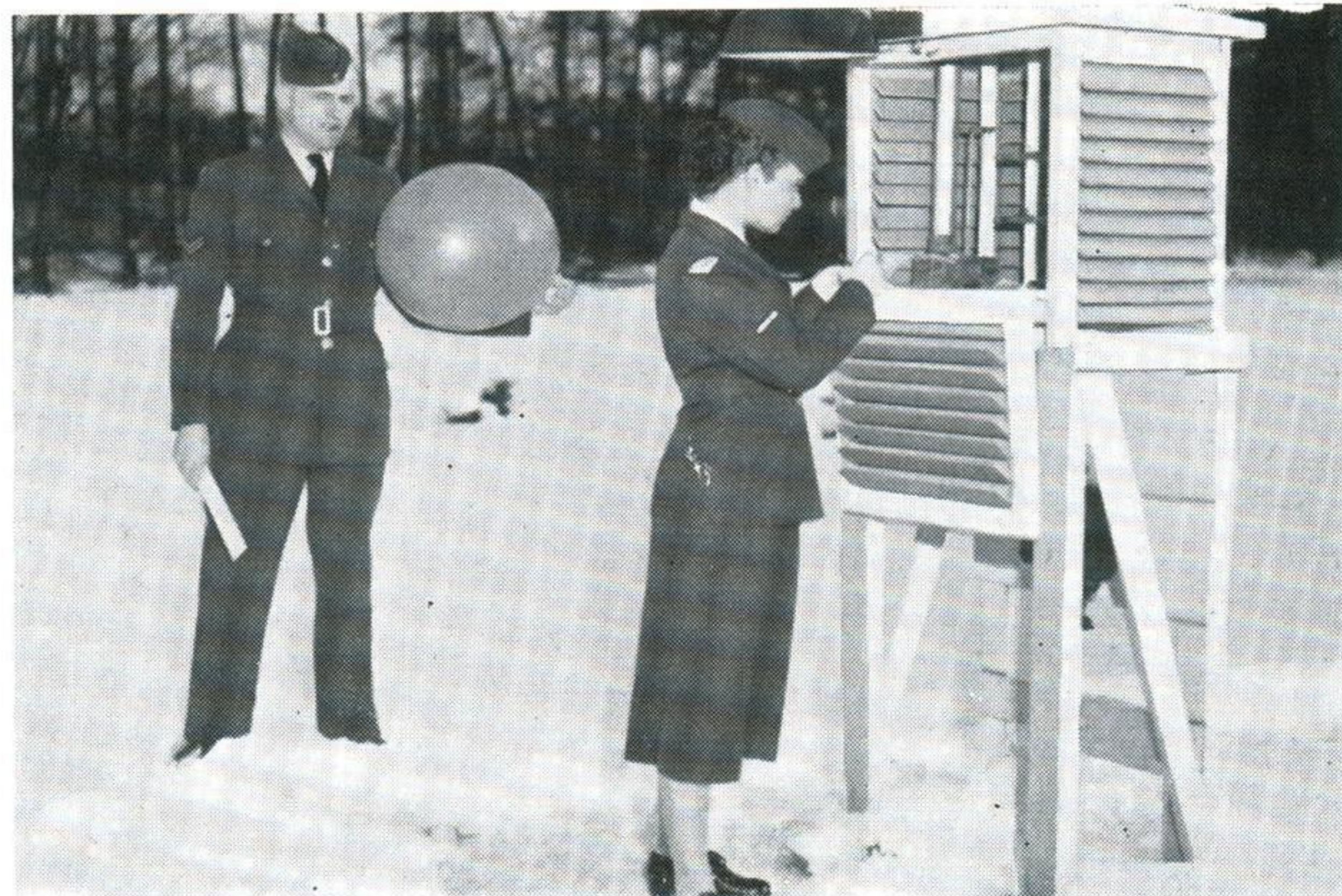
LAW Gow is recording temperature readings while Cpl Vannduyvoenvoorde is ready to release a balloon for measuring the height of the cloud base. The ruler in his hand is used for measuring depth of snowfall (Last January — you unbelievers).
