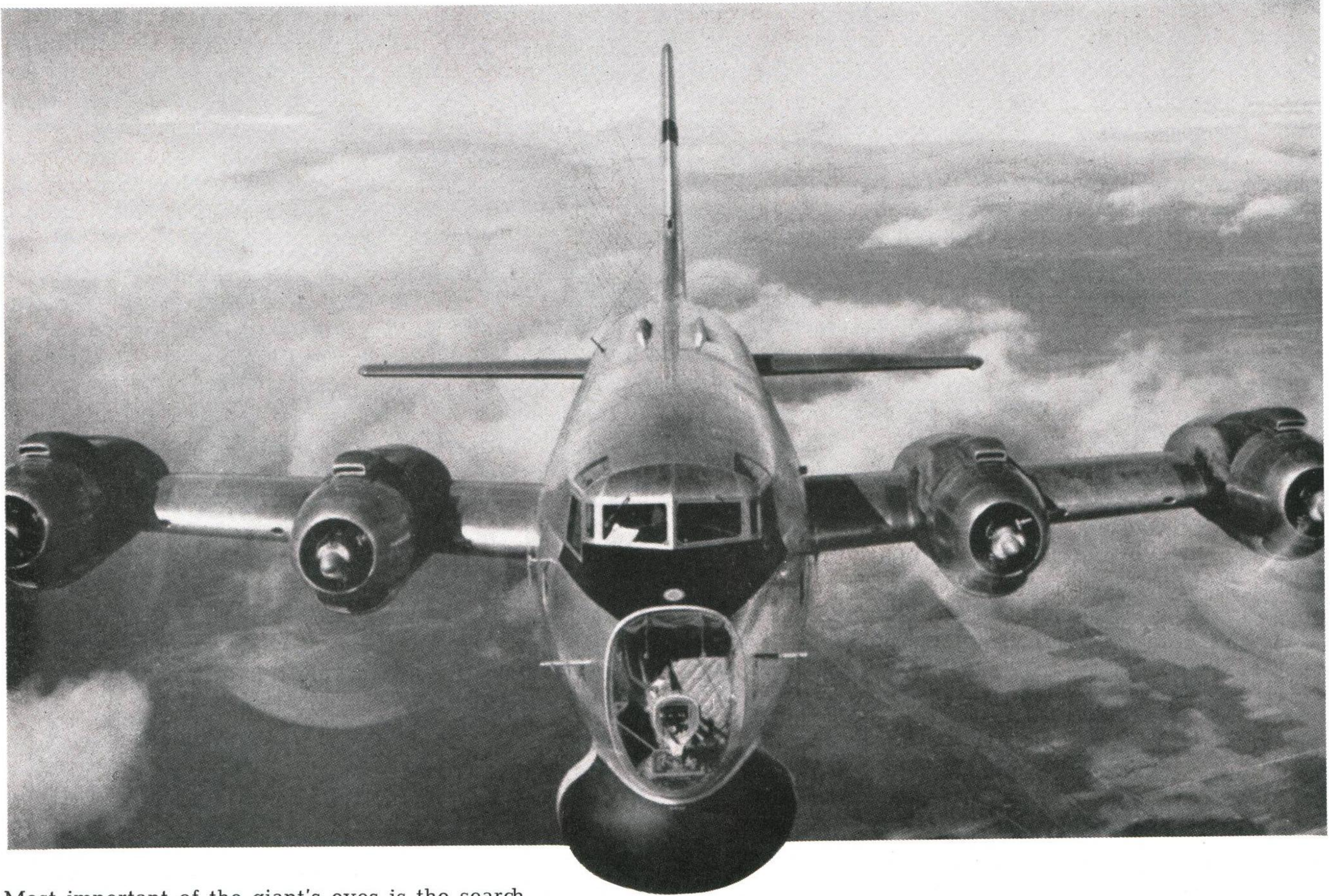
Most important of the giant's eyes is the search radar located in the radome beneath the bomb aimer's position
