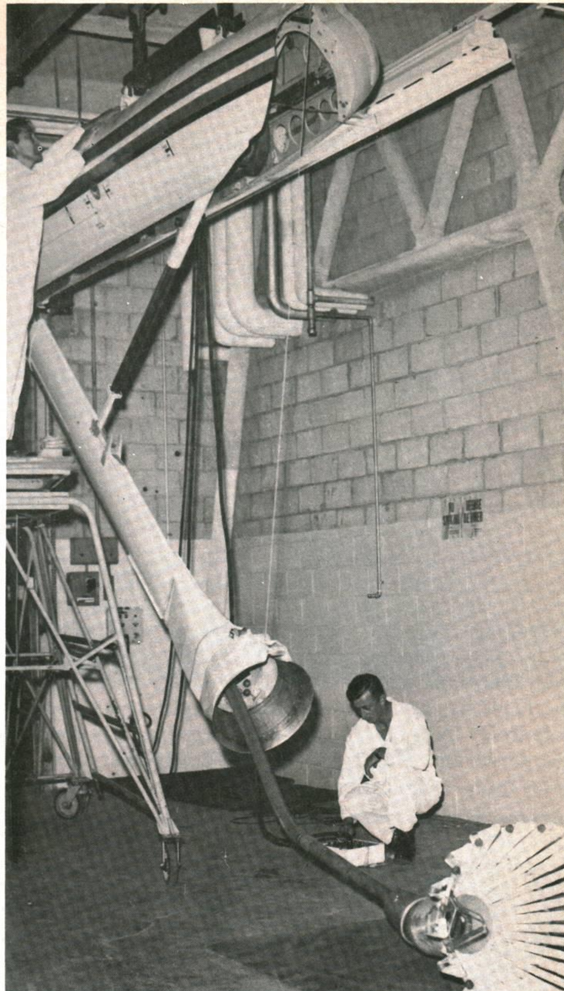
Air-to-air refuelling brings new problems for ATC technicians, seen here with a 707 refuelling boom.
