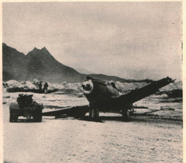
Another P-40, similarly destroyed on ground, limps on one wing-tip, its landing-gear buckled and bent. Rope attached to tail was used to tow it from scene of attack. The motor will be salvaged.
