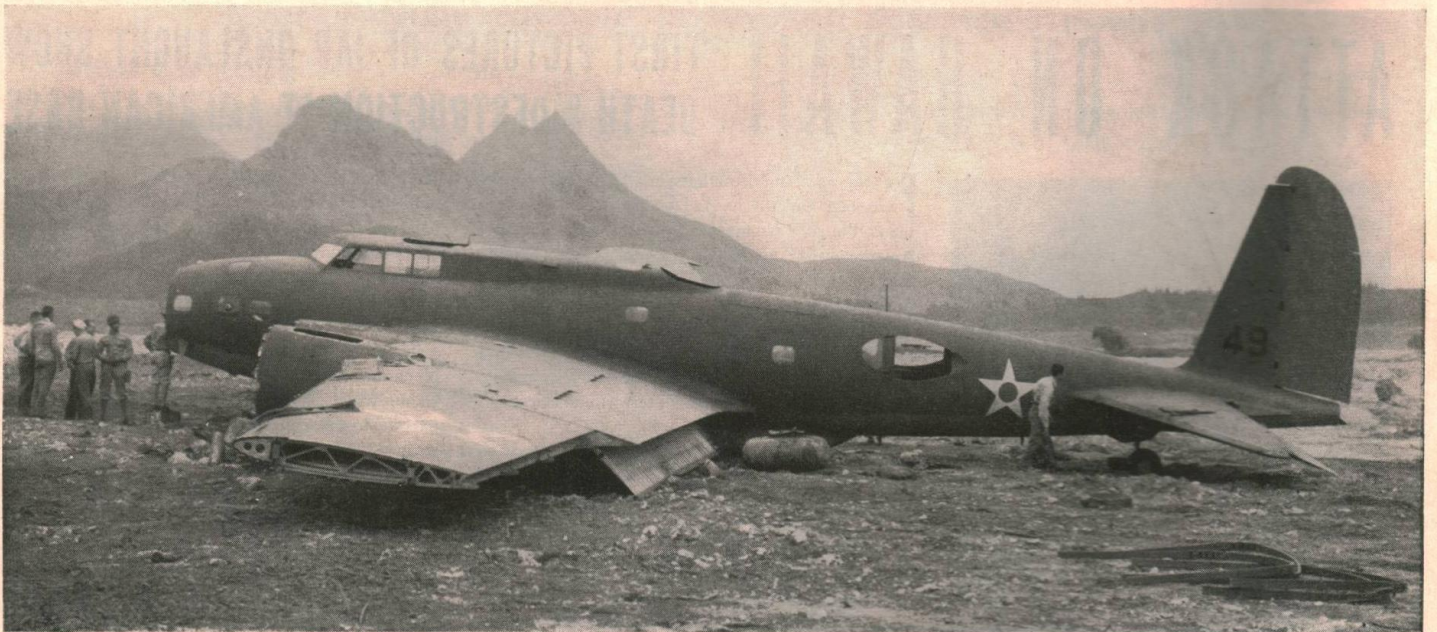
Flying Fortress , which was forced into a crash landing during the Japanese attack, is here shown being stripped by salvage crews. Engines, guns, ailerons, nose and wing tips have already been
