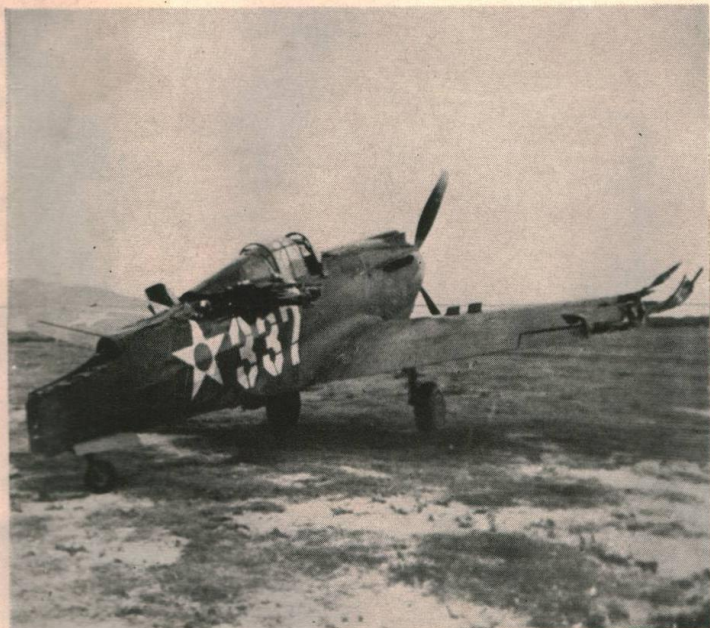
A Curtiss P-40, wrecked by Japs before it could take off, awaits scrappers. Note how right wing tip has been splintered by bomb fragments. Tail assembly and guns have been removed for salvage.
