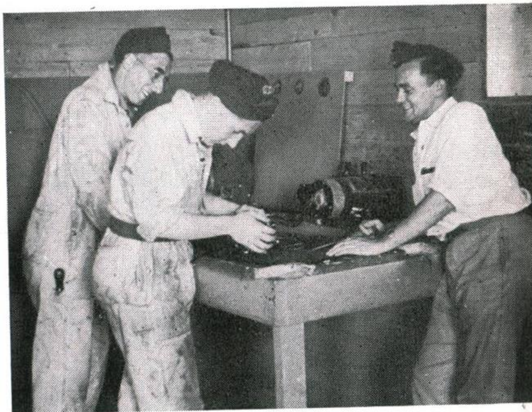
AC. Brown, LAC. Thomas and LAC. Boeth engaged in the painstaking work of adjusting generator regulators.
