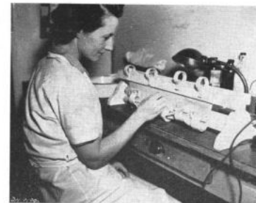
(12) Needles which were used in original blood donation here are being tested for sharpness by Mrs. George Bates, one of the staff technicians. Needle has to pierce chamois skin easily or it is discarded.
