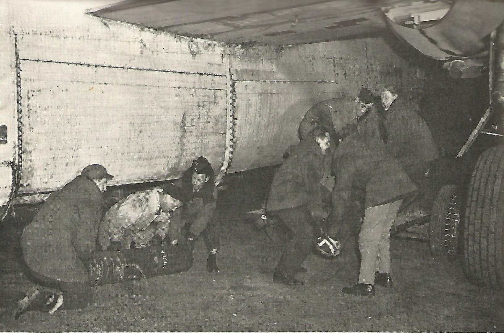
ARMOURERS LOAD and UNLOAD HEAVY DEPTH CHARGES. They are responsible for the proper functioning of the complicated release mechanism.
