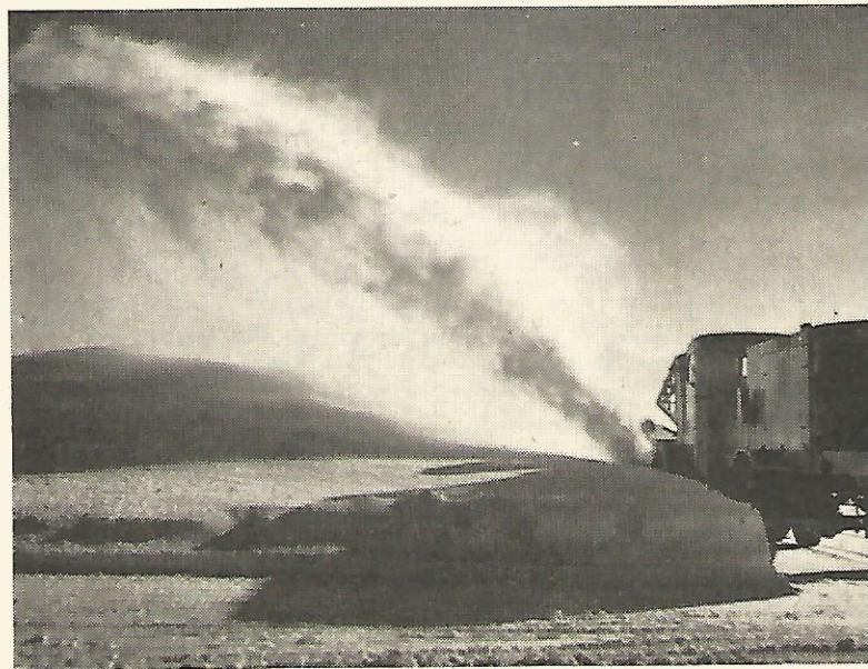
THE BLOWER can throw thirty tons a minute one hundred and twenty feet.
