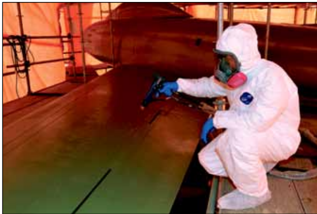
Cpl Rey Cadangan, an Aircraft Structures Technician with 402 Squadron, prepares to spray the first colour on a Canadair Sabre aircraft on display near the Garden of Memories on Air Force Way on 16 September 2014. The green colour on the aircraft is a coat of primer. Photo: Sgt Bill McLeod
