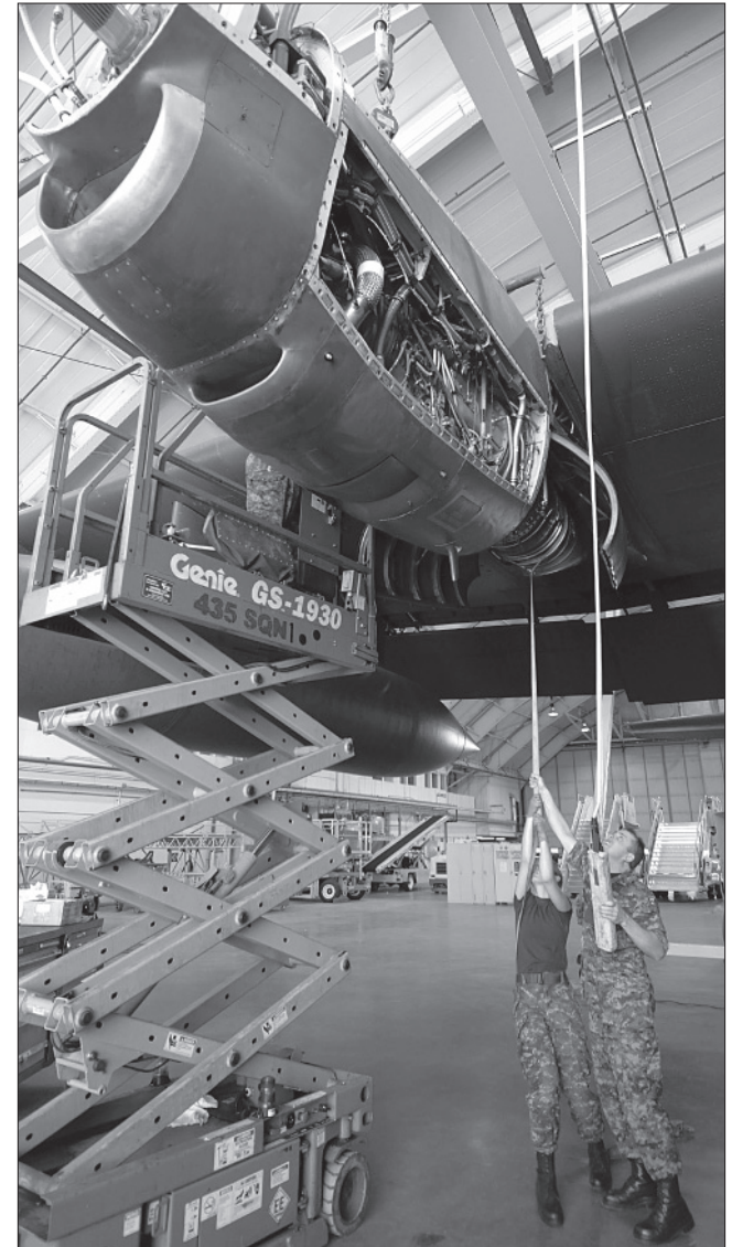
2nd Lieutenant Jessica Gaboury-Hamel and Master Corporal Mark Pic attempt to align a cc130 Hercules engine with the mounting holes during an engine change at 435 Squadron. Photo: Sgt Bill McLeod
