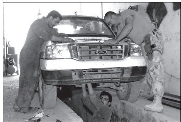
Master Cpl Richard Leray, a vehicle technician with the Kandahar Provincial Reconstruction team based at Camp Nathan Smith in Kandahar City, and two Afghan mechanics hired for the Afghan National Police vehicle Maintenance, Repair and Overhaul program work on an ANP truck, finishing up the removal of the engine for rebuilding.
