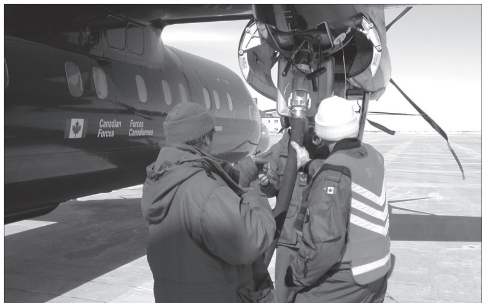
Mr. Fletcher and Cpl Morency assisting in hooking up the high pressure hose to a Dash 8 with 402 Sqn servicing.
