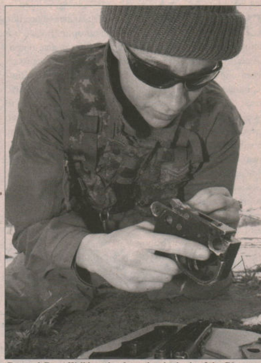
Corporal Grant Walkin strips down the pistol grip of the C6 general purpose machine-gun (GPMG) to properly align the safety mechanism.
