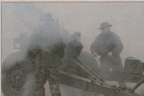
Smoke covers soldiers and the gun position after the C3 105mm Howitzer fires a blank round.
